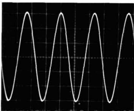
Pure sine wave at 700 Hz.
