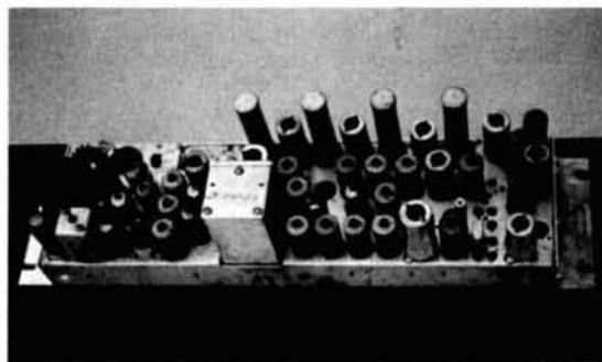
A T-44 receiver strip. Excellent for the 450-MHz primary receiver of a repeater.
