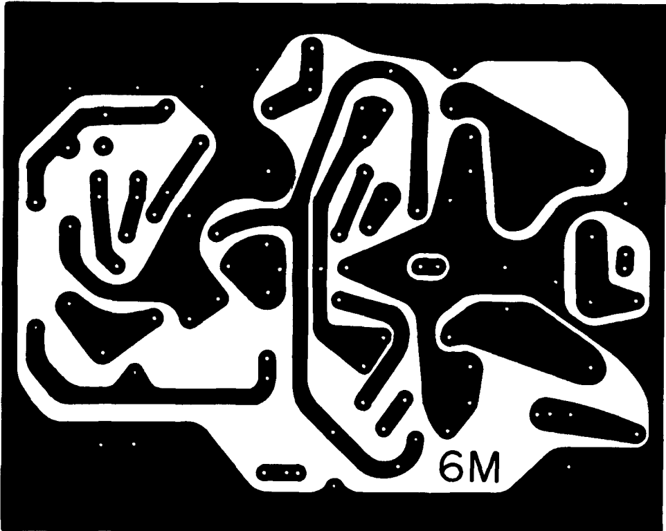
Full size printed-circuit-board layout for the six-meter converter.
