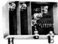
144/432 MHz Varactor Tripler, Model LVV 270. AM, FM and CW. Input up to 30 Watts. Efficiency: 50%. Input-frequency suppression: 40 dB min. .... $75.00
