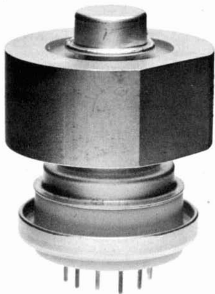
The 8873 conduction-cooled zero-bias triode.
