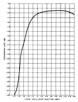
fig. 7. Measured conversion loss of the 1296-MHz double-balanced mixer circuit as a function of local-oscillator injection level.
