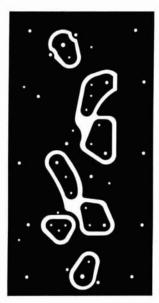
fig. 6. Full-sized printed-circuit board for the uhf preamplifier. Component layout is shown in fig. 5.
