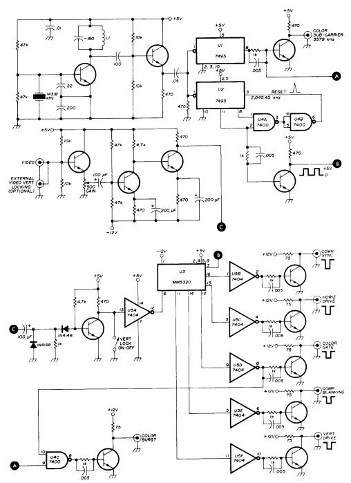
fig. 1. Schematic diagram of the television sync generator. A 16-pin socket is recommended for the National MM5320 IC (see caution in text). L1 is 25 turns no. 24, closewound on a 3/16" (5mm) diameter form.
