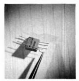
To bend the leads on the delicate double-balanced mixer package, first grasp the pins with long-nose pliers very close to the package and bend the lead downward at 90 degrees (left). Then grasp the lead at the bend and form the lead straight out from the package (center). The desired lead configuration is shown on the right.
