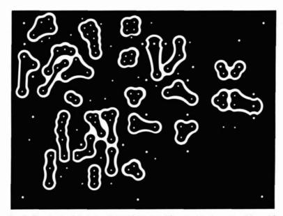
fig. 3. Full-sized printed-circuit board for the uhf converter. Component layout is shown in fig. 2.
