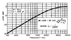
fig. 2. Response of pre-emphasis network. Changing the RC product moves the curve to the left or right but does not change its shape.
