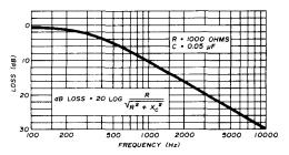
fig. 7. Frequency response of an RC de-emphasis network with R = 10k and C = 0.05  $\mu$ F.
