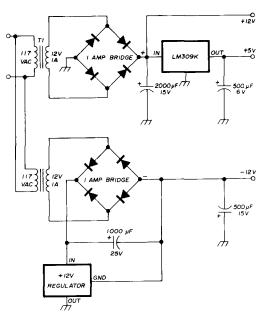
fig. 2. Power supply for the television sync generator uses voltage-regulator ICs.
