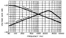
fig. 11. Frequency response of op-amp integrator and differentiator circuits shown in fig. 10.
