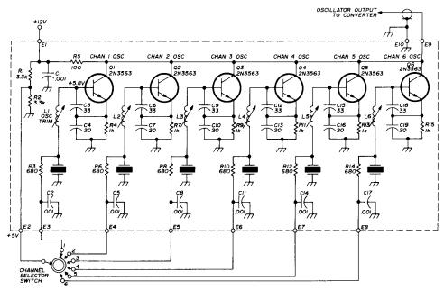
fig. 7. Schematic diagram of the six-channel oscillator for use with the uhf converter. Inductors L1-L6 consist of  $11\frac{1}{2}$  turns no. 26 (0.4mm) wire on  $\frac{1}{4}$ " (6.5mm) diameter forms with carbonyl-J slugs.
