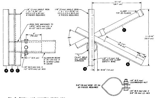
fig. 3. Spider and spreader clamp construction for the low-profile quad.
