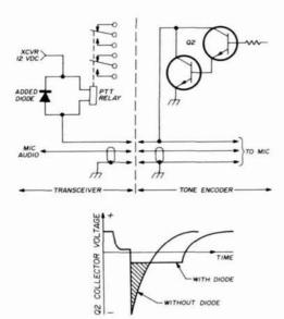
fig. 2. Correct wiring for the PTT relay in your fm transceiver, Proper waveform on the collector of transistor Q2 is shown below the schematic.
