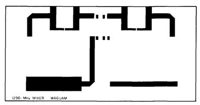
fig. 4. Full-size printed circuit board for the 1296-MHz double-balanced mixer. Material is 1/16" (1.5mm) G-10 fiberglass-epoxy board, double clad with 1 ounce copper.
