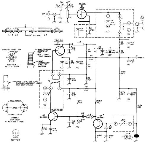
fig. 1. Schematic diagram of the unit converter, Components marked with an asterisk are not required if the multi-channel oscillator (fig. 7) is used. Inductor LS is 11-2/3 turns no. 22 (0.6mm) on 14" (6.5mm) diameter, slug-tuned coil form (carbonyl-J slug). Windings of other inductors depend upon operating frequency and are described in the text. Printed-circuit layout is shown in fig. 2.
