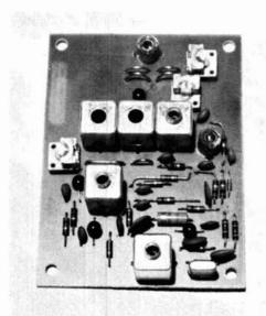
Basic uhf converter covers the range from 420 to 470 MHz. Printed-circuit layout is shown in fig. 5.
