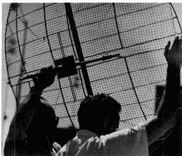
WA6KKK and WB6MGZ aim 18.6-dB 1296-MHz dish.
