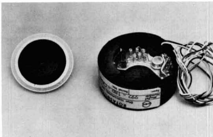
Internal construction of the optical shaft encoder. The LED light source is under the half-moon shaped shield on the left-hand side of the unit (right).
