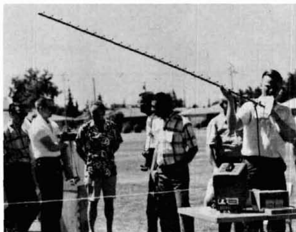
K7ICW's 30-element Yagi for 1296 MHz yielded -2.5 dB!
