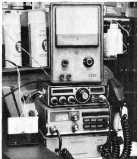
Test setup used by K2PMA to check VU meter readings with a calibrated audio power meter.
