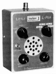
The DF is battery-powered, can be used with accessory antennas, and is 12/24V for use in vehicles or aircraft. It is available in the 140-150 MHz VHF band and/or 220-230 MHz UHF band. This DF has been successful in locating malicious interference sources, as well as hidden transmitters in "T-hunts", ELTs, and noise sources in RFI situations.
