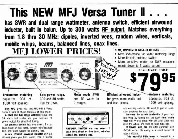
toroid for more watts out. A 1:4 balun for balanced lines. 1000 volt capacitor spacing. Mounting brackets for mo-
