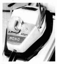
The switching arrangement is shown in this view of the dual-impedance headphones. Photo by WD9CXG.
