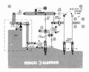
fig. 10. Parts layout, Microcomm model LO-70 uhf local oscillator (microstripline side).
