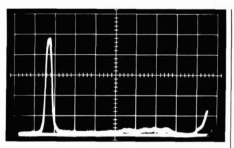
fig. 13. Swept-frequency response of the Microcomm model PB-70 filter ultimately used as a tuning aid for aligning this LO, as described in the text. Vertical and horizontal scales are as in fig. 12. Note absence of spurious responses out to 2.5 GHz, as well as the passband insertion loss of less than 1 dB.
