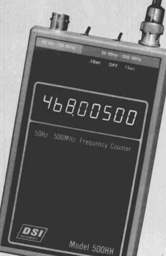
BNC Inputs 1 Meg Direct 50 Ohms Prescaled 8 Large .4" LED Readouts Auto Decimal Point & Zero Blanking
