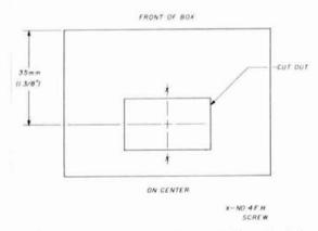
fig. 6. Location of the plug cutout on the end of the minibox. Location of the plug should be adjusted if necessary, since alignment affects appearance when the unit is plugged into the rack.
