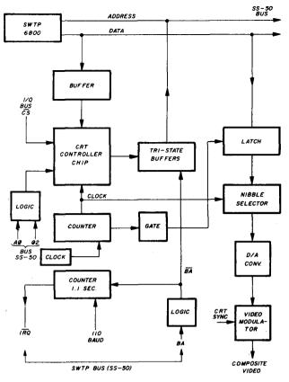
fig. 2. Block diagram of the video-interface card.
