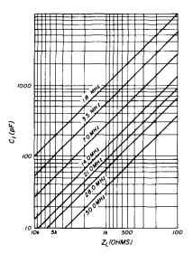
fig. 5. Plot of the tuning capacitance (C1) vs. plate load impedance (Q = 12).
