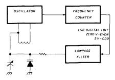
fig. 1. Basic frequency-locked-loop system.
