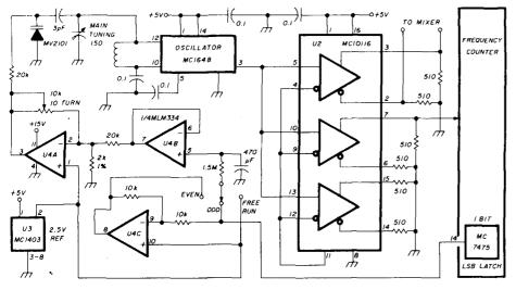
fig. 3. Frequency-locked-loop schematic.
