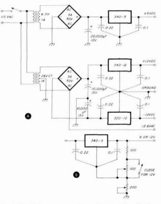
fig. 4. Circuit for power supply used in the racks, (A). The 320 regulator case must be insulated from the ground. (B) shows an alternative connection for +9, +12 volts. The negative line would be similar.
