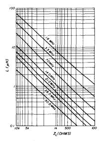
fig. 4. Plot of the plate inductance vs. plate load impedance for the high frequency Amateur bands ( $\Omega \approx 12$ ).
