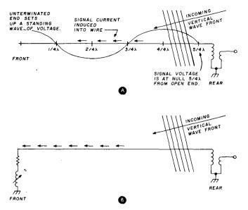
fig. 3. Diagram (A) shows the standing wave on the unterminated wire caused by an incoming signal from the rear. The signal voltage across the transformer is at a null  $5/4\lambda$  from the open end. When the wire is perfectly terminated (B), the signals from the rear of the antenna are absorbed by the termination.
