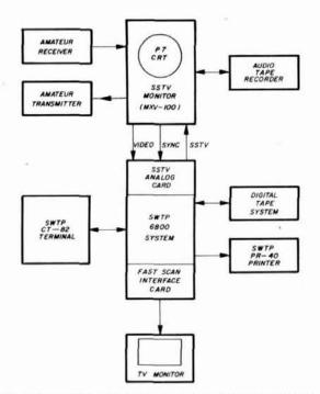
fig. 1. Block diagram of the computer and SSTV systems.
