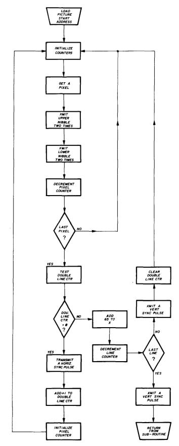
fig. 14. Flow chart of the zoom routing on the SSTV picture (TRZ).
