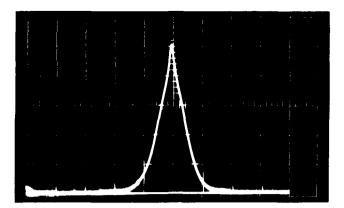
fig. 4. Spectral display of the Microcomm LO-70 LO-chain (operating frequency  $\pm$  100 MHz) shows the absence of close-in spurious components. Vertical scale is 10 dB/division; horizontal scale is 20 MHz/division; resolution is 1 MHz.
