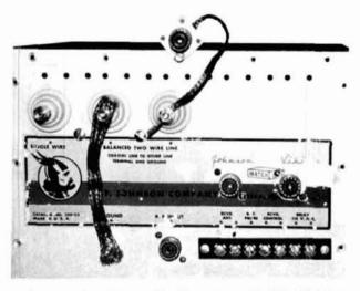
In this view the rear panel holds an extra SO-239 which has been installed to experiment with coax-to-coax tuning.
