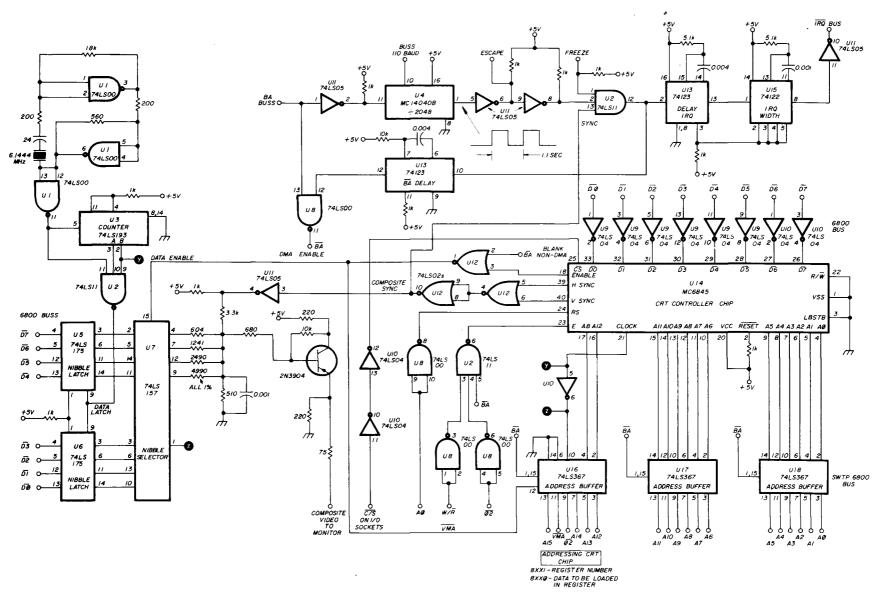
fig. 5. Schematic diagram of the video-interface card.
