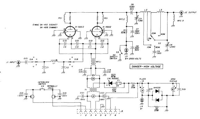
fig. 7. Schematic diagram of the 3-500Z linear amplifier.
