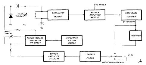
fig. 2. Frequency-locked local oscillator block diagram.
