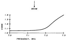
fig. 1. Four-element truncated LP antenna for 40 meters designed from data provided by W6PYK (reference 2). Curve showing VSWR is also provided.
