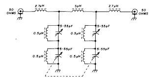
fig. 3. Whf input filter covers the range from 118 to 136 MHz. Tuning capacitors are 5-55 pF trimmers. Selectivity curve is shown below in fig. 4.
