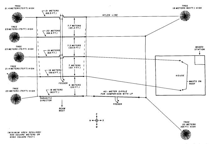
fig. 2. Author's 40-meter LP west beam using four driven elements and a director. A dipole was added for comparison in the 40-meter tests described in the text.
