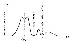
fig. 4. Selectivity curve of the vhf input filter of fig. 3.
