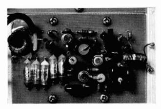
The VFO board. Note coax connection to variable capacitor.
