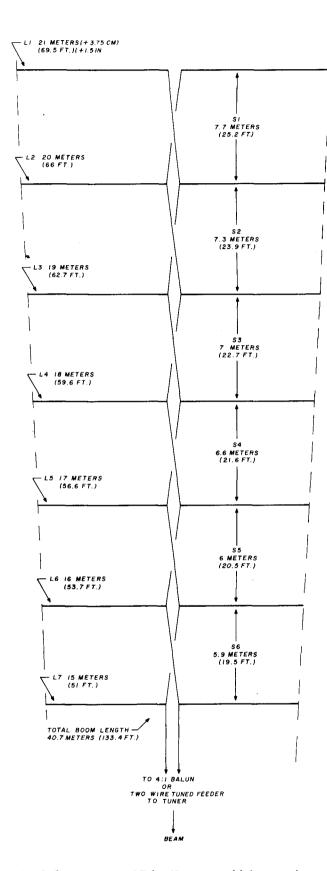
fig. 3. Seven-element LP for 40 meters with improved performance. You'll need an open space about 30 meters (100 feet) wide by about 46 meters (150 feet) long in the desired beam direction.
