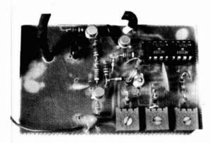
Circuit board and parts. The three square pots are at lower right; the two 555s are in one sixteen-pin socket. Q1 is at top left; Q2 at top right, which is nearest the 555s. Q3 is at bottom left. (Some resistors are standing on end.)
