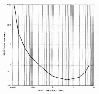
fig. 4. Measured sensitivity of the high-frequency range.
