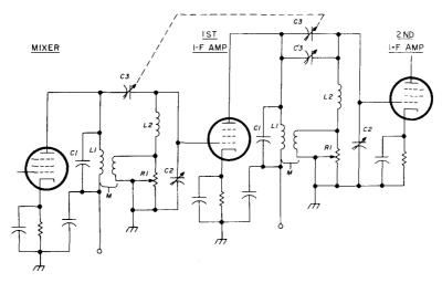
fig. 17. Two infinite rejection circuits ganged to give continuously adjustable bandwidth. In the DD-1, the i-f amplifier of each receiver has its own infinite rejection pair, and all four circuits are ganged together.
