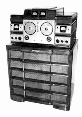
fig. 8. The late production or "jazzed-up" version of the DD-1 showing the special hi-fi loud speaker made by Jensen especially for this receiver. Note that the bandspread dial is blank. (Photo courtesy Charles Dachis, WD4EOG.)
