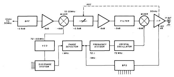
fig. 1. Block diagram of a modern high-frequency communications receiver showing the use of a 72-MHz first i-f and oven stabilized 72-MHz crystal oscillator as the reference oscillator for the phase-locked loop.
