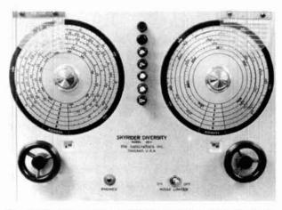
fig. 11. The main tuning dial of the monster. Note the "writ by hand" calibration on the bandspread dial.
