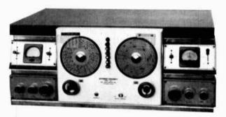
fig. 1. The tuner section only of a Hallicrafters DD-1 receiver. There was also a power supply chassis and an audio amplifier chassis. Dual S-meters sat on top of the receiver, all of which added impressiveness to the system.
