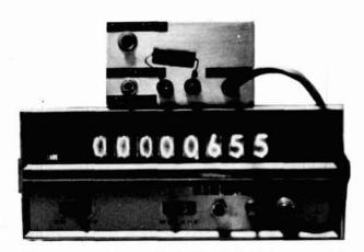
Accessory unit in use with the Heath IB 1102 counter. The extra BNC socket to the right of the counter MHz-kHz switch is for input to a divide-by-10 scaler.
