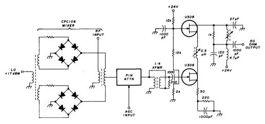
fig. 7. High-level mixer stage used in the Rohde & Schwarz HF1030 communications receiver offers noise figure of 2 dB with intercept point at +35 dBm.
