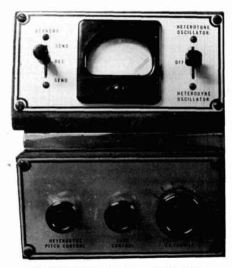
fig. 10. The left-hand control panel of the DD-1.
