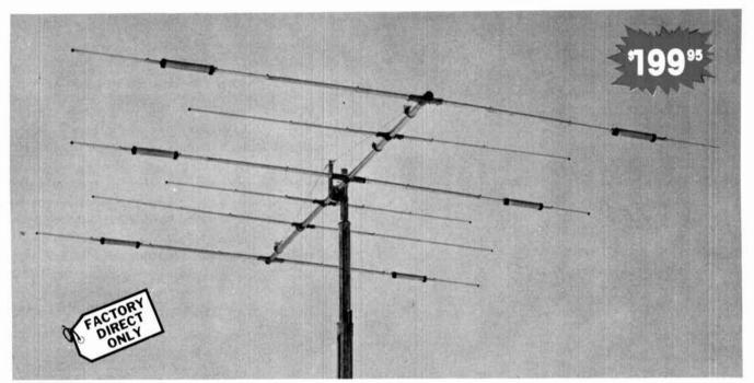
A trap loaded antenna that performs like a monobander! That's the characteristic of this six element three band beam. Through the use of wide spacing and interlacing of elements, the following is possible: three active elements on 20, three active elements on 15, and four active elements on 10 meters. No need to run separate coax feed lines for each band,
