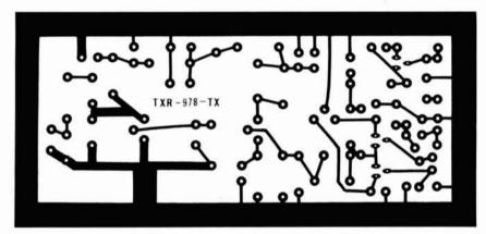
fig. 3. Above, transmitter-board parts layout. Below, transmitter board, foil side.
