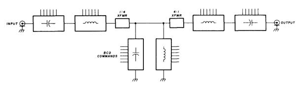
fig. 2. Preselector is microprocessor controlled, using PIN diodes to switch inductors and capacitors in the filter.
