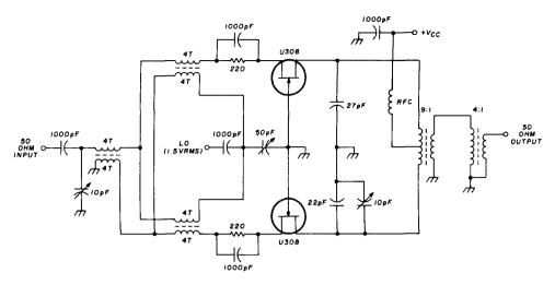
fig. 6. Circuit for a high-level balanced fet mixer. Local oscillator requirement is approximately 1.5 volts rms.
