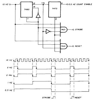
fig. 1. Schematic and timing diagram that shows the generation of the strobe and reset pulses.
