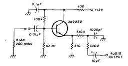
fig. 8. Linear detector is highly recommended for a-m.
