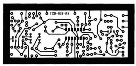
fig. 2. Above, receiver-board parts layout. Below, receiver board, foil side.
