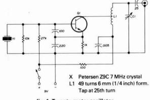
fig. 1. Twenty-meter oscillator.
