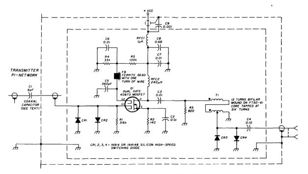
fig. 2. Schematic of a solid-state T-R switch that is suitable for use with moderate-power, vacuum-tube transmitters.
