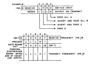
table 4. Conversion from decimal to BCD code for up-scan (increasing frequency) at the synthesizer counterjaminputs.
