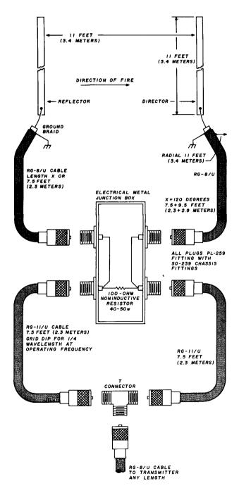
fig. 2. Construction details for the phased vertical beam for 21 MHz. Derivation of phasing-line lengths are discussed in the text.
