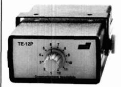
Communications Specialists has introduced a programmable 12-tone encoder, model TE-12P, available in either sub-audible or burst-tone configuration.
