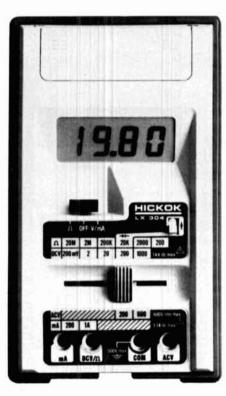
Hickok Electrical Instrument Co. has introduced the LX304, the latest model in their LX series of hand-held DVOM's. Like the LX303, the LX304 features an easy-to-read, ½-inch high, 3½ digit LCD display; automatic polarity, zero and over-range indica-
