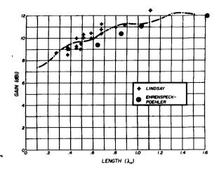
fig. 15. Theoretical Yagi beam gain envelope in dBi as a function of boom length in  $\lambda_o$ ; comparison with experimental data of Lindsay (+) and Ehrenspeck-Poehler (o).
