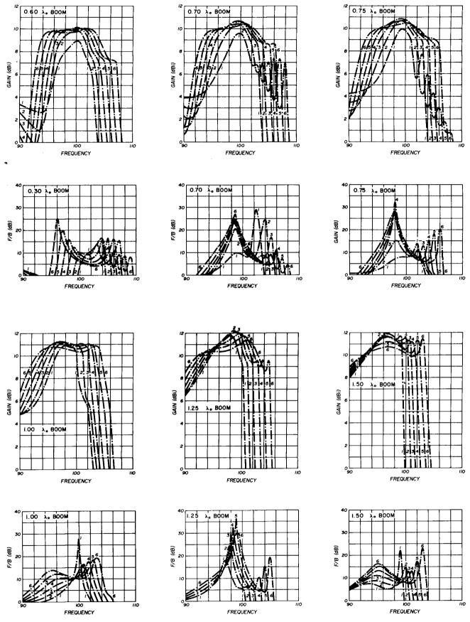
Gain and front-to-back (*F*/*B*) ratio in dB for six-element Yagi beams; boom lengths from  $0.6\lambda_o$  to  $1.5\lambda_o$ .
