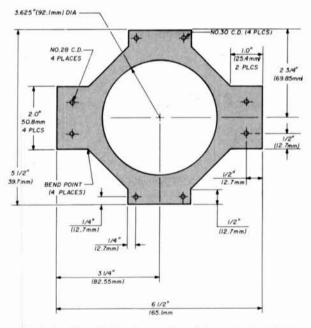
fig. 4. Anode collet and capacitor plate support pattern.
