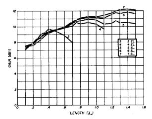
fig. 14. Yagi beam gain in dBi for 3, 4, 5, 6, and 7-element beams as a function of boom length in  $\lambda_a$ .
