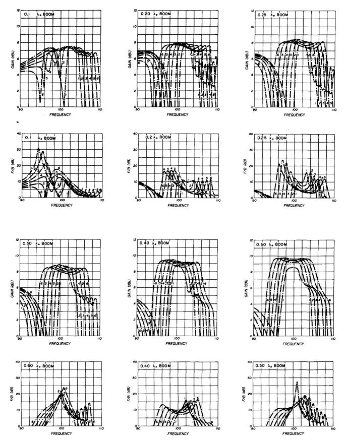
fig. 13. Gain and front-to-back (*F*/*B*) ratio in dB for six-element Yagi beams with boom lengths from  $0.1\lambda_o$  to  $0.5\lambda_o$ , and changing reflector and director lengths (see table 3 reference 5 for complete data).
