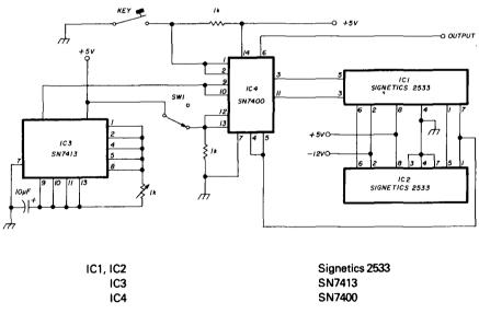
fig. 3. Schematic of the memory keyer by GW4CQT, which takes the drudgery out of contest work for sending ID, CQ, and callsigns. Memory capacity is 2048 bits.
