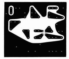
fig. 4. Printed-circuit board layout for the T-R switch. Component layout is shown in fig. 5.
