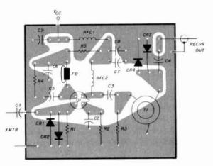
fig. 5. Component layout for the T-R switch.
