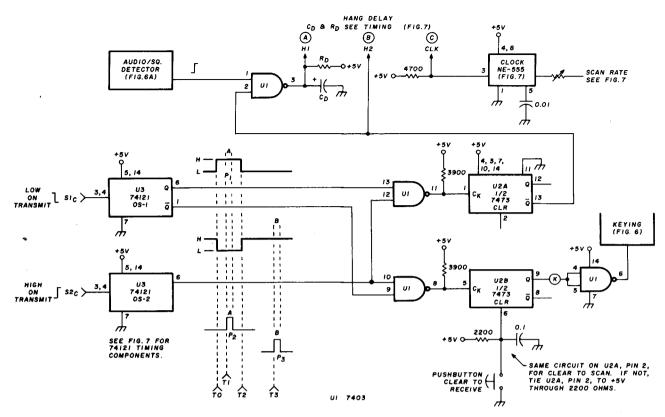
fig. 5. Push-to-talk and push-to-receive and scan/halt control circuits.
