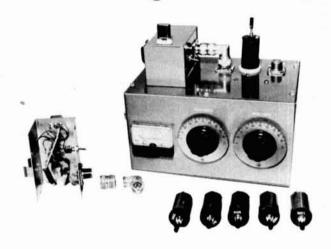
Several years ago I built the Macromatcher and the pickup coils<sup>1</sup> and used it with a grid-dip meter for antenna matching. This combination is rather cumbersome if used at the antenna terminals when the antenna is at the top of the tower. An alternative method is to use the above setup on the ground with one-half wavelength of coax to give the same characteristics as at the antenna.
