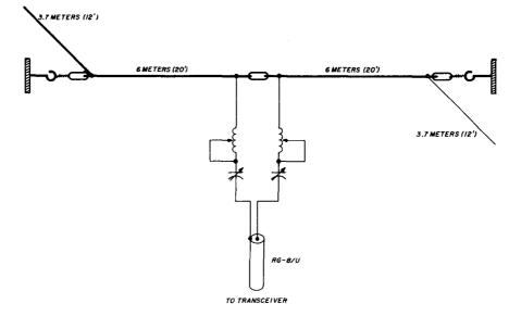
fig. 1. Author's inside 40-meter dipole. Horizontal sections occupy the length of the mobile-home attic. The end sections follow the corners of the attic to make a total radiator length of 19.5 meters (64 feet). The tuner provides near unity SWR in the phone portion of the band.
