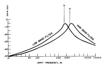
fig. 4. Filter response curves come close to the ideal; precision components are not required.
