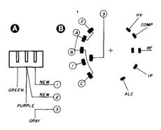
fig. 2. Modifications for selectable filter switching for the TS-820. The meter switch (S-1) is shown at (A) viewed from rear of panel. New connections to connector IF2 are shown in (B).
