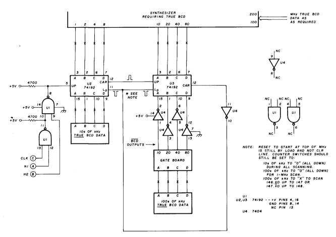
fig. 8. Schematic for synthesizers requiring true BCD input.
