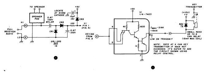
fig. 6. Input-output processing circuits. At (A) is a voltage doubler to handle the TTL gate input at U1 pin 5 (fig. 5). Component values have been chosen for maximum audio fidelity consistent with reliable halts during scanning. A keying system is shown in (B). U1, part of a 7403, will safely handle currents of 16 mA, but the relay circuit is recommended. CR4 is one of the 1N4000 family (approximately 50 volts at 1 ampere).
