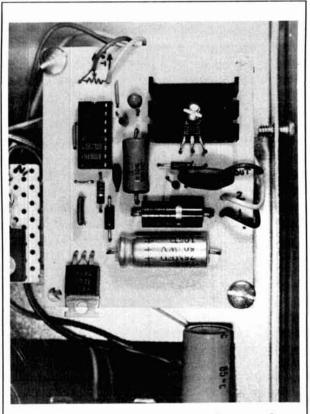
Close-up of the pulse-control unit showing parts placement. Unit is mounted on the underside of the Tailtwister control box chassis above the power transformer, as shown. Note that VR20 leans slightly to clear the bottom cover when installed.
