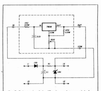
fig. 5. Schematic of the 13-volt regulator module for the rotor position is contained in the dashed box. Also shown are the connections from the module to the original circuit. R1 and VR1 are removed before connections are made. Adjust the trimpot for 13 Vdc across terminals 3 and 7 of the control box.
