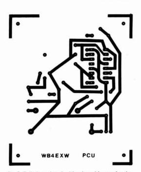
fig. 3. Full-size printed wiring board layout for the pulse-control unit. Wire side is shown.
