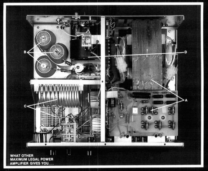
(A) A FULL KW <u>CCS</u> POWER SUPPLY WITH A 45 POUND, 1.5 KVA TRANSFORMER that plugs in for easy handling.
