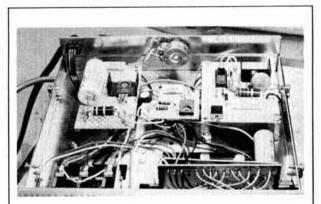
Overall view of the PCU and regulator module installed in the control box. The smaller board next to the PCU is the regulator module. Also shown is the external rateadjustment pot mounted on the rear panel. Azimuthindicating meter in this control box has been modified to a digital readout for improved accuracy.
