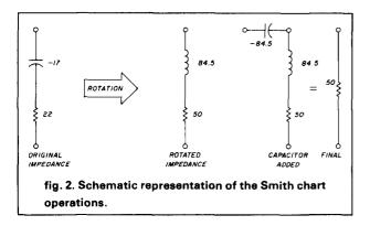
at the original impedance-measurement frequency; choice of capacitor or inductor depends on the added line length.
