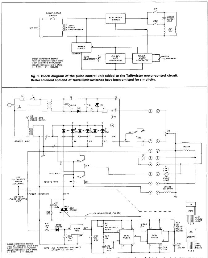
fig. 2. Schematic of the pulse-control unit and Tailtwister control box. The PCU schematic is below the dashed line that separates the two circuits. Note wiring changes to control box.
