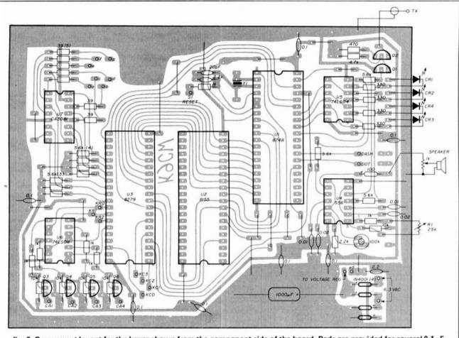
fig. 6. Component layout for the keyer shown from the component side of the board. Pads are provided for several  $0.1 \,\mu\text{F}$  bypass capacitors on the +5 volt supply line.
