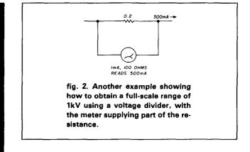
full-scale meter requires  $100 \text{ ohms} \times 0.001$  ampere = 0.1 volt for full scale; a 1000-ohm, 100micro-ampere full-scale meter requires  $1000 \text{ ohms} \times 0.0001 \text{ ampere} = 0.1 \text{ volt}$ , and so on.
