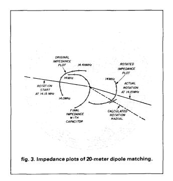
a hurry with a temporary dipole. The antenna tuner had been mislaid and the transmitter did not seem to load correctly. *RX* noise bridge readings and calculations showed a reasonable VSWR condition given in the left columns of **table 1**. A better match was desired at 14.15 MHz.
