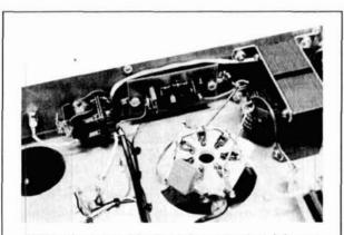
8877 socket assembly. The tube socket is a Johnson 248 submounted 1/2 inch (12.7 mm) below the chassis. Grid clips were made from a stiff copper stock and were silver plated. (An Eimac socket assembly, SK-2210, can be purchased directly from Eimac.) The Eimac Technical Data Sheet for the SK-2200 and SK-2210 air system gives detailed mounting information. If only the grid clips are needed, order Eimac part 149-842.
