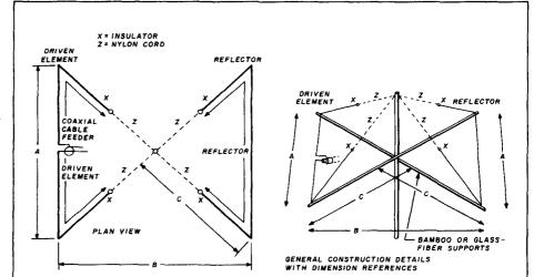
fig. 7. The G3LDO wire beam antenna for 10, 15, or 20 meters. Framework consists only of vertical mast and four bamboo or glass fiber support rods. Antenna is fed with coaxial line at midsection of driven element. Dimensions are given in table 1.
