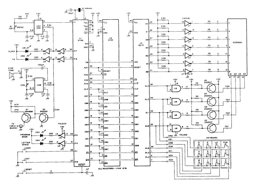
fig. 2. The keyer schematic. The four-digit LED display module may be replaced with four individual seven-segment common-anode digits.
