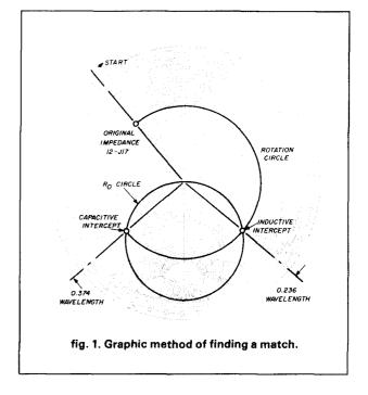
Matching requires adding an *opposite* reactance in series with the new end impedance. It is simply series resonating, so that only the resistive part remains. You have reached the perfect match!
