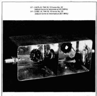
fig. 3. Photograph and inductor specifications of filter constructed from design 18 ( $F_{A_n} = 14.9 \text{ MHz}$ ).
