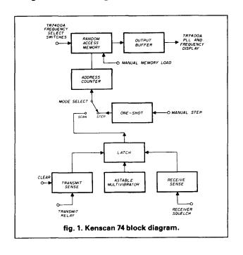
Fig. 1 is a block diagram of the Kenscan 74 mod-
