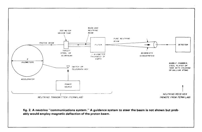
the particles except neutrinos. To detect the neutrinos, a bubble chamber or an apparatus containing approximately 1000 tons of steel is used. Even that much steel produces only about 1 interaction per pulse. A person can (and often does) stand in the neutrino beam without any effect on either the person or the beam.
