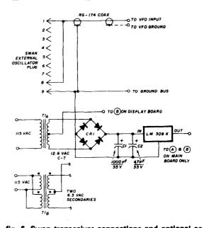
fig. 6. Swan transceiver connections and optional ac power supply. Part numbers indicated are available in Radio Shack stores. complement would be 07000.0 and obviously wrong. Changing the MSD to nines complement, or 97000.0, would correct this:
