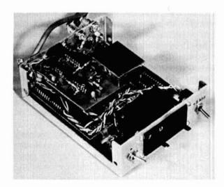
Inside the 2-meter synthesizer. All CMOS circuits are mounted on a piece of Veroboard and are supported by four standoffs. Remaining circuitry is on a doublesided PC board.
