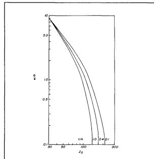
fig. 19.  $Z_0$  versus w/h for selected values of t/h for a stripline over a plane,  $\epsilon_r = 1$ .
