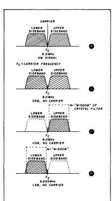
fig. 1. The derivation of DSB, LSB, and USB from an amplitude-modulated signal. Note that to obtain lower sideband, the carrier is moved to keep the desired sideband in the "window" of the filter, rather than use a separate filter, which would be very expensive. The frequencies shown are for illustration purposes only — SSB can be generated at any frequency and then heterodyned to the ham band of your choice.
