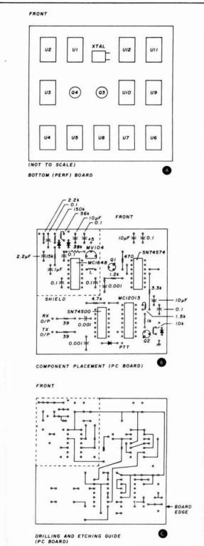
fig. 3. Circuit-board layout. All CMOS devices are mounted on a piece of Veroboard (A). (The American equivalent is Vectorboard No. 3682-4.) Interconnections on this board are made using No. 30 (0.25-mm) insulated wire on the underside. The PC board, (B) and (C), is double-sided copperclad. The bottom is left unetched to serve as a ground plane and shield. Circuit trails, made with a resist pen, are on top.
