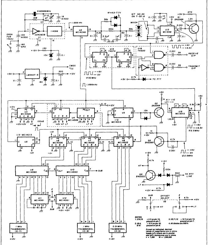
fig. 2. Schematic diagram of the 2-meter synthesizer. Reference oscillator operates in the range 5-10 MHz for best stability. Crystal is cut for 30-pF load capacitance.
