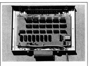
Cover removed to show parts placement on perf board. Perforated metal cover on rear is used for protection from the heat of the series-dropping resistor.
