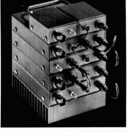
RF Pwr Out: 10 W nom. (CW & PEP) Power: 13.6 VDC @ 4 A nom. 2 meter drive: 10 W nom. (Other drive levels available on special order.) Examples of frequency conversion in the following modes:
