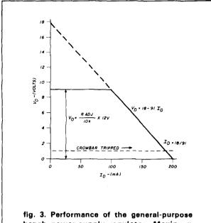
bench power-supply regulator. Maximum power condition is 98.9 milliamperes at 9 volts.
