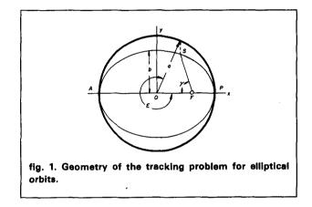
A circle has been constructed with center,  $\theta$ , bisecting AP, and with radius a. Angle E is identified as the elliptic anomaly, and  $\Gamma$  is the true anomaly. Both E and  $\Gamma$  are related to the mean anomaly, M (see eqs. A1 and A3).
