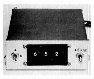
Completed synthesizer. Unit is a compact 4 by 5 by 1.5 inches (10 by 13 by 3.8 cm).
