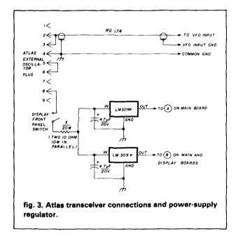
minal regulators were used, the outputs divided into A and B power connections of **figs.** 1 and 2. The 5ohm dropping resistor reduces regulator dissipation. It is mounted inside the perforated metal cover at the display enclosure back panel.
