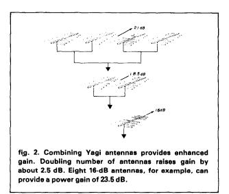
stations having more than 21 dB of antenna gain. A station having an 18dB gain antenna, for instance, should be able to hear and work moonbounce stations having an antenna gain of 24 dB. Exceptions to this rule make moonbounce very exciting.
