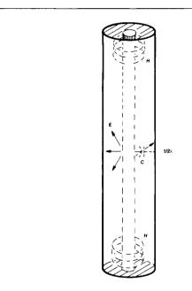
fig. 4. Half-wavelength resonant re-entrant cavity. Magnetic field, H, is at both short-circuited ends; electric field, E, is at center. Device is tuned to resonance by capacitor C.
