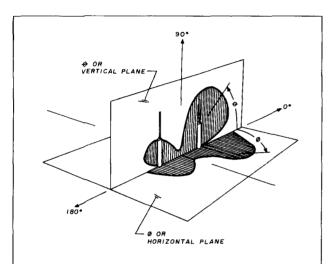
fig. 1. Two-dimensional representation of an array field strength.
