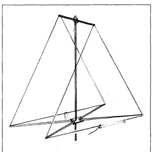
fig. 2. The conventional delta-loop wire beam. The top boom is eliminated in the Giza design, which results in a more rigid structure.
