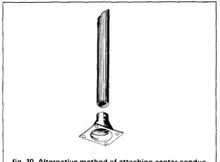
fig. 10. Alternative method of attaching center conductor to coffee can using UG-177/U or UG-106/U coax hood.
