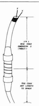
fig. 3. Typical means of constructing a quarter-wave matching section from coax. The feedpoint impedance of the beam (about 30 ohms) is transformed to the feedline impedance (72 ohms) by means of a quarterwave transformer of 50-ohm coaxial cable. Accompanying table and notes show dimensions for various bands. Center connector consists of two male connectors joined by a female (barrel) connector, for convenience. Joint should be taped and waterproofed after completion.
