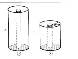
fig. 3. Quarter-wavelength resonant re-entrant cavity (A) shortened at (B) using capacitive loading to resonate to same frequency.
