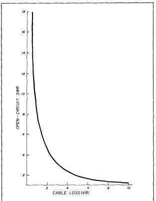
fig. 2. Open-circuit SWR as a function of cable loss (eq. 5).
