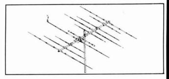
The System 40 is the answer to the DXer who does not have space to stack monobanders yet wants the advantages they offer. Through the use of our split beta matching method, only one feed line is required and complete coverage of both the phone and cw bands are available with only one setting.
