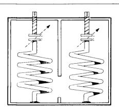
fig. 5. Helical resonator: a hybrid resonant re-entrant cavity.
