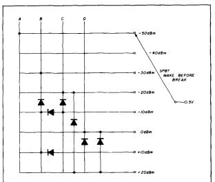
fig. 8. Diode matrix for switching input-attenuator relays. Single pole, 8-throw switch was used.
