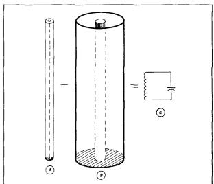
fig. 2. Quarter-wavelength coaxial cable (A) and reentrant cavity (B), both short-circuited at one end, is equivalent to a parallel resonant circuit (C).
