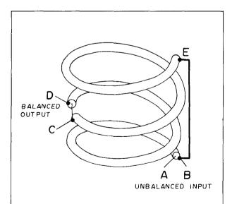
fig. 1. The 1:1 broadband coaxial balun. Actual transformer consists of seven turns closewound (3½ turns either side of the output) of RG-8X coax approximately 4 inches (100 mm) diameter. Center conductor in upper winding is not used.
