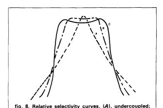
(B), critical coupling; (C), over coupling.
