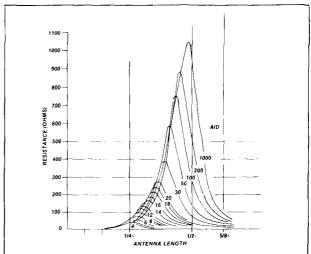
fig. 15. Terminal resistance as a function of antenna length. A/D is the ratio of antenna length to diameter.  $^{10}$
