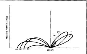
fig. 14. Vertical-angle patterns of various lengths of vertical radiators. Five-eighths wavelength, three-quarter wavelength, and full wavelength high-angle lobes are shown on right for clarity. (Note absence of low-angle lobe for full-wavelength vertical.)
