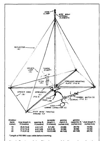
fig. 1. Design of the Giza beam with dimensions for the three high-frequency bands. Simplicity and readily available parts make this antenna a definite candidate for the homebrewer.
