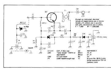
fig. 2. Schematic of wideband preamplifier. Connections also shown for use as a microwave mixer i-f amplifier.
