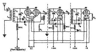
FIG. 1 - WIRING DIAGRAM OF THE RADIO-FREQUENCY END
