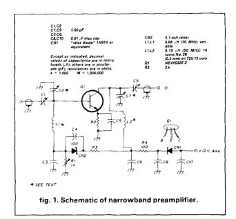
small-signal diode rated for at least 15 volts, is in series with a current-limiting resistor, R4. If a 3-k resistor isn't available for R3, a 2.7 k will work as well, although slightly more preamplifier current will be drawn from the B + supply.
