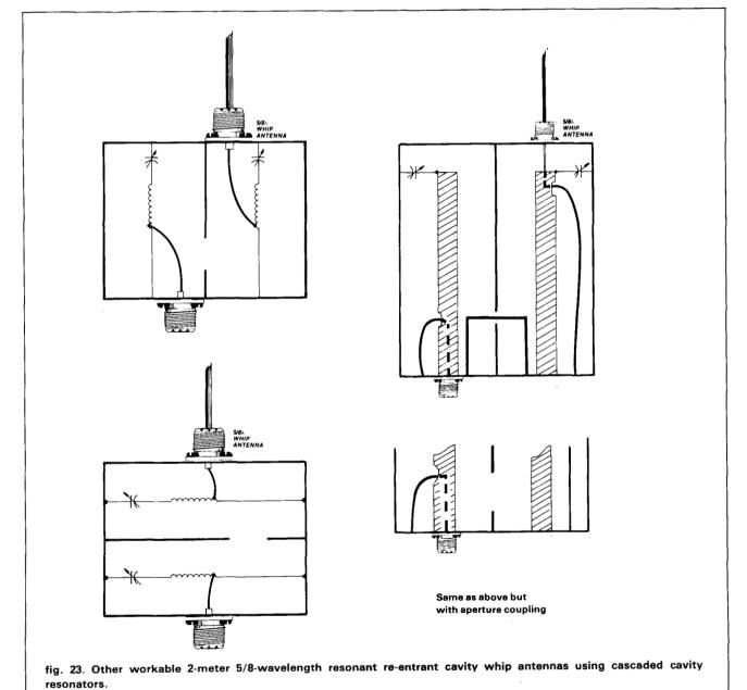
may be too high. Adjust the antenna feed pickup loop until the SWR is very low at resonance; the whip has now been resonated. The input loop may now be repositioned and reshaped for the desired degree of selectivity versus insertion loss. Keep in mind that all adjustments are interdependent.
