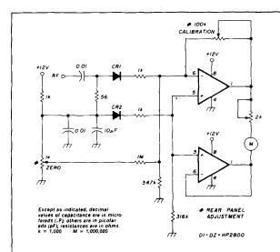
fig. 3. Biased detector schematic. CR1, CR2 are Schottky diodes. Meter is 0-100 microamps or higher. Original circuit was described by Wes Hayward, W7ZOI.
