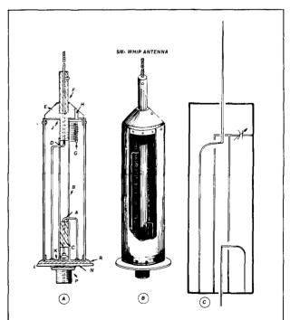
fig. 19. Five-eighths wavelength resonant re-entrant cavity whip antenna in cross section (A), cutaway (B), and schematic diagram (C).
