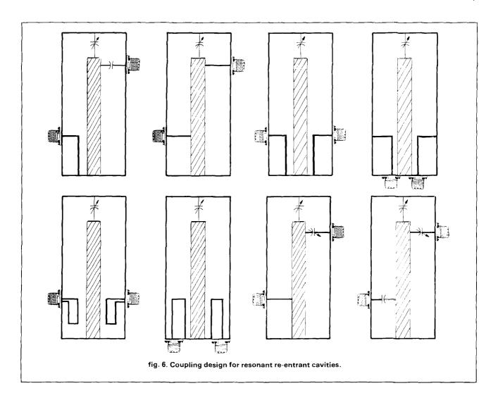
pickup loops are usually used. In some cases, direct connection to low-impedance positions on the inner conductor is used, especially where cavities are connected in cascade. Capacitive probes provide a convenient method of feeding energy to or from high-impedance circuits. Some coupling configurations are shown in fig. 6.
