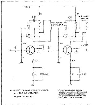
fig. 6. This 37-dB broadband preamplifier is stable, with emitter and shunt feedback. Measured input VSWR is less than 1.2.
