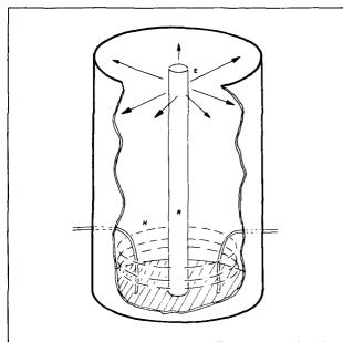
fig. 1. Concentration of magnetic field, H, and electric field, E, in a resonant cavity with a re-entrant section, R.
