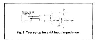
signal-to-noise ratio on a *weak* signal. (A noise-figure test setup is preferable, although many can't obtain such equipment.)
