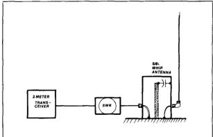
fig. 18. Coffee-can resonant re-entrant cavity used as a resonator for a 5/8-wavelength vertical. Pickup loops are adjusted for lowest SWR at resonance.
