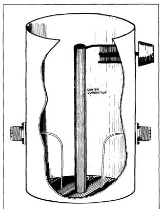
fig. 9. Cutaway of coffee-can resonant re-entrant cavity.
