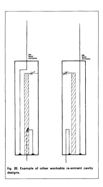
this antenna has a small insertion loss at resonance, which is about the same as the loss in the usual resonator that it replaces. However, there are bandwidth limitations under certain conditions which will be discussed later.
