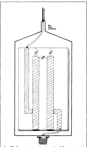
fig. 25. Resonant re-entrant cavity 5/8-wavelength whip antenna using microstrip techniques.
