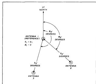
rig. 2. Geometric relationships of spacing and location, top view.
