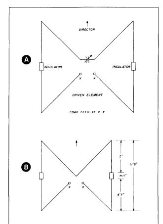
fig. 1. Schematic representation of the "butterfly" beam (A) showing the 'M'-shaped director, tuned by a capacitor, and the 'W'-shaped driven element with feedpoints X-X. It looks a bit like a quad loop, but lies flat instead of standing vertical. B shows dimensions of typical 15-meter version, constructed for lower band edge (21.0 MHz). In this figure, capacitor has been eliminated (see text).
