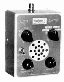
(120 dB total range with the sensitivity control). Its 3 dB antenna gain and .06 uV typical DF sensitivity allow the crystal-controlled unit to hear and positively track a weak signal at very long ranges. It has no  $180^{\circ}$  ambiguity.
