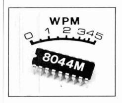
The addition of two extra pins at the end of the package permits a pinfor-pin fit with the standard 8044. One of the pins is used for a timing capacitor and the other pin drives the meter directly. This allows retrofitting in many existing keyers with relative elase. The keyer function of the 8044M remains the same as in the 8044 design, providing dot and dash memories, iambic operation, key debouncing, weight control, monitor oscillator, and extremely low power dissipation.
