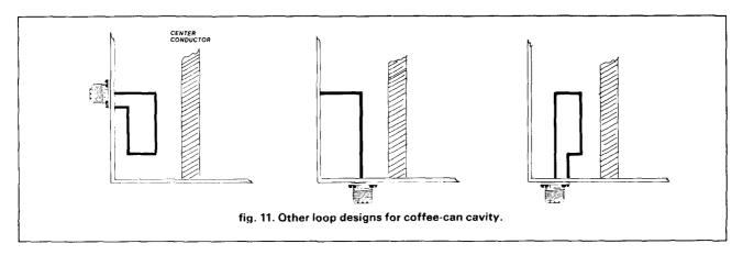
as shown. Other loop configurations that can be used are shown in **fig. 11**.
