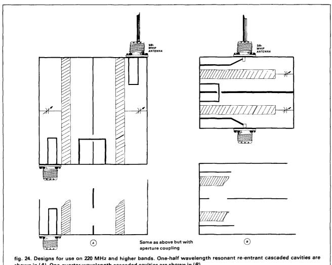
shown in (A). One-quarter wavelength cascaded cavities are shown in (B).
