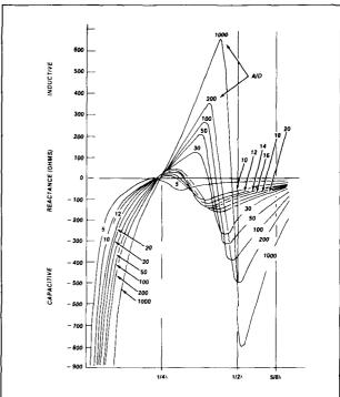
fig. 16. Terminal reactance as a function of antenna length. A/D is the length/diameter ratio.  $^{10}$
