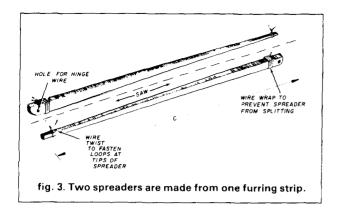
length. Attach the loop ends to the appropriate plastic insulator of the gamma match and the tuning stub. Secure the lower sides of the two loops loosely to the spreader tips with the stiff wires on each tip. Meanwhile keep the insulators centered and the two lengths equal. Pull the wires taut so that no slack exists in the spacer cords, then firmly twist the stiff wire so that the loop wires will not slip through.
