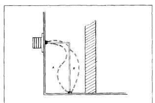
fig. 13. One method of increasing or decreasing coupling. Less coupling is at (A); more coupling is at (B).
