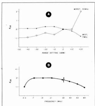
fig. 9. Power-meter step gain accuracy relative to 0 dBm (A) and relative frequency response (B). In-band flatness is less than  $\pm 0.1$  dB on all bands.
