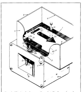
fig. 4. Mechanical mounting details for using the preamp on a Gunnplexer.
