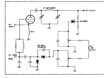
fig. 5. A unique ALC circuit using both grid and plate detection. When the grid is driven into the positive-voltage region, this voltage is doubled and fed together with the sensed plate signal to the ALC bus. The two voltages are balanced by individual potentiometer settings.
