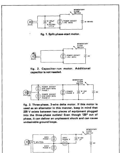
fig. 4. Three-phase, 4-wire star-connected motor. The note in *fig. 3* applies to this alternator as well.
