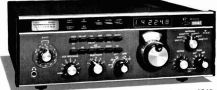
Full general coverage reception, 0-30 MHz, with no gaps or range crystals required.
