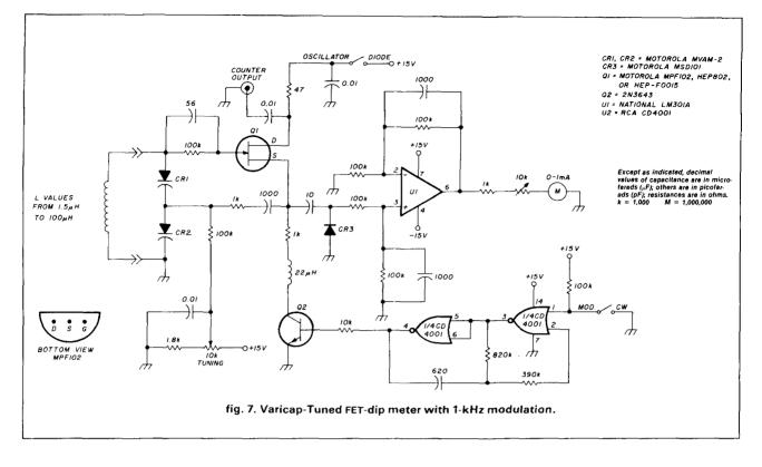
time is perhaps right to dispense with the calibration dial on the modern dip meter. Once this step has been taken, it is only a logical, short jump to replace the tuning capacitor with varicaps and use a remote dc pot to tune the dip oscillator, since no calibration scales are now needed. If the counter is not desired, the dc pot can be calibrated just as well as could the traditional tuning capacitor dial.
