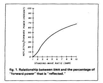
a given power level, the higher the SWR, the higher the observed current and voltage will be. If you're using RG-58/U or TV-type twin lead, *don't* use a power input over 200 watts. If you're using RG-8U with a kilowatt, beware if the SWR is more than 5.
