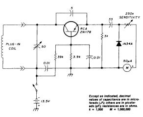
fig. 2. Typical dip meter using germanium PNP bipolar transistor with separate diode detector.
