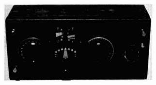
Here is a panel view of 1922 version of the Reinartz shortwave tuner, built by W. W. "Woody" Wilson, WA6KVW, from an early magazine article. He used authentic parts of that period from his extensive antique wireless collection. Switch points picked up progressive taps on the coils — an early version of band switching, you might say.
