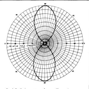
fig. 4. Radiation pattern of two collinear elements.
