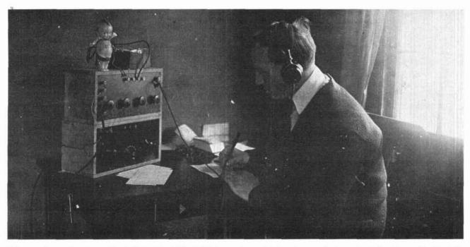
This operating position shows John L. Reinartz in 1921 with his famous tuner of that era in use, with three stages of audio amplification in the top cabinet. The spark transmitter, located in the cellar, was remotely controlled from this upstairs room. The Kewpie doll on top of the receiver was sent to him by a Canadian Amateur as a mascot — he had the famous 1QP call at that time and signed some of his message traffic "Kewpie."
