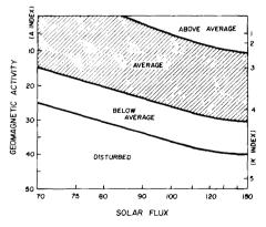
fig. 1. Relationship between geomagnetic and solar flux indexes and their combined effect on ionospheric propagation of radio signals.
