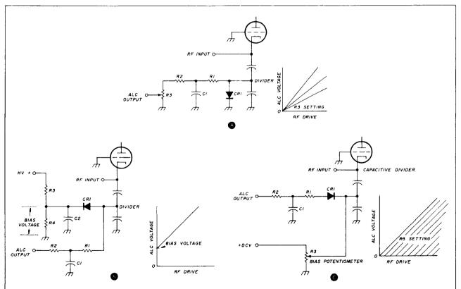
fig. 4. Examples of practical ALC circuits. Circuit at (A) is a simple system with no threshold and is adjustable by potentiometer R3. The most common ALC circuit is shown in (B), a system using a biased diode to determine the threshold point at which ALC action begins. In (C), the threshold point is made variable by using the potentiometer (R3) to set the bias to the diode.
