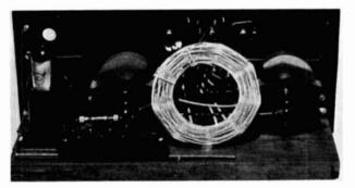
Inside view of the Reinartz tuner with spiderweb inductance, which was an improvement over the original version in June, 1921 QST. The tube is a UV-199. Gridleak resistor was in clip holder for easy changing. Note hole in panel to check on tube filament glow, controlled by varying rheostat on front panel.
