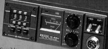
Sensible and affordable, the IC-22U offers simplicity with ease of operation. Easy to use push buttons for up and down tuning. 800 channels at the push of a button. 4 MHz coverage. EX-199 optional remotable frequency selector.
