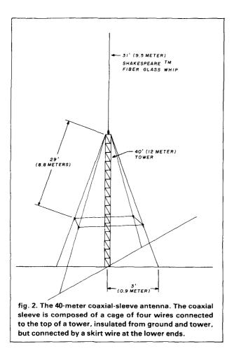
cable that runs up the center of the mast. The outside conductor of the coax is connected to the top of the tower; the center conductor is connected to the base of a free-standing, base-insulated whip at the top of the tower. (For base-station use, the tower should be grounded for lightning protection.)
