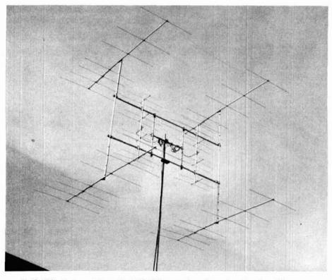
fig. 2. This photo explains why K6QXY has such a robust signal on 6 and 2 meters. The 6-meter array is composed of four seven-element KLM LPY Yagi antennas. Inside the array is the 2-meter beam, which consists of two twenty-element expanded collinear arrays.
