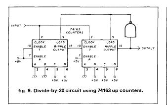
design with a device such as the 74163. It features synchronous loading; the preset loading occurs only when the required clock edge is received. A divideby-20 circuit is shown in **fig. 9**, with waveforms in **fig. 10**.
