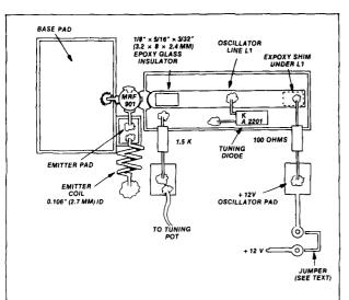
fig. 4. Details of oscillator assembly. Feedback capacitor C2 in fig. 1 is made by bending the unused emitter lead of the MRF-901 up and over the top of the transistor. A  $1/4 \times 1/8$  inch (6.4  $\times$  3.2 mm) piece of copper foil is then slid under the emitter and over the epoxy insulator and soldered to the emitter. (This capacitor is not shown in the drawing. See text for adjustment.)
