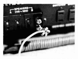
Parasitic oscillations and high-frequency attenuation (described in the text) can be avoided by installing a toroid on each speaker lead.
