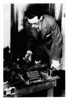
fig. 1. Charlie Atwater, nu2JN, and his pioneer 10-meter transmitter. Charlie's 1928-1929 experiments helped open this new Amateur band. Using a UX-210 driving a UX-852, Charlie's transmitter delivered about 80 watts into a Zeppelin antenna. Unfortunately, the sunspot cycle was on the downward trend. After a few exciting months 10 meters went dead, and interest lapsed for nearly eight years.
