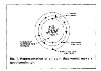
Surrounding the nucleus, however, are orbiting electrons, **fig. 1**. The electrons have a negative charge and are attracted to the positive charges of the nuclear protons. These constantly moving electrons travel in orbits around the nucleus, somewhat similarly to the way in which the planets orbit the sun. The earth is attracted to the sun by gravitational forces; electrons are attracted to the nuclear protons by electrostatic (negative to positive) forces.
