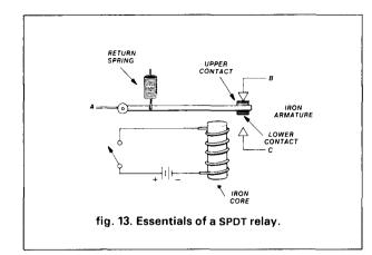
causes the armature to vibrate. However, if half of the top of the iron core piece is encircled with a copper ring, there will be an induced current in the ring that produces its own field which tends to hold the armature while the magnetic fields are alternating. This makes an ac relay.
