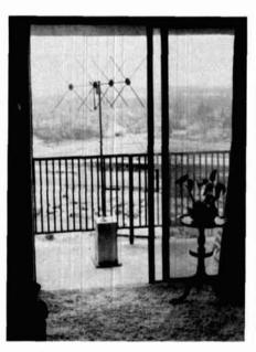
fig. 5. The compact 2-meter quad at K3AC is ideal for the apartment dweller. Sometimes Mal uses it indoors, shooting the signal through the sliding-glass doors. See text for dimensions and construction details.
