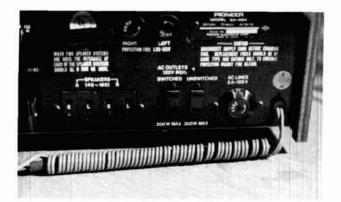
If the interference is entering the stereo through the ac line, the cord can be wrapped around a ferrite rod to form a bifilar choke.
