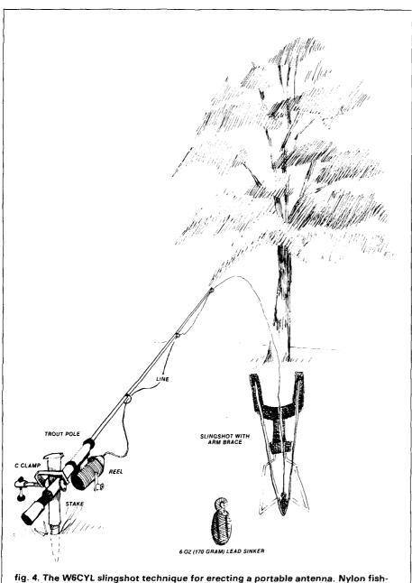
fig. 4. The W6CYL slingshot technique for erecting a portable antenna. Nylon fishing line on a trout pole is attached to lead sinker, which is then catapulted over nearby trees using an arm-brace slingshot. Bob prefers this to the bow-and-arrow technique. Try it out next Field Day. mounted at the bottom of the vertical handle, which rests back on the forearm and reduces the force on the handle when you draw back on the rubber tubing bands for a long shot into a tall tree.
