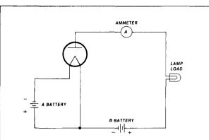
fig. 5. Vacuum diode with a filament or A-battery, a plate circuit or B-battery, ammeter in the plate circuit, and a lamp as the load.
