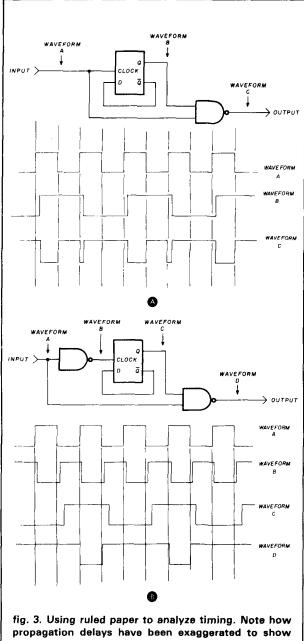
fig. 3. Using ruled paper to analyze timing. Note how propagation delays have been exaggerated to show glitch formation. Circuit of *A* is the same as in *fig. 1; B* adds a gate to eliminate the output spike.
