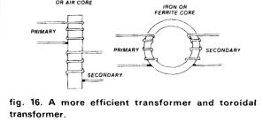
ber, P = EI will always be slightly more than the product of the secondary E and I, the difference being due to core losses and other inefficiencies. Since the power output can never exceed the power input, the power ratio is usually considered to be about 1:1 for all iron-core transformers.
