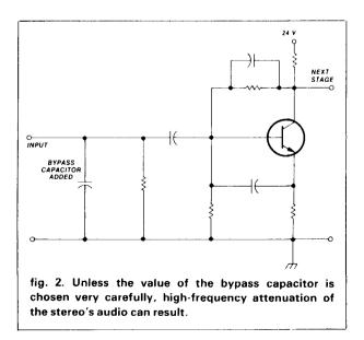
How much capacitance is too much? Specification sheets for good-quality phono cartridges include data for the optimum load resistance and maximum load capacitance. High-frequency attenuation can be avoided by keeping the total capacitance well below the maximum tolerable capacitance.
