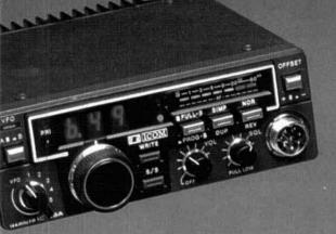
The best 2 meter multimode mobile on the market today, the IC-290A has features to make multimode mobile a snap. 2 VFO's, 5 memories, priority channel, memory and band scanning, squelch on SSB, selectable AGC and NB, and RIT. Touchtone <sup>™</sup> encoding provided with HM-8 microphone standard.
