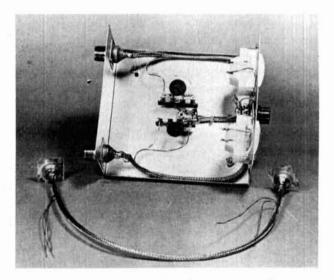
Interior of the SWR meter showing component layout. The sampling assembly (foreground) was made from RG-58/U coaxial cable.
