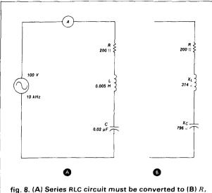
fig. 8. (A) Series RLC circuit must be converted to (B) R,  $X_L$ , and  $X_C$  values to compute it, using the given frequency.
