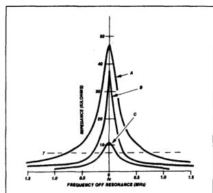
fig. 6. Comparison of relative rejection of 15-meter traps. A represents the single-element trap connected as described in the text. B represents the commercial trap of conventional design that was evaluated by the author. C represents the single-element trap's rejection if improperly connected as discussed in the text. Note the 7 kilohm bandwidth improvement over the conventional design. The rejection is plotted versus frequency away from resonance ( $f_c$ ).
