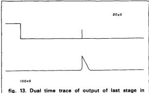
counter cascade of fig. 12. Upper trace is 20  $\mu$ sec per division. Bottom trace is expanded time of upper trace center at 100  $\mu$ sec per division to show spike.
