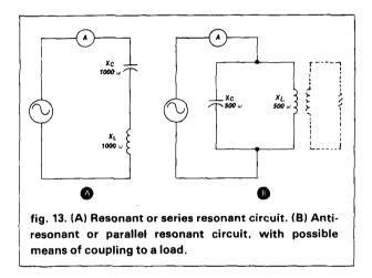
will lag the current by 90 degrees, and the  $X_L$  voltage will lead the current by 90 degrees. These two equal but opposite voltages (180 degrees out of phase) cancel, leaving the source looking at a zero voltagedrop load, or a short circuit. A series resonant circuit acts as an impedance of zero ohms, and if there is no resistance in the line the ammeter and the source might burn up.
