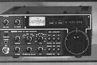
The IC-451A provides space age technology for space communications. Satellites, EME and local modes of communications are available by basing a system on ICOM's full featured 432 MHz transceiver.
