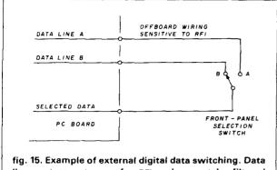
lines act as antennas for RFI and cannot be filtered without destroying data.
