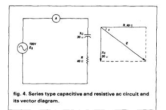
viously, an inductor always has its current lagging behind the circuit voltage by 90 degrees. A capacitor always has its current *leading* the circuit voltage by 90 degrees. These reactive phase shifts are important in the operation of ac circuits. For one thing, it is possible to add capacitance to an inductive-resistive circuit to reduce a phase lag of the current caused by the inductance.
