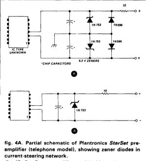
fig. 4B. StarSet preamplifier modified for radio use.
