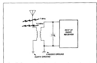
fig. 15. Resonant circuit used at the input of a radio receiver to select the desired frequency to receive.
