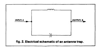
as an illustrative aid. If flexible cable such as RG-58/U is used, a rigid form such as PVC plumbing stock would be required.
