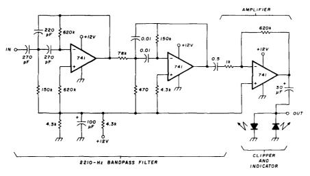
fig. 1. Diagram for RTTY tuning indicator.
