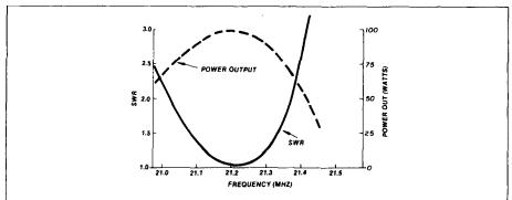
fig. 1. Representative SWR vs power output for solid-state transmitter. As SWR of antenna increases, power output of transmitter drops rapidly. At 21.45 MHz, for example, 100 watt nominal output is reduced to less than 30 watts because of high SWR on antenna system. A line flattener will reduce input SWR and boost power output of the transmitter.
