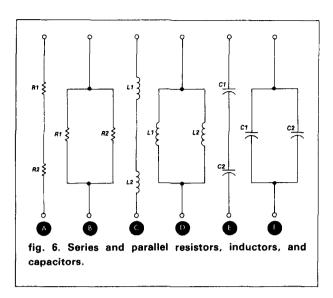
tance. Now, all oppositions, resistance and reactances, if in series, are found by simply adding the component values. Similarly, when in parallel you use the parallel resistance type formulas to determine the total oppositions, substituting *Xs* for *Rs*.
