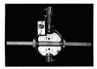
Details of the electrical outlet box, which forms the base of the 10-meter antenna. Wooden dowels are handles for working the bottom piece of conduit (not shown) into mud or sand.
