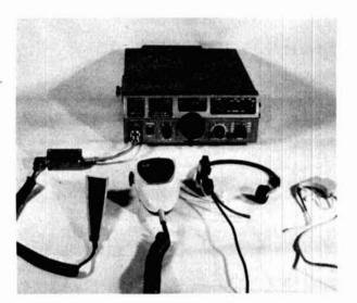
Current-source adapter allows Amateur transceivers to use simulated-carbon microphones such as (left to right) Telex aircraft microphone, Motorola mobile microphone, Pacific Plantronics MS-50 and *StarSet* headsets.
