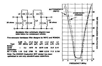
fig. 1. Calculated bandpass filter responses based on an inductor Q of 100 at 5.3 MHz.
