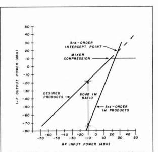
fig. 2. Third-order intercept point is determined by extrapolating the desired product curve beyond the mixer compression point and intersecting it with the third-order IM-product curve. (From the ARRL Radio Amateur's Handbook, 1981.)
