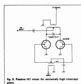
With suitable bias applied, the intercept point can be as high as +40 dBm with little difficulty in reproduction. This technique is currently used by the Racal RA6790 receiver and by the AGC Telefunken E1700 receiver.
