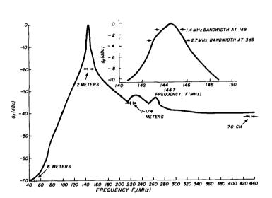
fig. 3. Preamplifier frequency response.
