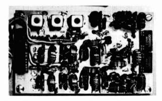
Typical board construction as shown on the filter board. Terminal strips are soldered to PC material directly. Components are supported on strips and groundplane. Breadboard rf circuitry may be constructed rapidly with this technique.
