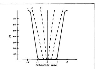
fig. 3. Typical i-f response curves. Curve 1: Built-in 2.4-kHz filter. Curve 2: Added 500-Hz filter. Curve 3: Alternate 250-Hz filter.
