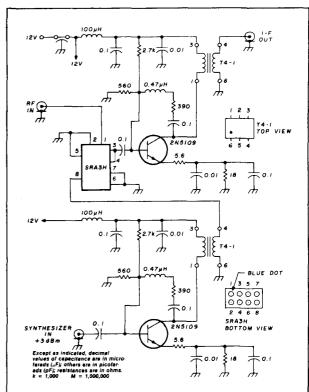
fig. 4. First-mixer schematic (M1 module). One of the 2N5109 feedback amplifiers is used as an i-f post amplifier, and the other increases the synthesizer injection signal to 17 dBm. Amplifier gain is about 14 dB; the output compression point is 23 dBm.
