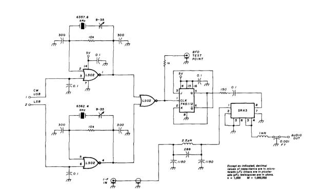
fig. 9. BFO and product-detector schematic (M6 module). The BFO consists of two crystal oscillators, one for LSB and one for USB/CW. An SRA-3 double-balanced mixer is used as the product detector. Unit gives excellent results when driven with a square-wave carrier.
