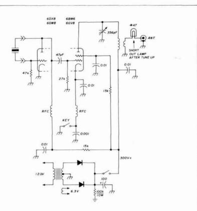
fig. 2. VK5EK's tongue-in-cheek reply to the modern QRP solid-state transmitter. Why use six expensive transistors and about 100 components when one tube and two diodes, plus a handful of flea-market components will do the job? Old-timers will certainly remember low-power transmitters of this general type. (Drawing adapted from Amateur Radio magazine, a publication of the Wireless Institute of Australia.)
