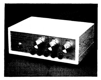
The Datong Model FL1 audio filter, as well as being a variable CW filter with noninteracting center frequency and bandwidth controls, can also automatically locate, track and notch out single interfering heterodynes. It continually searches from 300 to 3000 Hz and needs only about two seconds to achieve lock. Notch bandwidth in the AUTO mode can be only 20 Hz. The notch is therefore inaudible while searching.
