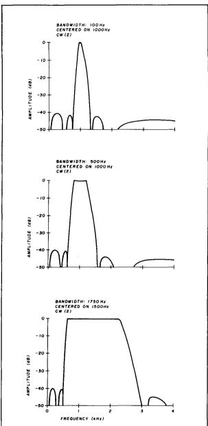
fig. 4. Three examples of the response in the CW(2) mode. The control settings correspond to those in fig. 3; and, in fact, the responses in fig. 3 are those of fig. 4 combined with the response of a two-pole peaking filter (as in fig. 2C). Note the relatively square passband. These curves are also typical of those obtainable in the SSB mode (but of course using different knob settings). Note also the two-notch stop-band responses characteristic of the five-pole elliptic function filters.
