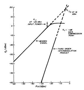
fig. 4. NE73437 preamplifier input/output and intermodulation response.
