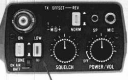
· HI/LO power output selection Allows operation at 2.5 watts or 300 mw RF output.
