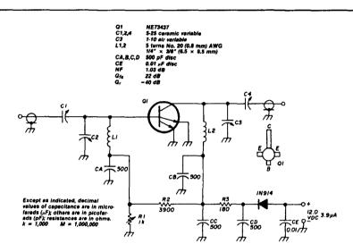
fig. 1. Schematic diagram of preamplifier.
