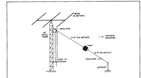
fig. 3. The 5-band sloper antenna of VE3CPU as described in reference 3. The antenna is used on bands between 10 and 80 meters. It is one-half of a regular trap dipole using a metal tower as a ground counterpoise. One trap dipole kit makes two antennas, so you can split a kit with a friend who also wants this antenna. Braid of coax is grounded to top and bottom of tower, and center conductor connects to the sloper wire.
