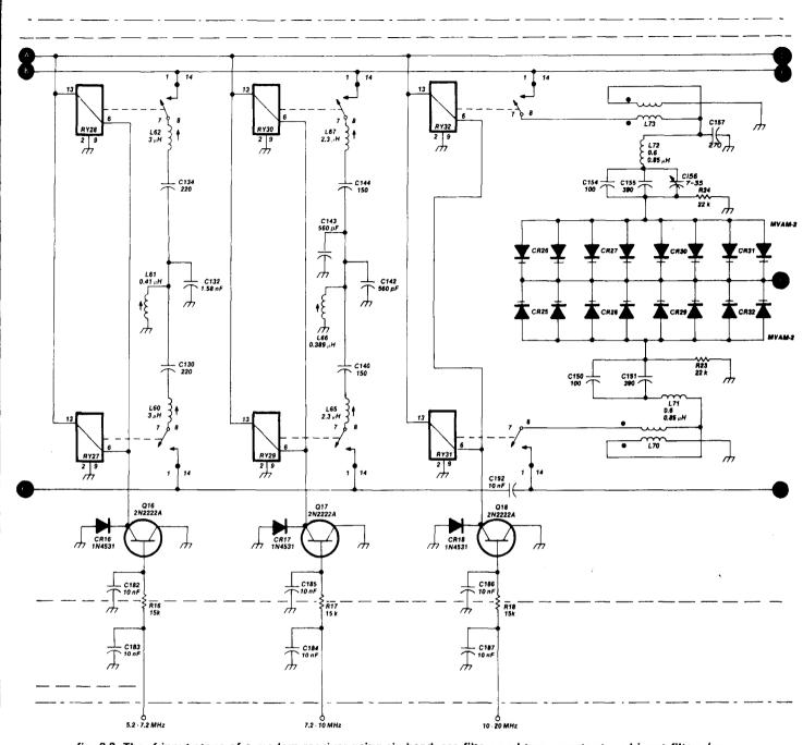
fig. 2-2. The rf input stage of a modern receiver using six bandpass filters and two varactor-tuned input filters (continued).
