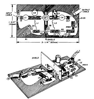
fig. 2. PC board and component layout. Note that the NE73437 device package has three equal-length leads and a longer (collector) lead. The base lead is opposite the collector lead.
