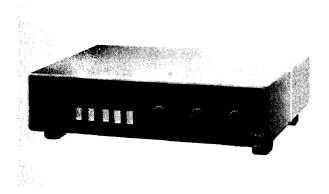
Datong's Model FL2 contains three linearly voltagetuned filters: a five-pole elliptic function lowpass, a similar highpass, and a two-pole peak or notch. The three filters can be tuned independently with separate knobs, or ganged to simulate a bandpass filter with independent center frequency and bandwidth controls. Precise tracking by all twelve poles of filtering is achieved by using pulse-width modulation techniques to simulate twelve identical voltage-controlled resistors.
