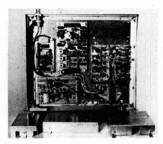
Bottom view of receiver with shields removed. Small board in the upper left is the rf preamplifier. To its right is the filter board. On the right side is the crystal-oscillator board, and in the lower left is the audio-AGC board. All except the audio board are normally covered with aluminum shield boxes.
