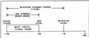
fig. 1. Performance characteristics for the receiver example discussed in the text. Shown are IMD dynamic range (93 dB) and blocking dynamic range (113 dB).
