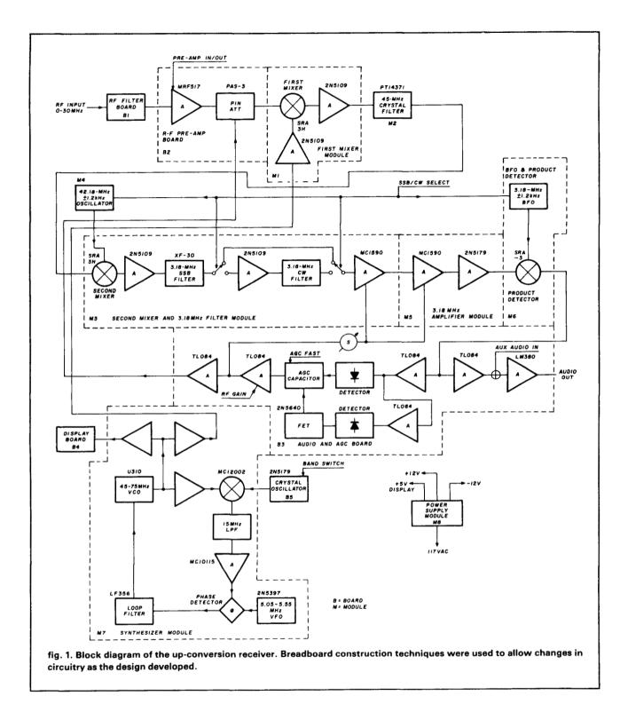
pass filter. The input filters are followed by an rf stage. This stage may be switched in when high sensitivity is required, or it may be switched out when maximum resistance to overload is needed. The high sensitivity is useful on a quiet 10-meter band or when an inefficient antenna is used.
