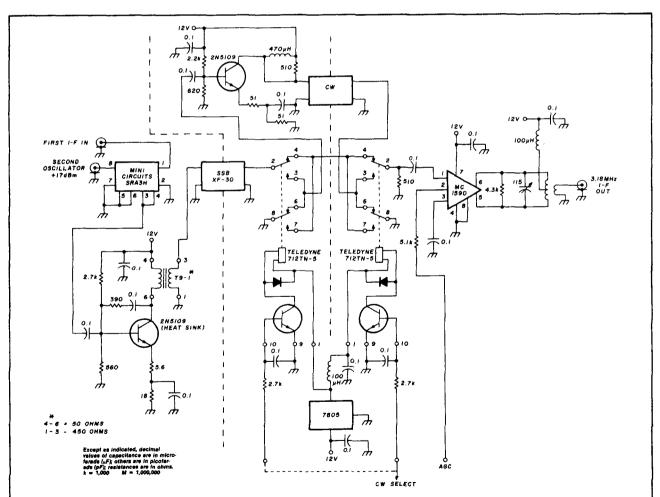
fig. 6. Second mixer and 3.18-MHz crystal filter schematic (M3 module). This high-level unit preserves good high-amplitude performance for frequencies within the 45-MHz filter passband.
