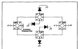
fig. 3. Schematic diagram of double-balanced mixer with two diode bridges, Model CPC106, developed for the HF1030 receiver.
