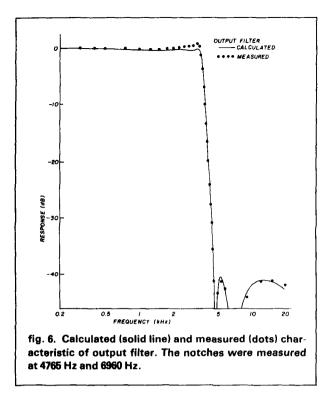
carrier frequency used; that is, above 4500 Hz. On the other hand, this filter must pass the entire spectrum of interest — for a maximum carrier frequency of 2300 Hz and a maximum video frequency of 750 Hz, the filter cutoff frequency should not occur below
