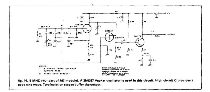
The VFO has been very satisfactory in operation; however, I could have used heavier material than a minibox, because a shift of 100 Hz is noticeable if the receiver is turned upside down while listening to a CW signal. Flexing of the tuned circuit components causes this problem.
