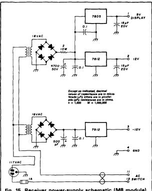
fig. 15. Receiver power-supply schematic (M8 module). Full-wave bridge circuits provide regulated positive and negative voltages for the receiver. The short-term stability characteristics of this oscillator determine the over-all receiver performance. Therefore, high-Q components should be used in the oscillator tank circuit.
