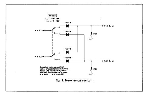
permits use of two, more precisely controlled tuning ranges for the VCO.
