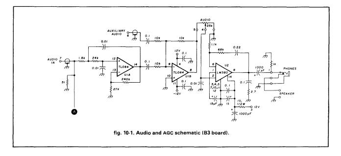
use, because much of the "operating character" of the receiver stems from its AGC system. One need only to listen to some of the modern transceivers to note that an otherwise adequate receiver can be almost ruined by poor AGC system design.
