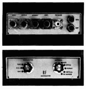
Front view and rear view of the home made rf-power distributor.
