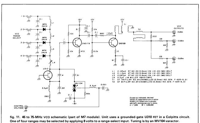
A 2N5179 isolation amplifier couples a small amount of VCO output power to a 2N5109 power amplifier. This amplifier drives a two-way power divider. One output goes to the first mixer module at a 3-dBm level. The other output is split to provide synthesizer feedback to drive the display module.
