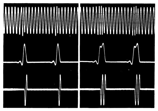
fig. 10. Overall response (bottom) to burst-modulated 1800-Hz sine wave (top) applied to converter input, producing at TP3 a video signal (center) alternating between -1500 mV and -2300 mV. Burst duration 1100  $\mu$ s (left) and 555  $\mu$ s (right).
