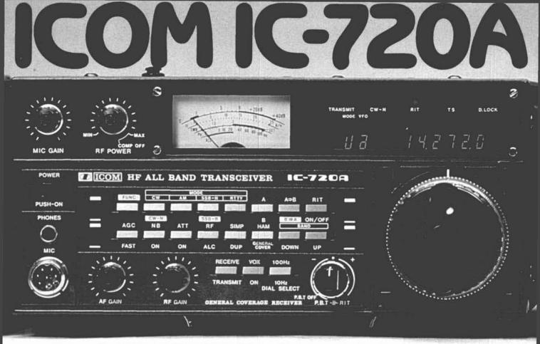
Multi mode operation includes CW/AM/ SSB/RTTY — Normally used side band selected automatically.
