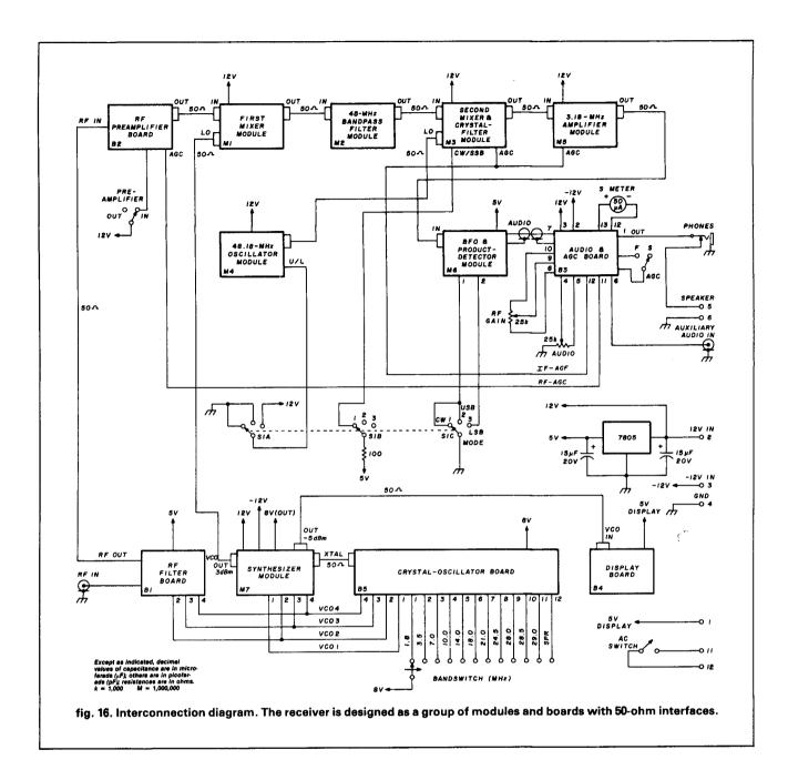
Several board construction techniques are used. The rf circuitry is built onto blank printed-circuit material. Miniature terminal strips are soldered to the boards, and the components are mounted on the strips. This method requires no hole drilling except for the four mounting holes. The audio-AGC board is built on a VERO<sup>TM</sup> card, and the display module uses wire wrap. All boards have ground planes and use extensive bypassing.
