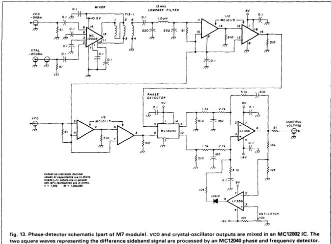
The LF356 IC operates as a differential loop filter.
