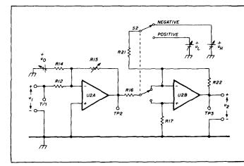
fig. 5. Processing of video signal. Switch S2 selects between positive and negitive contrast of the input a-m signal.
