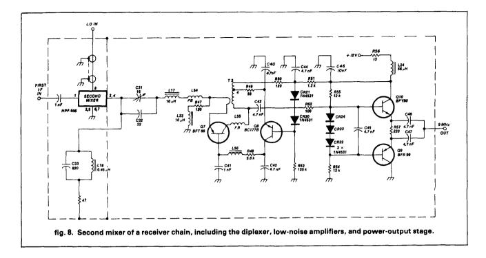
feedback, and extremely low distortion. The noise figure is now determined by the BFT66 stage, and the second stage contributes very little. The other advantage of this circuit is that there are no tuned circuits; therefore, it can be used from a few hundred kHz to almost 100 MHz. This makes this circuit design very useful.
