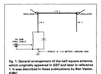
**4.** Once the low point of SWR has been set at the desired portion of the band (no matter what its value), proceed to adjust the low-side tap  $\frac{1}{4}$  to  $\frac{1}{2}$  turn at a time to get a match of 1.2:1 or better at the desired operating frequency.
