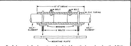
fig. 4. Log-periodic elements are insulated from the boom by a length of PVC plastic tubing. Two top bolts pass through element and tubing to make connections to transposed transmission line made of 1/4-inch-diameter tubing. U bolts passed over PVC tubing to clamp element firmly to mounting plate, which is attached to boom by two additional U bolts.
