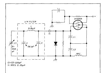
fig. 3. Tentative circuit for a VXO using an artificial quarter-wave line to transform a variable capacitor to a "phantom" variable inductance. The crystal "sees" an inductance that is variable continuously from zero to 35  $\mu$ H by means of  $C_T$ . Omitting the left-hand C, the variable capacitor must have the range 87-301 pF approximately.
