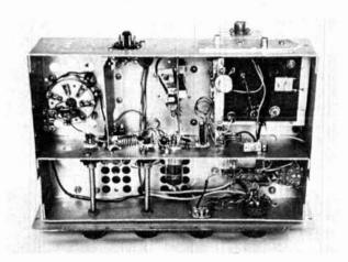
Underchassis view. Controls at lower left are, from left, the 5894 grid control, C5; 12AU7 plate control, C4; bias-adjust pot, R4; and the grid-meter switch. The 5894 PA tube-base compartment is at upper left. Shielded box at upper right houses the heterodyne oscillator.
