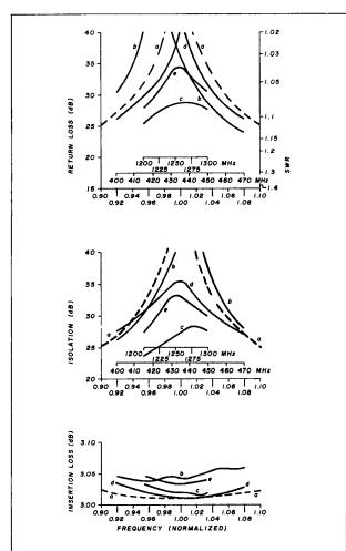
fig. 5. Performance of a Wilkinson Divider using 70ohm quarter-wave lines: curve a: theoretical; b: 70-ohm semi-rigid lines at 432 MHz; c: 70-ohm semi-rigid lines at 1296 MHz; d: 70-ohm microstrip at 432 MHz; e: 70ohm microstrip at 1296 MHz.
