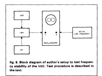
The beat between the oscillators generally holds to within about 5 Hz over a one-hour period when both are stabilized. Since this is probably as good as the crystal standard, I conclude that the phantom-coil VXO is about on par with ordinary crystal oscillators.
