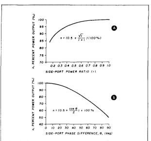
fig. 9. Percentage output power remains at greater than 97 percent of the sum of the two inputs, A, for side port power ratios to 2:1. The power output remains greater than 97 percent, B, for phase differences  $\pm$  20 degrees.
