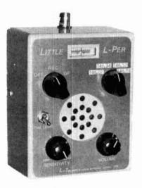
(120 dB total range with the sensitivity control). Its 3 dB antenna gain and .06 uV typical DF sensitivity allow the crystal-controlled unit to hear and positively track a weak signal at very long ranges. It has no  $180^{\circ}$  ambiguity.
