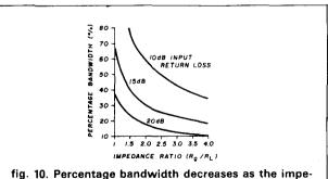
fig. 10. Percentage bandwidth decreases as the impedance transformation of a Wilkinson Divider increases.
