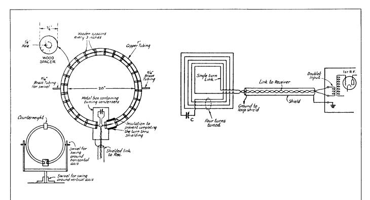
fig. 2. A reproduction of the 1938 QST drawings of the W6GPY receiving loop antenna for 160 meters. An electrostatic shield made of copper water pipe surrounds the four-turn loop. One end of the pipe is insulated from ground so as not to include a shorted turn adjacent to the loop. This deluxe design was movable in both azimuth and elevation and, by removing one turn from the loop, was capable of operation on 80 meters.
