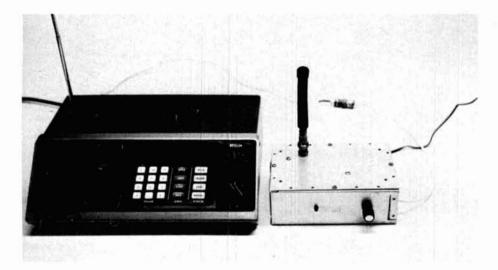
The wireless 220-MHz converter alongside a programmable scanner. The converter input antenna in this version is a rubber ducky, and the output antenna is a 33-inch (82.5-cm) length of coax with the braid stripped back about 19 inches (47.5 cm).
