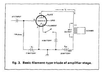
in the early days of radio. Essentially all radio equipment made before about 1955 used vacuum tubes of the triode type or improvements on the triode. Even today, many of the higher power transmitter amplifiers have one or more vacuum tubes as the active devices in them.
