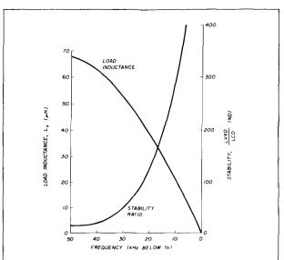
fig. 1. The LXVO can exceed a tuning range of 50 kHz on 40 meters, but the stability will decrease with range. Left-hand ordinate, equivalent load inductance versus frequency shift below crystal series resonance,  $f_{\rm s}$ . Right-hand ordinate, stability ratio of the LXVO with respect to an LCO versus frequency shift below crystal series resonance. (HC6/U crystal, 40-meter LVXO.  $C_0 = 6 pF_{\rm s} r = 250.$ )
