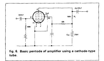
get to the screen grid. This forms a *pentode* (five-element) tube. Pentodes have even greater gain than tetrodes, and are found in most of the high-frequency amplifier stages of almost all vacuum-tube Amateur equipment in use today.
