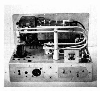
The 5894 plate lines have been bent back upon themselves to save space. Metal box behind plate lines houses the receive converter.
