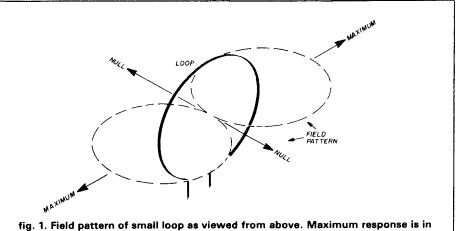
fig. 1. Field pattern of small loop as viewed from above. Maximum response is in the plane of the loop and nulls are at right angle to the loop. This is the reverse of the pattern of the larger "quad" loop whose maximum response is at a right angle to loop plane.
