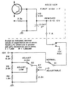
fig. 3. Simple circuit for desensitizing repeater receivers for weak input signals.
