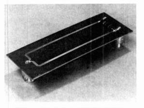
Wilkinson Hybrid using printed circuit board.
