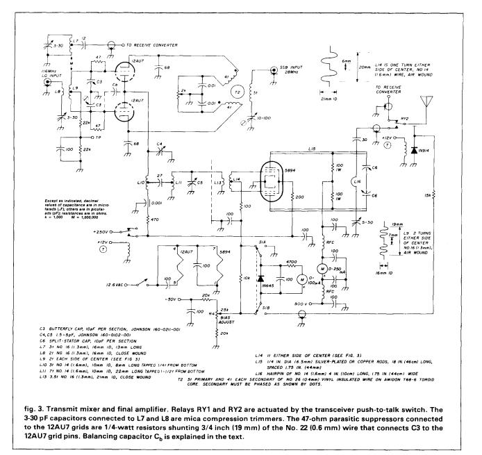
damental. It can be set to frequency with a griddipper by temporarily connecting C1 across L3.
