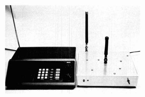
A "de-luxe" version of the converter using rubber ducky antennas for input and output.
