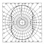
The radiation pattern of a horizontal one-wavelength antenna for a 30-degree vertical angle is:
