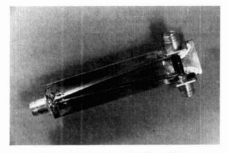
Wilkinson Hybrid using semi-rigid coaxial lines.
