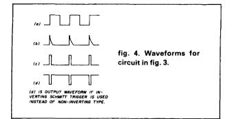
before the square wave goes down again. Again, the diode cuts off the negative part of the wave. The waveforms are shown in **fig. 4**.
