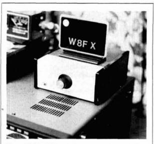
Clegg AB-144 "All Bander" atop author's KLM-2700 2meter transceiver. The KLM-2700 directly tunes 10 meters by means of an internal OSCAR receiver, so the AB-144 isn't necessary for 10-meter fm reception. The AB-144 up converter is used here to continuously receive 100 kHz to 30 MHz on the KLM-2700.
