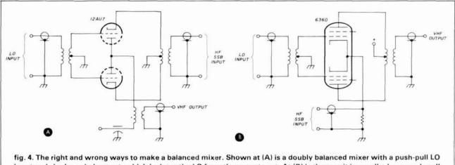
input and single-ended output, which isolates the LO from the output port. At (B) is the way it is usually done, push-pull in and push-pull out, which provides no isolation for the LO in the output.
