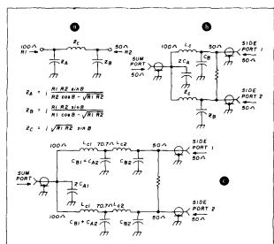
fig. 7. A pi section of lumped constants, A, forms the quarter-wave section in a single-section Wilkinson Hybrid, B, and eighth-wave matching sections in a double-section Wilkinson Hybrid, C.
