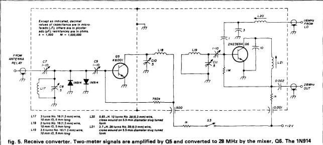
diodes at the input are for overload protection.
