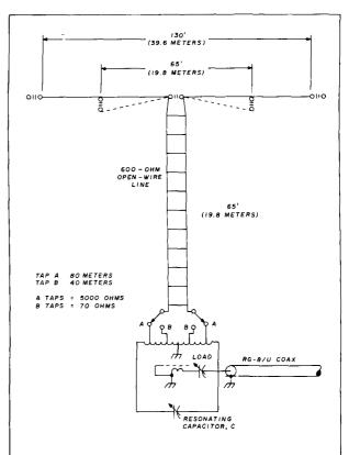
fig. 1. This center-fed dipole has an omnidirectional pattern with a 70-80 degree vertical radiation angle on the 80-meter band. On the 40-meter band, the antenna becomes a full wavelength long, with a vertical radiation angle of 30 degrees, but with a deep null normal to the plane of the wire. The omnidirectional pattern can be restored on 40 meters by adding a 40-meter dipole in parallel with the 80-meter dipole. See text for tuning instructions.
