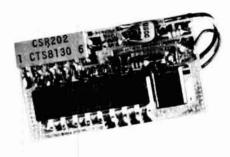
using jumpers. Measuring just  $1.45 \times 0.8 \times 0.13$  inches, the SS-32M may also be used in other applications where size is critical. Priced at \$29.95.
