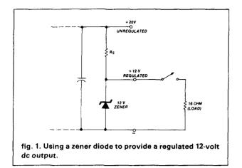
value of  $R_s$  is computed to be R = E/I, or 8/1, or 8 ohms. Its wattage rating would have to be at least P = EI, or 8(1), or 8 watts. Any 8-ohm resistor with a power rating over 8 watts would be satisfactory.
