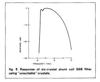
Ripple increases at the low end and decreases at the high end. Without going into details, the deviations in the reactance of the crystal branch with shunt inductance from the reactance of the series LC branch alone are opposite from the deviations with crystal shunt c.
