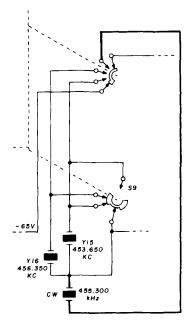
fig. 1. Heavy line shows addition of new CW BFO crystal to Collins 75S-3.
