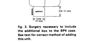
sanded the piece of box to final dimensions with No. 400 silicon paper.
