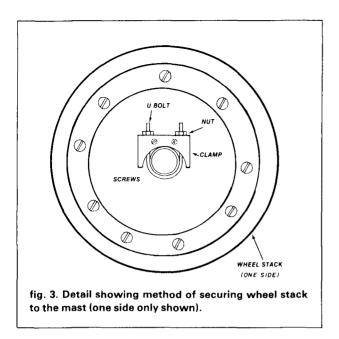
wheel-like device, which will allow you to rotate the antenna mast by means of a nylon rope and your arm muscles. Before you position either the thrust bearing or the pipe brackets with their supports, consider the radius of this wheel, keeping in mind the pole as the axis of the wheel. The wheel must be able to turn without scraping the side of your house. **Fig. 2** shows a suggested mounting scheme.
