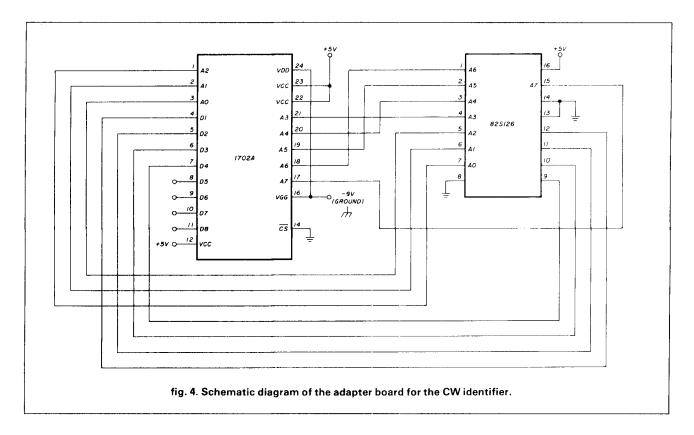
Using wire wrap wire and tools, connect the pins as indicated in **table 2**. (See also the schematic, **fig. 4**.)
