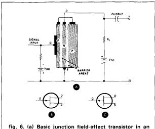
fig, 6. (a) Basic junction field-effect transistor in an amplifier circuit. (b) Symbol for an N-channel JFET. (c) Symbol for a P-channel JFET.
