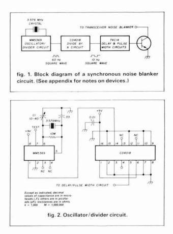
broadened by the narrow selectivity stages. The circuit is designed to be connected into transceiver noise blankers of the type that operate by reverse biasing diodes in a series gate. The circuit should operate without changes on the TS-520, TS-820 and earlier models on the ICOM 701, and any rigs using similar blanker circuits, with minimal modifications to the rig. It has been used to good effect on my ICOM 701 for several months.
