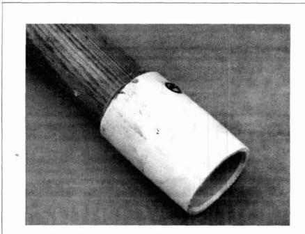
fig. 4. Wood boom has PVC plastic pipe union driven on it and screwed in position. The plug of the cross-arm support slips into open end of the union. Boom is coated with varnish after completion to prevent the wood from warping.
