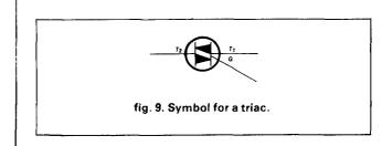
cations discussed here these devices act as solidstate ac relays. They have other uses, such as phase controlling and light dimming circuits, for example.
