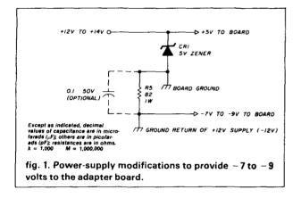
*never* be connected to the ground on the PC board! To do so will short out R5, disabling the -7 to -9 volt supply and almost certainly destroying CR1.
