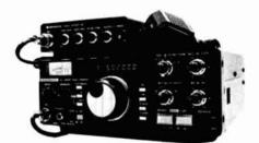
The rf output power is 10 watts on SSB, CW, and fm, and 4 watts on a-m. The Quad Bander operates on 13.8 Vdc drawing 1 ampere in receive, 4 amperes in transmit. Additional information may be obtained by contacting Trio-Kenwood Communications, P.O. Box 7065, Compton, California 90224.
