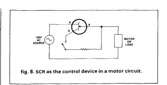
verse biased, preventing any current from flowing in the motor or load. When the switch is closed, one of the junctions that would normally be reverse biased is now forward biased and current can flow through the SCR, turning the motor. With an SCR, however, only current in one direction will be flowing through the load because of the one-way rectifying action.
