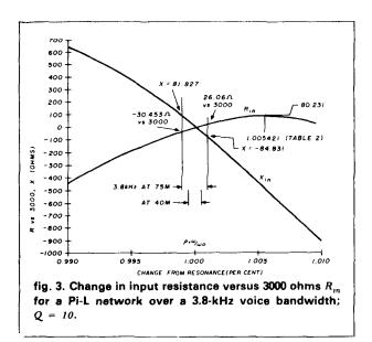
fact that  $R_{in}$  peaks (in this case) about 20.6 kHz higher than the design frequency. This approximate 2 percent change in resistance presented to the final amplifier tube over the voice bandwidth no doubt contributes something to distortion, although it is probably negligible. In any event, using a lower design Q will certainly correct whatever problem may exist.
