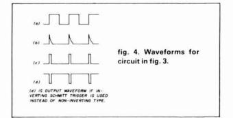
before the square wave goes down again. Again, the diode cuts off the negative part of the wave. The waveforms are shown in **fig. 4**.
