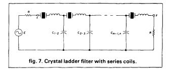
values as for the simple **fig. 3** configuration but would use a resistance slightly lower than the calculated terminating resistance. The latter variation should compensate somewhat for the loss in the chokes.
