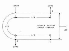
fig. 2. Power divider schematic. The double sliding short provides controlled shunt susceptances to obtain unity input admittance and thus a matched load to the input at all levels of power division.
