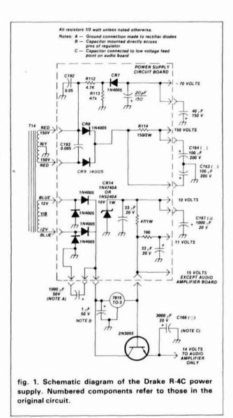
A problem yet unresolved is the presence of excessive hum in the audio output. As pointed out by Sartori,<sup>3</sup> the original Drake power supply also generates significant heat under the R-4C chassis. In that article, Sartori described modifications to the power supply, but the suggested circuit produces marginal voltage for proper operation of the recommended monolithic voltage regulator. In addition, the circuit yields a regulated low voltage 2 volts lower than the original 14-15 volts.
