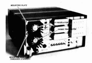
Rear apron of the Drake R-4C receiver showing the voltage regulator and pass transistor, heat sinks, and homebrew mounting plate.
