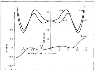
fig. 5. Response of a four-section tandem line, matching 300 to 50 ohms. Each line is nominally one-quarter wavelength long at  $\rho = 1$  for  $Z_{\rho} \approx 240$  and 258 ohms.
