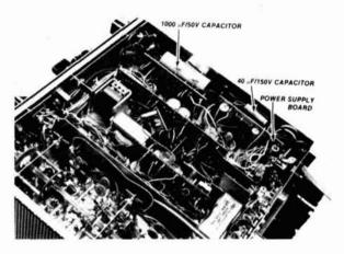
Underside of the Drake R-4C receiver chassis showing revised power-supply board and component layout.
