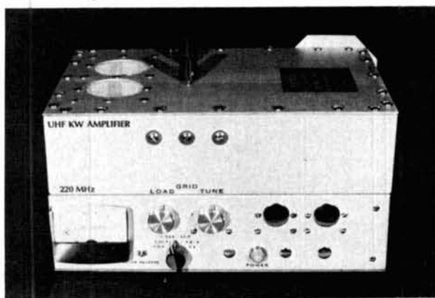
Front and rear views of the 220-MHz stripline kilowatt amplifier, which is enclosed in two mated chassis. Two optional designs are available, one for triode and one for tetrode tubes.
