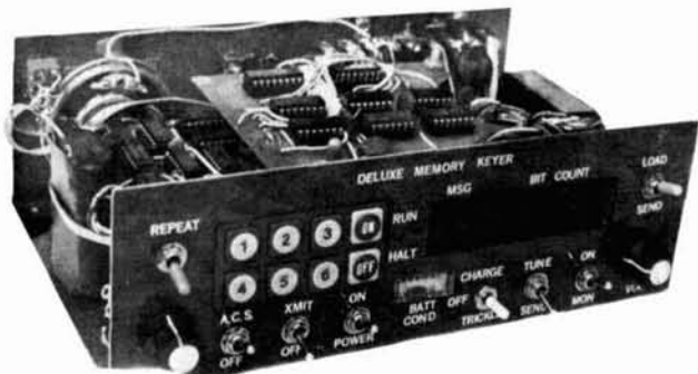
View of the speed adapter board mounted on top of the driver board. The existing keyer memory board is under the driver board. The bit count, WPM mode switch is mounted in the upper left corner, rear, next to the speaker. (Photo courtesy of Bill Mansfield, W1MLT.)
