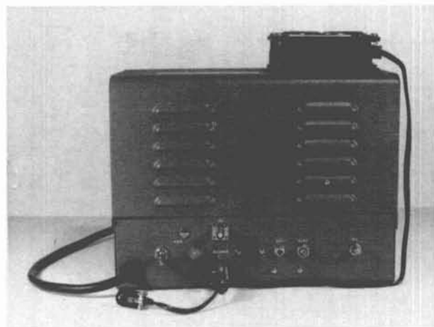
Front view of the power supply for the stripline amplifier with cover installed.
