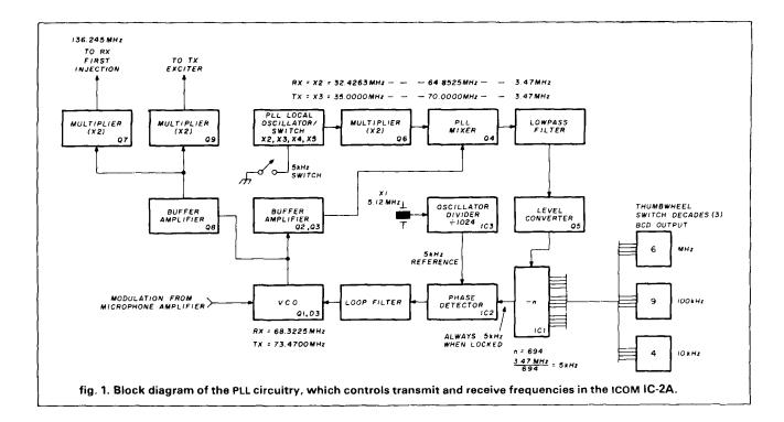
rive the standard offsets from fixed thumbwheel switches without the added expense of CMOS adder circuits, since only two offsets are necessary. However, if an extra odd offset or two are needed, adding more crystals with their associated components is not the answer. Aside from being impractical, it is unnecessary since all that is required is to change the inputs of IC1 appropriately each time you want the VCO to change frequency.
