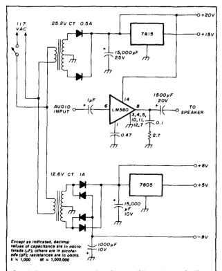
fig. 4. Power-supply and audio-amplifier schematic diagram. This module is built into a separate box away from the receiver circuits to isolate the largest source of heat and to prevent frequency instability.
