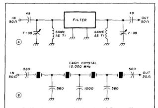
fig. 5. Matching networks for the i-f filters. The network for the monolithic filters is shown at A. Values of components are determined by the filters used (see text). The 500-Hz CW filter, B, is made from four fundamental-mode crystals, which are calibrated for seriesmode operation and have a series resistance of less than 30 ohms.
