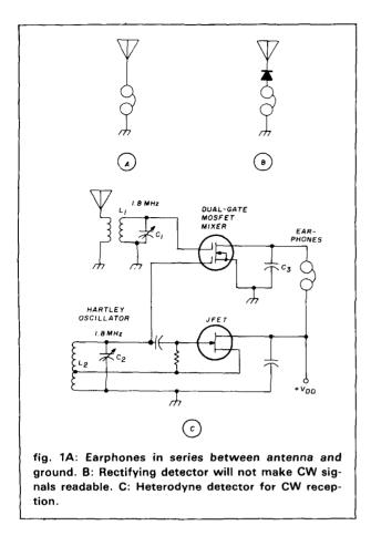
hear it if they did. The earphones (or a loudspeaker) will need an ac of a frequency less than 20 kHz or a dc that is varying at a rate of less than 20 kHz for them to produce a sound wave that we can hear.
