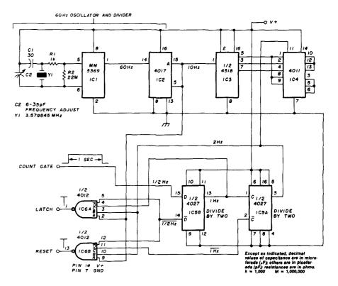
fig. 1. CMOS frequency-counter timing circuit inspired by a previous article in ham radio<sup>1</sup> using TTL devices.
