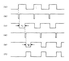
The timing diagram (**fig. 6**) is confusing, however, in that it depicts waveforms (b) and (d) occurring prior to the signals from which they are derived, waveforms (a) and (c), respectively. I am enclosing a corrected timing diagram. It's really a minor error.
