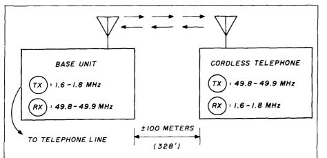
fig. 1. Typical "cordless telephone," model CP-911, marketed by Wenping International under the "Silware" brand name. A U.S. buyer is now applying for FCC approval of this system. Wenping hopes to introduce an improved model with a guaranteed range of 3280 feet (1000 meters).
