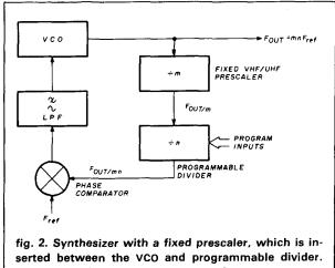
serted between the VCO and programmable divider. Prescaler reduces the VCO output frequency to one that the divider can accept.
