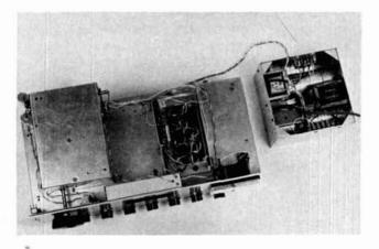
Top view of the receiver. The large box to the left is the VFO assembly, while the smaller box with cover removed is the synthesizer. Power supply is at far right.
