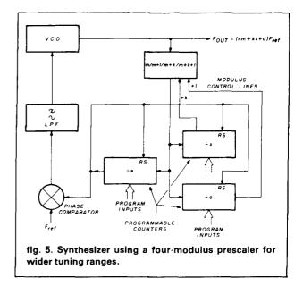
synthesizers. For example, with 25-kHz channel spacing and a 40/41 prescaler, the minimum division ratio is  $40^2 = 1600$  and thus the minimum frequency is 40 MHz. Generally the programmable counter sets limits that are higher than these theoretical minima.
