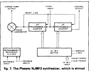
identical to the NJ8811 but is designed to be used with the SP8793 as its prescaler in low-power applications up to 200 MHz.
