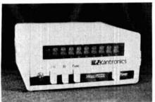
The Micro-RTTY receives any shift of RTTY and displays the message on a ten-character, 3/8-inch high, vacuum-tube fluorescent display.
