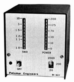
The frequency range of the M-827 SWR meter is 1-30 MHz. Power ranges are 20, 200, and 2000 watts. The SWR scale is 1 to 10 with a logarithmic response that gives much improved resolution where you need it. The M-827 is a compact 4  $\times$  4  $\times$  5 inches with a brushed aluminum control panel, baton switches, and a black vinyl cover. The light bars are 2 inches long with a bright red display.
