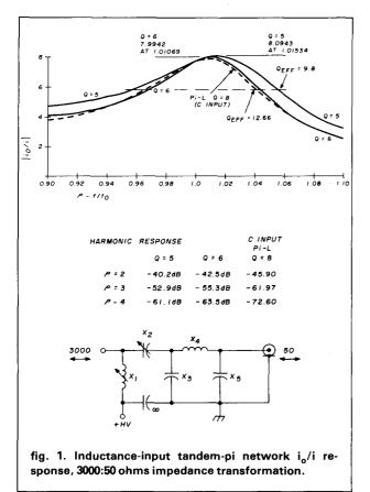
second-harmonic attenuation of this network is only 32.9 dB — slightly less than the conventional pi. Compared with the shunt-capacitance pi-L, it is really disappointing: 32.9 dB versus 47.3 dB.
