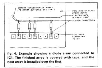
Next insert silicon diodes, such as 1N4148s, cathode-side down into the holes left by the pins. Solder the diodes as close to the board as possible. Next, thread the anode leads into the flex cable holes that will be over each diode when the cable is properly reinstalled. Each diode takes the place of one of the removed pins. Push the cable end firmly over IC1 and solder the leads after making sure that none are crossed. Bridge both gaps on the cable traces with solder.
