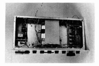
Underneath the receiver. The box in the center with the cover attached is the second mixer. The front-end module is to the far left and the i-f amplifier is at the far right (covers removed).
