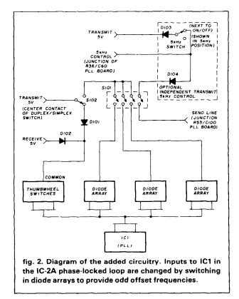
the 5-kHz digit on transmit, leaving the original switch to control 5 kHz in receive if the transmit and receive frequencies differ in the kilohertz digit, since the smallest step the PLL can synthesize is 10 kHz without a change in the PLL local-oscillator frequency.
