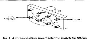
fig. 4. A three-position speed-selector switch for S8 can be made from a miniature double-pole, three-position slide switch. The switch terminals also provide tie points for R10, R11, and R12.
