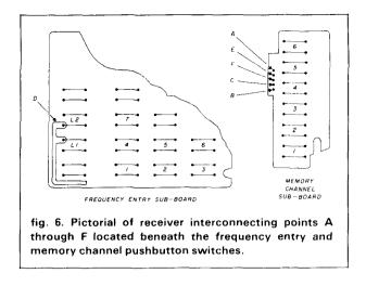
2. Check interface points A through G with the scanner mod powered up to ensure that less than about 0.6 volt dc to ground appears at these points. A high on any one of these points indicates a wiring error, which must be corrected before connecting the mod to the receiver.
