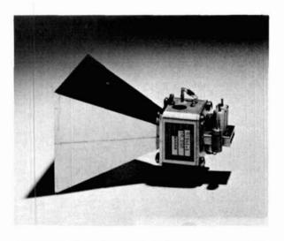
The 10-GHz Gunnplexer features bandwidths in excess of 20 MHz and direct adaptability to multi-unit linking. Transmitting frequencies of communicating units are offset by the amount of the desired i-f.
