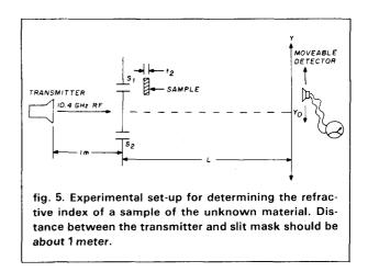
**3B**. The thickness of the sample,  $t_2$ , in this instance proved to be 25 mm, and the observed envelope shift,  $\Delta Y$ , was measured 0.51 meter. This reveals a refractive index,  $\eta_x$ , of 1.593, using **Eq. (6)**. We now know the refractive index at 10.4 GHz of the material.
