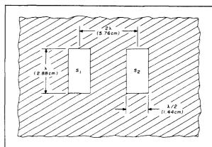
fig. 4. Construction details of the double-slit mask, a device that can be used to determine the refractive index of the material in question. Once the refractive index is known, it is a simple matter to calculate the wall thickness required to make the box appear transparent at 10.4 GHz.
