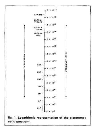
an electromagnetic field. This kind of field has a way of reproducing itself in such a way that, even at great distances, the electrons in a conductor are accelerated in a manner identical to that of the particles in the far-off antenna. Usually, when electromagnetic fields are produced deliberately for communications purposes, a sine-wave current is generated in a piece of wire. This current may have any frequency, from less than 1 Hz to billions of Hz.
