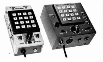
Of two versions of the auto-dialer built by the author, the one on the left was housed in a plastic case and the other in a standard LMB metal box. Both units are used in the author's cars, but only the one on the right has provisions for using the car battery as a supply. The additional connectors are for using the auto-dialer with other rigs.
