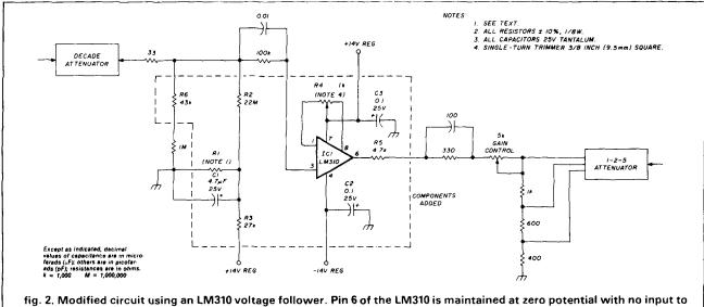
fig. 2. Modified circuit using an LM310 voltage follower. Pin 6 of the LM310 is maintained at zero potential with no input to the oscilloscope.
