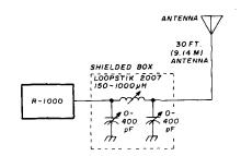
fig. 1. Lowpass filter for the R-1000.
