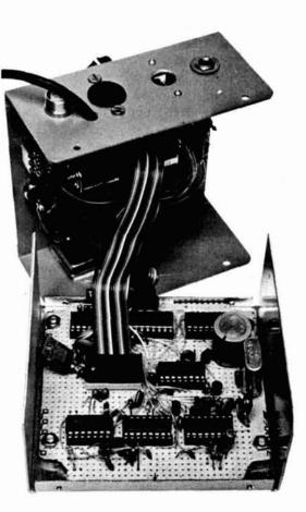
This version of the auto-dialer was built using point-topoint wiring. A ribbon cable and connector connects the two halves of the case together to facilitate servicing. A  $4\frac{1}{2}$ -volt backup battery can be seen in the cover.
