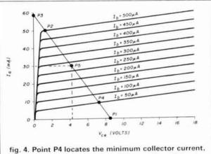
fig. 4. Point P4 locates the minimum collector current,  $I_e$ , under maximum signal conditions. Point P5 locates expected idling current under no-signal conditions.
