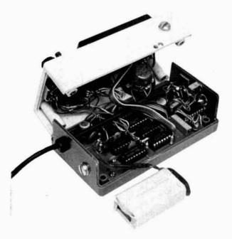
The auto-dialer in this plastic case uses an earlier version PC board that is a hair narrower than the board shown in *fig. 3.* The battery fits right on top of the ICs. Note the 1-inch speaker in the upper right corner of the cover.
