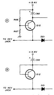
fig. 1. Original break-in delay circuit of the Heath HW-8, A. The improved circuit, B, eliminates choppy-sounding CW at higher keying speeds.
