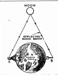
This represents a suggested method of sending a radio wave to the moon and back; to determine by the reception of the reflected wave the permeability of the Heaviside layer. It was proposed in RADIO NEWS for February, 1929, by H. Gernsback, the editor.
