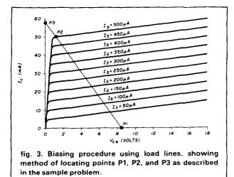
examination reveals that the collector current,  $I_c$ , is being plotted against the collector-emitter voltage,  $V_{ce}$ , at various base currents,  $I_b$ . Actual common emitter characteristics vary from transistor to transistor of the same type and exhibit a marked shift with temperature; thus they are approximate.
