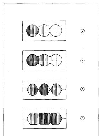
fig. 1. What you see on your CRT screen: A, a perfect string of dots as they might be seen under ideal conditions; B, the apparent running together of dots caused by lack of definition in the human eye; C, the effects of turn-on and turn-off times in the video amplifiers, display tube, gun, and even in the phosphor itself; D, the combined effects of B and C.
