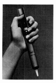
vacuum that instantly removes molten solder. Double O-ring piston-seals achieve maximum vacuum in a piston stroke of less than two inches. The piston is set with the thumb and released by pushbutton for maximum spring force. The worker's other hand is left free to hold the soldering iron that melts the solder.
