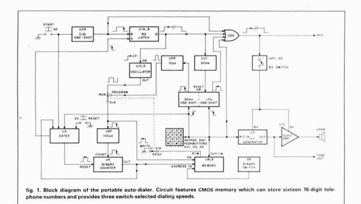
use. Three switch-selected dialing speeds are provided: 55 milliseconds per digit for state-of-the-art patches, 250 milliseconds per digit for slower patches, and 1 second per digit for those machines that use tone-to-rotary-pulse converters. To ensure full capture of the repeater, dialing tones are output 300 milliseconds after the dialer keys the transmitter PTT line.
