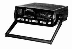
In addition to EIA CTCSS tones, the test unit works with digital codes compatible with Digital Private Line, Digital Channel Guard, Digital Quiet Channel, Digital Call Guard, etc. Used in conjunction with a monitor receiver, the test unit may be used to police shared repeaters, select unused codes and identify unknown codes right off the air.
