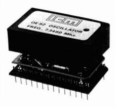
Specifications: input voltage – +5 Vdc; temperature stability – -30 to +60 degrees C; OE-52 –  $\pm$  0.0002 percent; OE-53 –  $\pm$  0.0005 percent; output voltage – 5.5V PP, 2.9V RMS; trim range –  $\pm$  10 ppm minimum; size – 0.430 × 1.45 × 0.795 inches.
