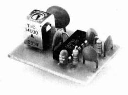
fig. 5. The fm demodulator board.
