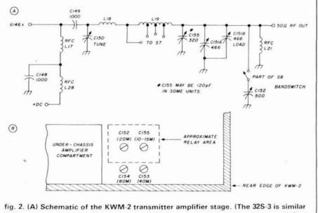
hig. 2. (A) Schematic of the KWM-2 transmitter amplifier stage. (The 325-3 is similar but component nomenclature may be different, as well as parts placement.) The capacitors to be readjusted for 10-MHz operation are C-152 and C-155, mica compression units mounted on the chassis deck. (B) Under-chassis view of KWM-2 showing placement of compression capacitors near amplifier compartment and rear edge of chassis. Capacitors may be adjusted from above or below the chassis.
