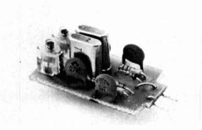
fig. 2. PC board making use of diode switching.
