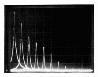
A multiple-exposure photograph showing the analyzer's good frequency and amplitude linearity. Amplitude steps are in 5-dB increments and frequency steps in 5-kHz increments across the screen. Greater than 40 dB of range is displayed here.
