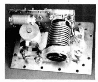
An example of a cylinder-tuned VFO.
