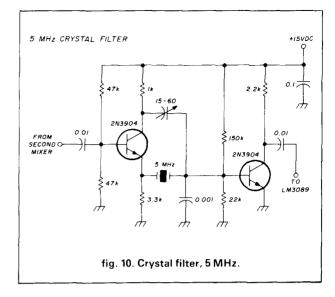
voltage-tuned first LO at 32 MHz, filter the image and amplify at a first i-f of 41 MHz, then beat this down to 5 MHz with the second LO at 36 MHz. Here just the second LO filter, the 36 MHz bandpass filter, and a few tuned circuits in the oscillators need be scaled accordingly.
