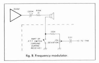
modulation transformer T110 and RV102 are discarded. The B + is restored to the final amplifier by joining points 18 and 20 on the Cybernet board. The output of the audio amplifier, IC 102, is routed from the positive side of C204 through R194 to the hot side of the speaker. The cold side of the speaker is grounded during receive through one of the contacts of the PTT switch.
