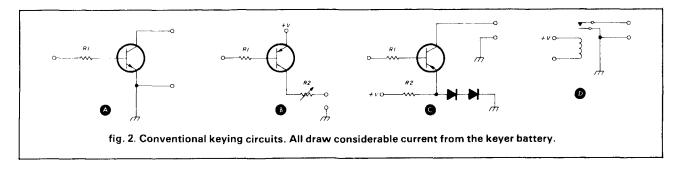
transistor turns on fully (saturates) with whatever collector current the transmitter presents in a keydown condition. This requires an additional 1 to 10 mA of current from the keyer battery.
