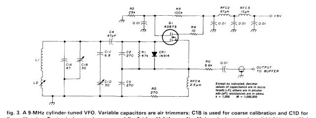
fig. 3. A 9-MHz cylinder-tuned VFO. Variable capacitors are air trimmers; C1B is used for coarse calibration and C1D for fine calibration. Tuning is done in the manner of *fig.* 2. L1 = 11-1/4 turns No. 16 tinned wire on a glass vial 1.04 inches (26.4 mm) in diameter and 1-1/4 inches (28.6 mm) long. L2 = 3-3/4 turns No. 16 enameled wire, close wound, 7/8 inch (19.4 mm) in diameter.
