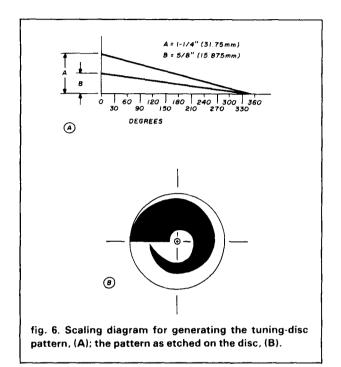
pattern as transposed to the disc in **fig. 6B** is centered toward the outside of the disc, since the center of the pattern must rotate past the center axis of the coil, and the coil must be positioned so that one edge must clear the shaft and its support bearing. Refer to **fig. 8** for details.
