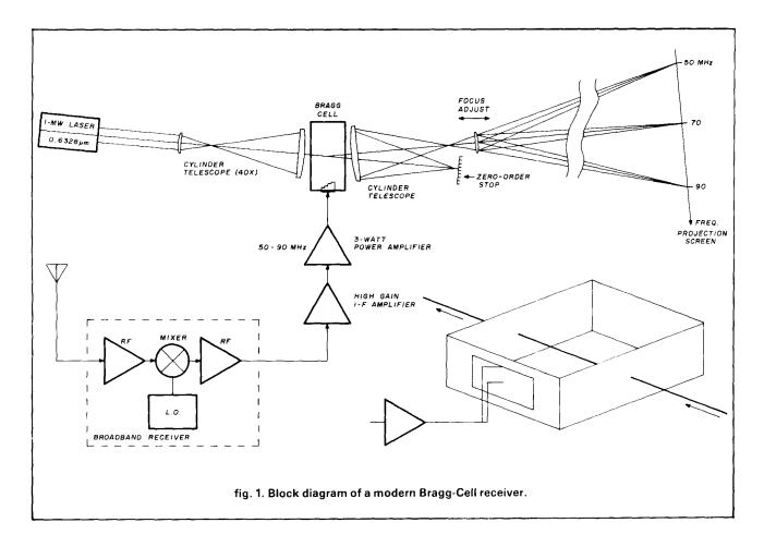
received signals. Post-detection demodulation can be accomplished by an array of closely spaced PIN photodiodes. The position of each photodiode corresponds to a specific frequency within the passband of the receiver's input, providing instantaneous reception of many signals, without sweeping or scanning.
