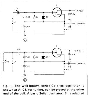
shown at A. C1, for tuning, can be placed at the other end of the coil. A basic Seiler oscillator, B, is adapted from the series-Colpitts. C1 is now a coupling capacitor and C4 is generally used for tuning. If L1 is tuned, C4 can be used for frequency calibration.
