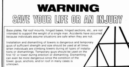
The dismantling of some towers should be done with the use of a crane in order to minimize the possibility of member, guy wire, anchor, or base failures. Used towers in many cases are not as inexpensive as you may think if you are injured or killed
