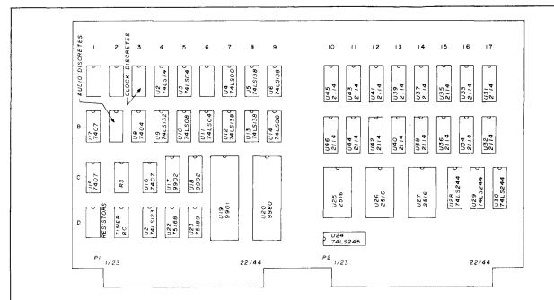
fig. 7. Location of ICs on controller board. Edge connections are double side, and pins etched in board. Letters and numbers used for construction reference. Two RAM chips in U31, U32 is the minimum requirement but photo indicates 4K RAM population up to U38 for development purposes.
