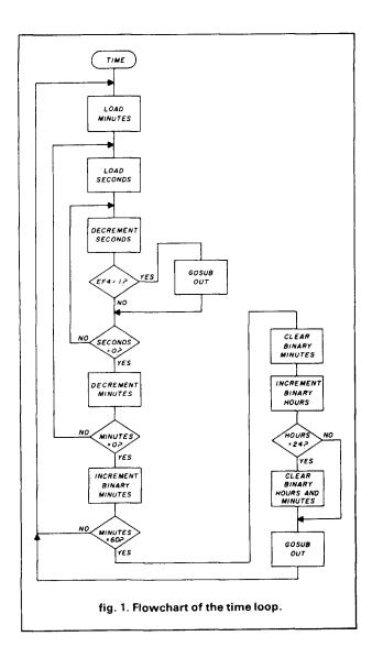
jumps to the BCD subroutine (**fig. 3**). Now that the program has the time in BCD, control passes to R5 for the Code routine, which converts the BCD digits into Morse characters. On return, program control reverts to R0 to resume the time loop.
