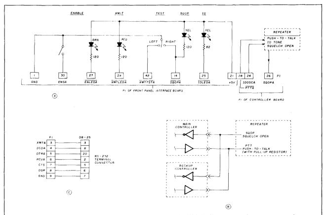
fig. 6. Front panel controls and indicators for 2-meter repeater in A. 220 MHz front panel and repeater connections are identical except for pin numbers. Underlined names are identical to front panel photo. B indicates parallel connection scheme for backup controller. C gives RS-232 serial interface pin connections to main controller.
