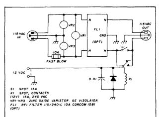
fig. 6. Primary power-relay schematic diagram. This relay box includes additional transient protection (optional). Switch S1 bypasses the relay if remote switching is not desired.
