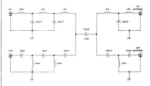
fig. 2. The capacitor changes to the N6RY diplexer mods.
