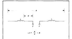
fig. 2. Loaded dipole with loading coils placed one-half the distance from the feedpoint (F-F) to the end. Distance A is one-quarter wavelength.
