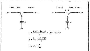
fig. 1. The switched-capacitor principle allows a small capacitor to be used in place of a large resistor. This has allowed the manufacturer to put filters and decoding circuits on one silicon chip.
