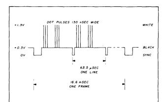
fig. 2. Typical video text display format. The actual picture is about 1.0 volt peak-to-peak with sync pulses 0.2 to 0.3 volt below black. The whole signal is usually positive, as shown. (Levels measured across 75 ohms.)
