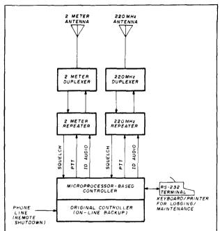
fig. 1. Overall system block diagram of the K50JI double-frequency VHF repeater. New controller includes a keyboard/printer terminal for logging and maintenance. Original controller on-line for backup. Telephone remote shutdown disables entire system.
