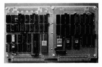
photo 2. Photo of controller board made just before final circuit freeze. All ICs are socketed on prototype board. Except for supply bypass capacitors, all discrete components mounted on DIP plugs. Number labels were construction references.
