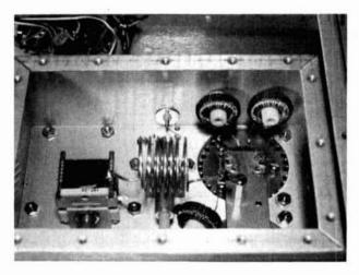
Bottom view of cathode box of triode amplifier.
