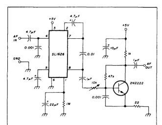
fig. 5. AGC amplifier schematic diagram. This circuit maintains a constant audio level to the phone patch.
