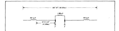
fig. 7. Compact, coil-loaded dipole for 3.80 MHz. Tip length is adjusted for minimum SWR at design frequency. Coil is wound with No. 16 (M1.3) wire per data in fig. 5.
