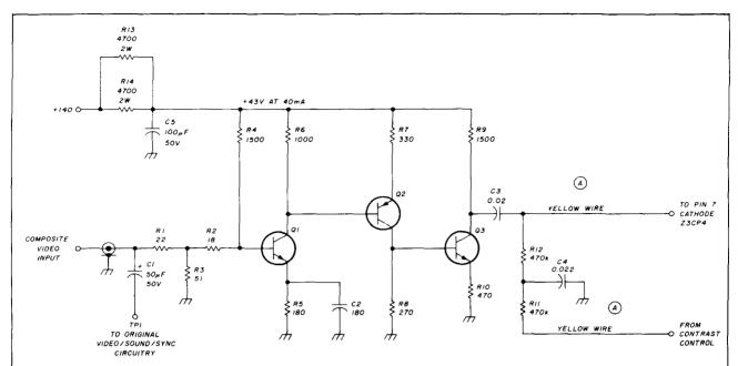
fig. 4. New broadband video amplifier for use with tube-type TV sets. For external connections refer to fig. 1. The cathode lead is cut at point A, and the amplifier is inserted as indicated. Q1, Q3 are 2N2222A and Q2 is a 2N3905.
