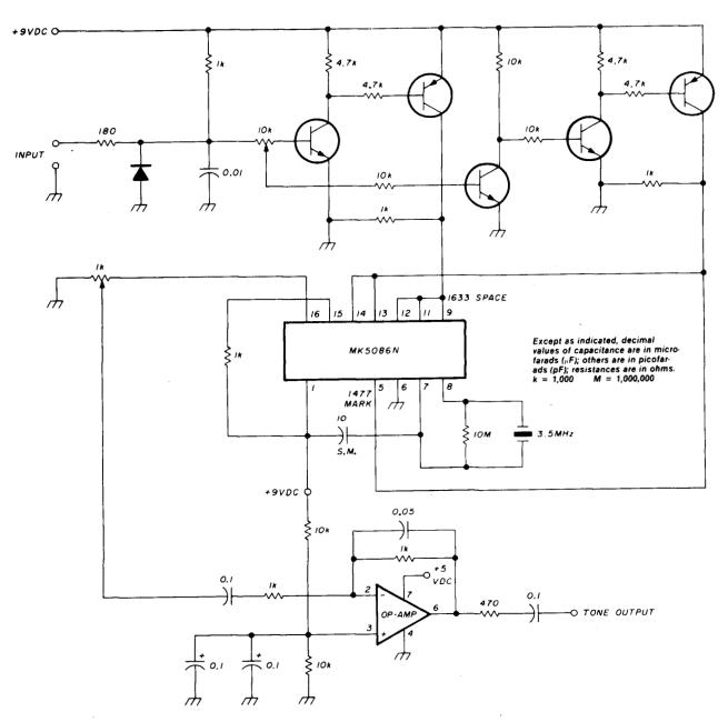
fig. 1. Schematic for the FSK tone generator.
