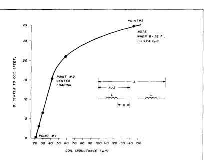
fig. 3. Inductance increases as the coil moves outward from the center of the loaded element. The increase in inductance is linear until coil reaches the center point of the element, and then it increases rapidly approaching the tip. If the coil is placed at the tip, inductance would theoretically have to be infinite. Coil loss increases with inductance, and point 2 on curve represents a practical compromise. Point 1 is for base loading.
