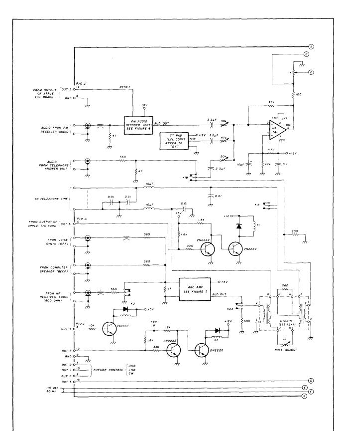
fig. 4. The interface-control schematic diagram. Note that the AGC amplifier and optional fm audio decoder schematic are shown separately.
