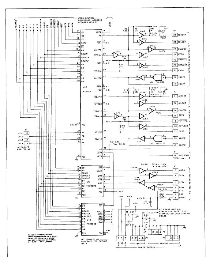
fig. 5. Interface circuitry and power supply connections. UART in U18 used mainly for internal timer. RC filter for CW ID tone (IDOSC) should be isolated to minimize digital noise. A minimum of one 0.01  $\mu$ F bypass per three ICs is recommended on entire board.
