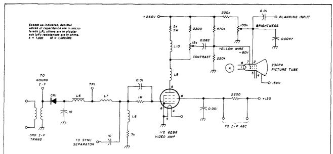
fig. 1. Partial schematic of black and white TV set showing video amplifier and picture tube connections. CR1 is a 1N60, 1N395, etc. L7-L10 are video peaking coils. Points TP1 and A are referred to elsewhere.
