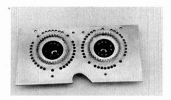
Triode amplifier socket plate assembly - top view.
