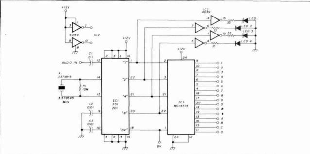
fig. 3. Schematic diagram of the author's completed decoder circuit. The CMOS signals are all 12-volt levels, so a converter is needed if the decoder must drive TTL.
