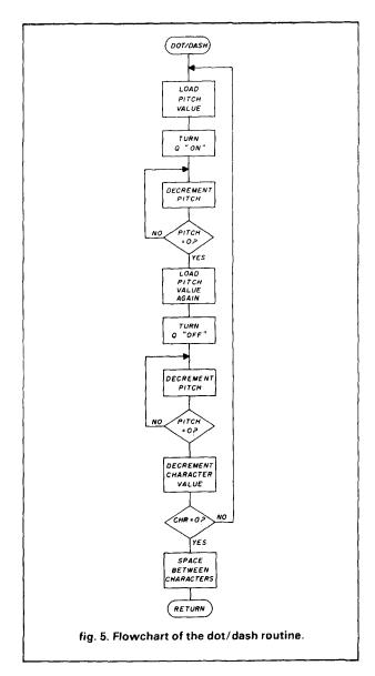
00B7 and 00BE. You can alter the speed of the Morse characters by changing the values for dot, dash, and space at locations 00A9, 00AE, and 00C9. Finally, if you prefer a twelve-hour format, change the value at location 0049 to 0C.
