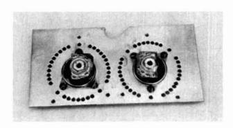
Triode amplifier socket plate assembly - bottom view.
