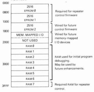
fig. 4A. Memory map of controller. Monitor ROM located in \$0000 to \$07FF address. Minimum RAM in address location \$3D00 to \$3FFF (\$ = hexidecimal).
