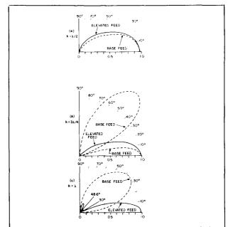
fig. 3. Vertical radiation patterns for base-fed and elevated-feed monopoles.<sup>3</sup>
