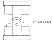
fig. 1C. Join the two capacitors as indicated.
