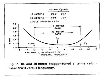
spacing of 7 percent. However, as the minimum is further reduced, the outside edge SWR begins to increase. A choice of 6 percent relative dipole stagger for both the 10- and 40-meter bands appears to be a reasonable compromise.
