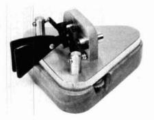
There are no power cords to clutter up the operating desk. Power comes from a self-contained 7.5-volt battery. The EK-1 is limited in that it does not have a memory like so many of the newer electronic keys. But not everyone feels that this is necessary and many will find the EK-1 a nice, simple package.
