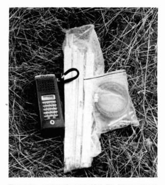
The station, ready to be assembled. The longer antenna parts are in a plastic bag. The smaller pieces and a length of coaxial cable are in the smaller pouch. (Photo courtesy N6ST.)
