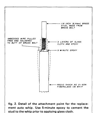
joint, wind each strip in overlapping fashion, like tape, to cover the joint and 1/2 to 3/4 inch of the bolt. Three layers of cloth will provide ample strength. Be sure to follow all instructions provided with the kit, including the safety precautions.
