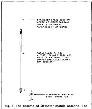
capacitor may be attached with spring clips for improved matching (see text).
