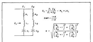
fig. 4. Equivalent circuit of two stagger-tuned crossed dipoles and SWR equation.
