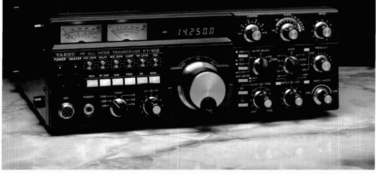
The FT-102 is factory equipped for operation on all present and proposed Amateur HF bands. An extra AUX band position is available for special applications. Equipped for SSB, CW, and AM (RX), the FT-102 may be activated on FM and AM (TX) via the optional AM/FM-102 Module.
