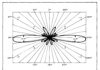
fig. 8. A 15-degree progressive phase delay (with the top dipole having the shortest delay line) produces the indicated beam tilt. The main radiation is depressed nearly 3 degrees from vertical while the half-power beamwidth remains near 13 degrees. The array is centered on the 0 to 180 degree axis with the top dipole in the 0 degree direction.
