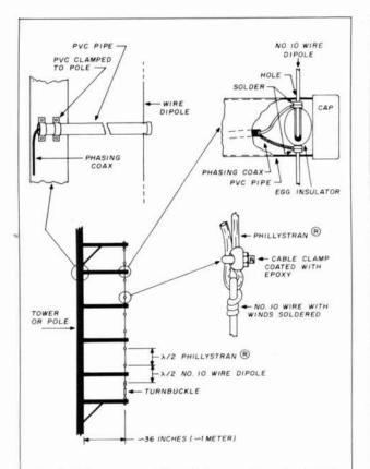
fig. 9. This suggested Four Pole array (constructed of cable with high tensile strength) may solve the tough environmental problems encountered on mountain tops. PVC pipe is used to protect horizontal feed cable runs from ice build-up.
