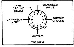
Figure 1. Pin Connections
