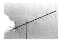
S/N ratios. Benefits of circular polarity on transmit are similar, regardless of the polarization of the receiving antenna.
