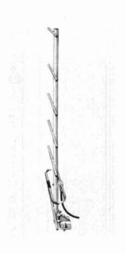
highway mobile radio systems. Reflector and director elements are 3/8-inch diameter aluminum rods welded to the boom, reducing the risk of damage and misalignment. The antenna clamp allows easy orientation for either vertical or horizontal polarization. A higher gain can be achieved by using dual (SRL-307-2) or quad (SRL-307-4) arrays with gains of 12.5 dBd and 15 dBd respectively.
