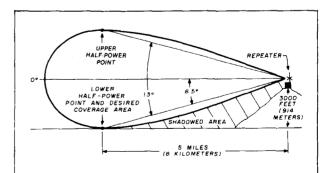
fig. 2. A repeater antenna with a vertical, 13 degree, half-power beamwidth barely meets the required depression angle. Any station closer to the repeater is shadowed while the repeater power in the pattern above 0 degrees is wasted.
