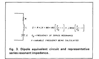
The equation for the impedance of a dipole given in this figure curvature has been derived by fitting to dipole impedance curves.<sup>3</sup>
