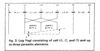
$l_2 - l_3$  spacing multiply the  $l_1 - l_2$  spacing by  $\tau$ .
