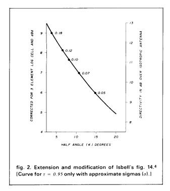
enable the designer to reasonably determine cell gain. One represents the  $\tau$  versus  $\sigma$  from K4EWG's work<sup>1,2,3</sup> and the other is from Isbell's<sup>4</sup> work using  $\tau$  versus half angles. The Isbell curve has been modified by extending the curves to include half angles near 3 degrees.
