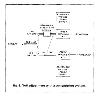
antenna spacing, feedline length, or both. Another method is to maintain the 180-degree null point and to aim the back of the array toward the undesired signal.
