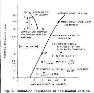
antennas from 3 to 90 degrees. Theoretically derived and modified to fit measured resistances ( $\Delta r$  less than 1 ohm at  $\theta = 50$  degrees).
