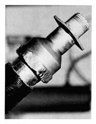
fig. 6. The finished connector installed on the line. It is ready to be protected from the elements and placed in service.
