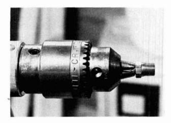
fig. 2. The Barb fitting prior to machining.
