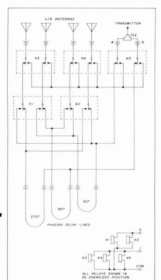
fig. 4. Relay inconnection diagram for the four-element phased array. The preferred end-fire direction is present with no dc applied. Voltage applied to terminals 2 and *COM* reverses the array (still end-fire), while dc applied to terminals 1 and *COM* provides a bi-directional broadside lobe pattern.
