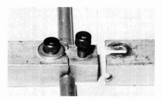
Close-up of the joint between the first director and the boom. The boom is made from lengths of aluminum anglestock which are fastened to the block by screws. The element halves screw into the sides of the same block.
