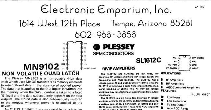
An OUTPUT ENABLE is also available, which when taken to logic '0' level presents a high impedance state on each data output line, permitting multiplexed operation.
