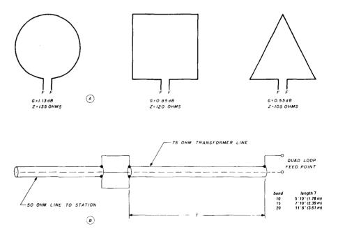
fig. 1. (A) The simple transmitting loop. Directivity is in and out of page. The triangular loop may be inverted, with apex at bottom and feedpoint at apex. (B) Quarterwave transformer for use with quad loop antennas.
