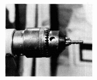
fig. 3. The Barb fitting after one end has been machined. The ribbed end is about to be machined.
