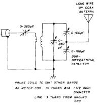
fig. 1A. Antenna tuner schematic.
