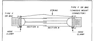
fig. 3. Adjustable-length coaxial line section using brass tubing with each half approximating impedance of associated cable.
