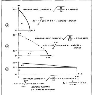
fig. 1. Current distributions for three referenced antennas, each over perfect ground, and 36 watts input to antenna terminals. All to scale, so areas are directly comparable. (A) Current distribution of  $\lambda/4$  vertical (reference antenna) against a perfect ground, (B) Current distribution of  $\lambda/16$  (23 degree) top-loaded vertical against perfect ground, (C) Current distribution of  $\lambda/16$  (23 degree) base-loaded vertical against perfect ground.
