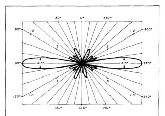
fig. 4. The vertical radiation pattern of a Four Pole antenna produces a half-power beamwidth of approximately 13 degrees. (Half-power points are synonymous with a 0.707 normalized field voltage.) The line of the Four Pole array is centered along the 0 to 180 degree axis with the top dipole in the 0 degree direction.
