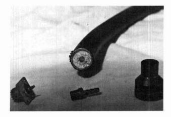
fig. 1. The 1-inch hardline, coax connector, and the plumbing fittings used to make a connector for the hardline.
