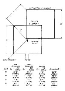
fig. 4. Design data for two-element quad. Dimension R is approximate distance from center point of loop assembly to point of attachment of wire.
