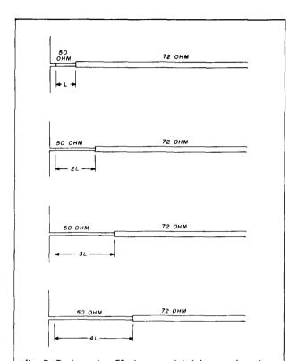
fig. 5. By inserting 50-ohm coaxial delay sections between the dipole feed points and the 72-ohm feed sections, a progressive phase shift is introduced. Selection of the proper phase shift causes the antenna pattern to electrically tilt downward.
