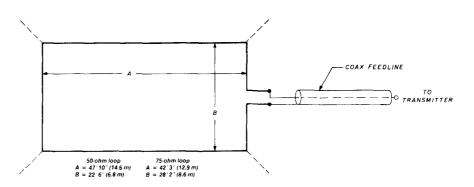
fig. 3. Vertically polarized 40-meter loop for 50- or 75-ohm feed. Mount loop in vertical plane as high above ground as possible. Bring feedline off horizontally.
