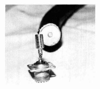
fig. 4. The inner assembly has been completed and prepared for insertion into the outer adapter.
