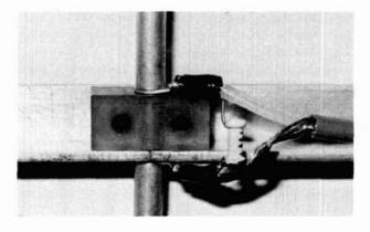
Close-up of the driven element and matching circuit. The mechanics are the same as Photo 2 except that the block is acrylic plastic and the coax cable is connected to the two sides of the driven element. The tubular capacitor is used for impedance matching.
