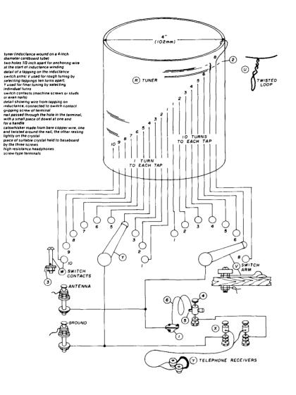
fig. 2. Construction details of the U.S. Bureau of Standards crystal radio receiver (1920).
