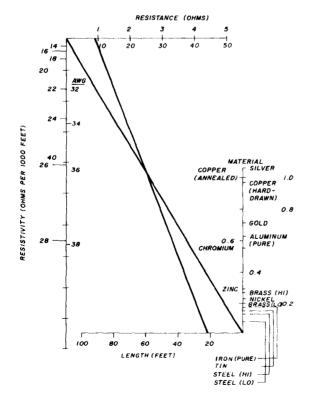
fig. 1. Nomograph for designing custom resistors.
