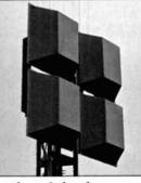
Phased dipole array 740/225-400 MHz
