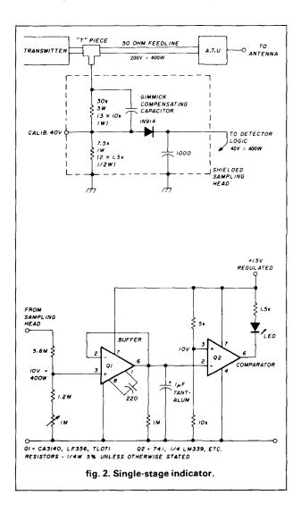
nominal ratio of 4:1 so that when it's adjusted, the original 200 volts on the feedline is now reduced to 10 volts. Since the output from the sampling head after rectification is audio with frequency components up to only 3 kHz, no compensation of the secondary divider is necessary.
