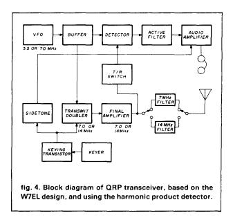
transistor, however, now becomes a doubler. There remains enough drive for the desired input of 2 watts to the final, for output on 40 or 20 meters of about 1 watt.
