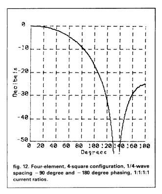
placement of -135 degrees. A number of representative arrays have been plotted to show their general properties and to illustrate the variations that occur with changes in physical layout or varying input drive conditions.
