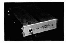
The amplifier operates on 13.8 Vdc and draws approximately 4 amps maximum during transmit. It utilizes carrier operated switching (COX) with no delay and has SO-239 connectors. The HL-30V measures approximately 4  $\times$  6  $\times$  1 inches (100  $\times$  158  $\times$  30 mm) and weighs 520 grams. Suggested retail for the HL-30V is \$69.95.
