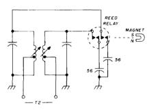
fig. 1. Magnet pulls in additional 56-pF capacitors, lowering the Triton IV bandpass filter to 10 MHz.
