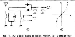
fig. 1. (A) Basic back-to-back mixer. (B) Voltage-current characteristics of the back-to-back matched diodes. porated two bands, a keyer, and two 0.9-AH rechargeable batteries all in a 4  $\times$  6  $\times$  2-inch (10.16  $\times$ 15.24  $\times$  5.08 cm) box. Naturally, the smaller the rig the worse the problem, because of the proximity of components and wiring.
