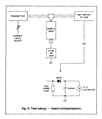
the 29.5-MHz reading, there is insufficient capacitance in the "gimmick" and more twists should be added. If the 29.5-MHz reading is higher than the 3.5-MHz reading, the head has been over-compensated for, and the "gimmick" should be untwisted. The aim is to get the voltmeter readings at both 3.5 and 29.5 MHz to be the same. Note that putting the cover on the sampling head enclosure has a slight effect on the readings and should be allowed for.
