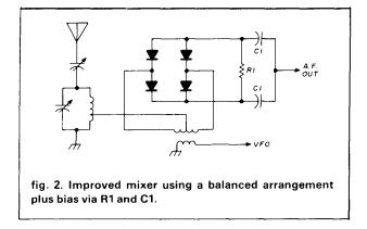
RA3AEE describes the operation of the detector as follows: "When the local oscillator voltage goes through zero, both diodes are open circuit and the circuit current vanishes. At the peaks of both positive and negative half-waves of this voltage, one or the other of the diodes conducts and the signal source is connected to the load. In this way the mixer works like a switch, closing the circuit at a frequency equal to twice that of the local oscillator."
