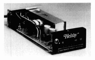
Interior view of a 50-watt model PEP indicator. The assembly slides into an extruded aluminum case. The sampling head is contained in the rectangular housing at the rear. All other components, including the power supply, are mounted on an L-shaped PCB. limit is set on the allowable dc input power to the final amplifying devices — be they valve or solid state. In Australia, the United Kingdom, and many other countries, a limit is set on the allowable peak rf output from a transmitter.
