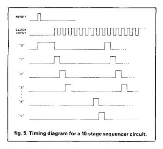
to sequence through a series of code-generating and condition-testing steps. Only the frequency of the clock need be adjusted to vary the code timing. The circuit described here was designed using digital complementary metal-oxide semiconductor (CMOS) integrated circuits to reduce power consumption.
