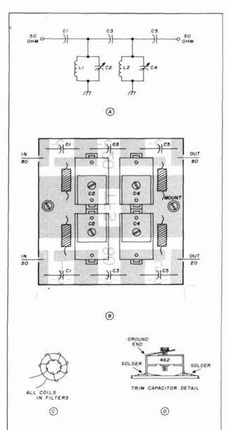
fig. 2. Schematic diagram (A) of the bandpass filters, and parts location (B). All coils are wound on a toroidal core as shown by (C); see table 2 for values. The tabs on trimmer capacitors are bent outward and soldered to the circuit board as in (D). All parts are on foil side of board.
