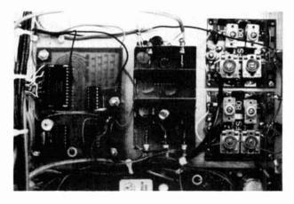
Three of the assembled boards. From left to right they are the digital readout board, the VFO, and the bandpass-filter board for 80 and 20 meters. A shielded control line goes to the VFO.
