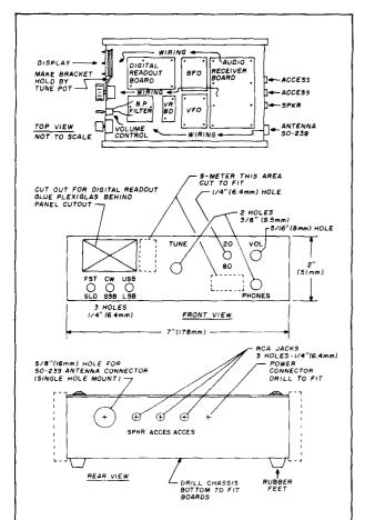
fig. 13. Suggested packaging for the two-band receiver. The enclosure is a standard  $2 \times 7 \times 11$  inch aluminum chassis (Bud AC402) with cover plate. Wood rails are added to the side and stained. The cabinet and panel can be painted to choice. Miniature toggle switches are used, and the volume control is a miniature type with on/off switch.
