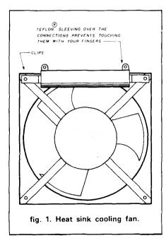
keep it cool. A four-inch resistor will mount on clips attached to the holes in the fan used for mounting (see **fig. 1**).
