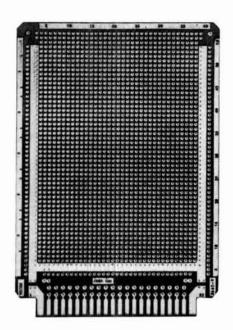
Fabricated of FR-4 (G10) epoxy glass laminate, the pads are 2-ounce copper cladding with bright tin plating for easy soldering. Cardedge connectors are nickel plated and gold flashed to ensure long life and low resistance. Zoned-wiring locations, etched into the cladding, permit easy component identification.
