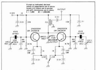
fig. 5. Schematic diagram of the BFO for the receiver. T3 primary is forty-five turns No. 28 enameled wire on T50-2 core; secondary is three turns No. 28 over primary.
