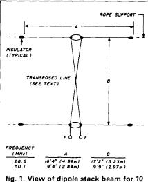
or 6 meters. Directional pattern is into and out of page. Array is fed at F-F with 50 or 75 ohm coaxial line, as discussed in text. Coax connection at F-F should be waterproofed.
