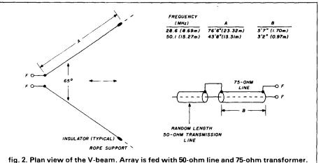
Joint between lines and coax connection at F-F should be waterproofed.
