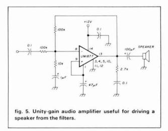
passing the power supply near the chip, and all ground pins on the chip should be used.
