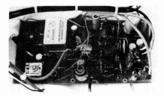
The main receiver board. Note the shielded wiring used on all audio and rf connections. From left to right are the mixer, crystal filter, i-f amplifier, product detector, AGC circuit, audio filter, and audio amplifier.
