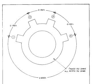
fig. 7. An equal-split hybrid ring can also be formed using 50-ohm transmission line.
