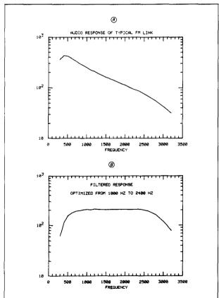
fig. 4A. Measured frequency response using a pair of 2meter FM transceivers, fig. 4B. The same frequency response after filtering. The filter design was optimized for the range 1000 Hz to 2400 Hz.
