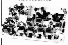
T51 VHF FM EXCITER for 10M, 6M, 2M, 220 MHz or adjacent bands. 2 Watts continuous. Kits only \$59.95
