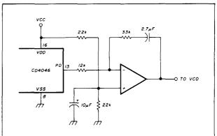
fig. 8. Simple Op-Amp integrator loop filter for example loop.
