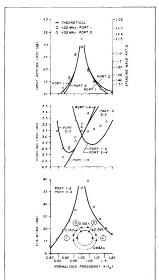
fig. 8. A hybrid ring formed using 50-ohm line microstrip operates over a much smaller bandwidth.
