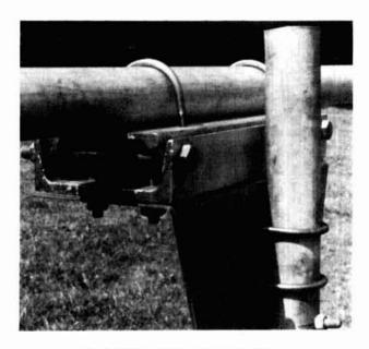
fig. 4. Bolts in place secure the hinge.
