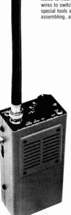
MX 2 (144 MHz band) and MX-6Z (50 MHz band) SSB/CW QRP...
