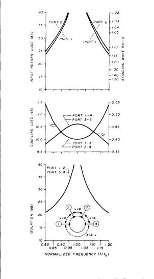
fig. 10. The theoretical response of the 10-dB coupler appears quite good over a 20 percent bandwidth.
