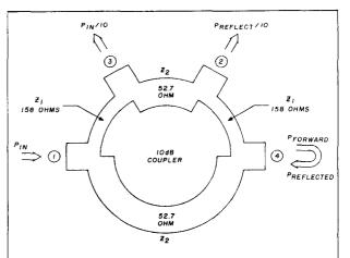
fig. 9. The power division is controlled by adjusting the ring transmission line impedance between ports.
