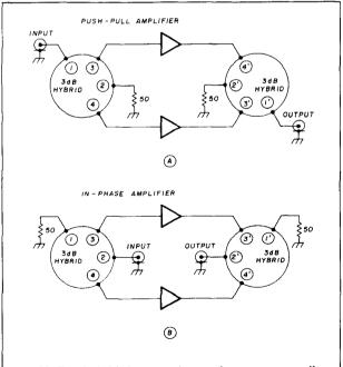
fig. 11. The hybrid ring may be used as a power splitter/combiner for a (A) push-pull amplifier or (B) an inphase amplifier.
