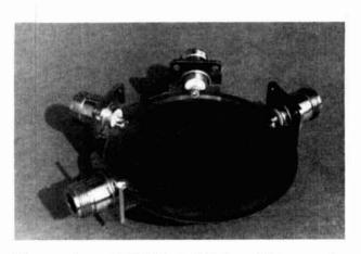
The experimental 1296-MHz hybrid ring with inexpensive type "N" launchers.
