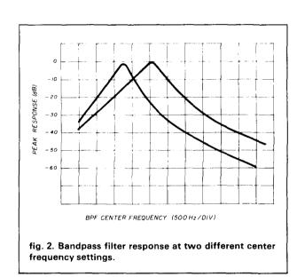
A major advantage of this type of filter is that the notch and bandpass position is determined by the clock frequency. Therefore, by varying potentiometer R2 the notch or bandpass can be moved in position as shown in the spectrum analyzer photographs in figs. 1 and 2. Fig. 1 indicates a notch filter response (notch depth approximately 60 dB) and fig. 2, the bandpass display displaced in two positions. The bandpass filter was adjusted for CW or RTTY operation.
