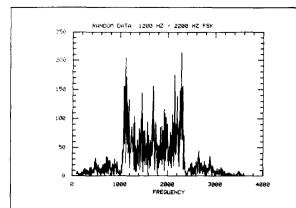
fig. 3. Sound spectrum of a one-second burst of 1200 Hz/2200 Hz 1200 baud random NRZI data. This data was generated and analyzed by computer.
