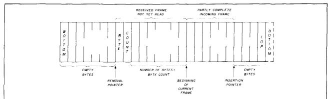
fig. 6. A typical data buffer, showing pointers, and order of placement of data. The buffer shown is the packet input buffer, and is similar to the other buffers.
