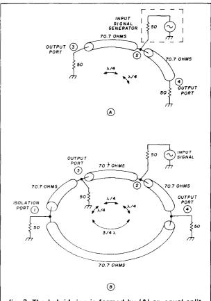
fig. 2. The hybrid ring is formed by (A) an equal split power divider followed by the addition of a cancellation line (B) to provide port-to-port isolation.
