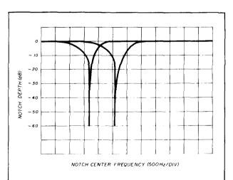
fig. 1. Notch filter response can be translated in frequency by changing the clock rate.
