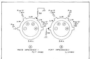
fig. 1. The hybrid ring provides (A) two equal signals 180 degrees out of phase or (B) two in-phase signals.
