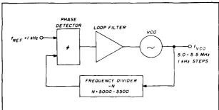
fig. 3. A 5.000-5.500~MHz synthesizer that tunes in 1 kHz increments.
