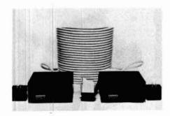
power, and will operate in ambient temperatures of 0 to 70 degrees C. The size is 6-1/2 × 6-1/2 × 3-1/4 inches. Six feet of flat cable connecting stretcher to printer are supplied.
