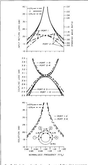
fig. 5. Variations in the impedance of the ring appears to have little effect on the operation of the hybrid ring.
