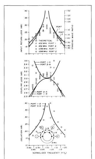
fig. 4. The experimental results using microstrip were also very close to the predicted values at 432 and 1296 MHz.
