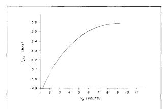
fig. 5. Example of  $f_{VCO}$  versus  $V_t$  showing nonlinear transfer function due to varactor diodes.
