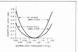
fig. 12. The insertion loss of two hybrids is lower for push-pull connections.
