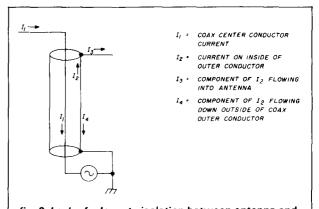
fig. 2. Lack of adequate isolation between antenna and feedline causes  ${\bf I_2}$  to divide into  ${\bf I_3} + {\bf I_4}.$
