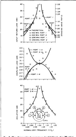
fig. 3. The theoretical response (solid line) of a 70-ohm hybrid ring is compared with experimental results using semi-rigid line.
