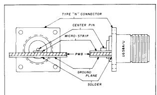
fig. 6. Inexpensive end launchers are formed by modifying common coaxial connectors.
