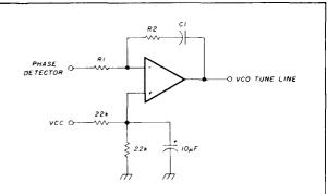
fig. 6. Op-Amp integrator used as active loop filter.
