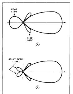
fig. 1. (A) Representation of field plot of a conventional Yagi showing side and rear lobes, and (B) Plot of "absorbing Yagi" showing reduction of unwanted lobes. The deep null to the rear of the array can be maximized by "fine tuning" the absorber element.
