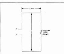
fig. 5. The terminated, traveling wave loop antenna provides good directivity, front-to-back ratio and bandwidth. Value of terminating resistor is not critical. RF energy reaching far end of antenna is dissipated in the resistor rather than being reflected back to the feedpoint. Wattage rating of resistor is equal to about one-half the power output of the transmitter.
