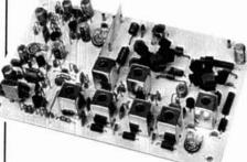
T51 VHF FM EXCITER for 10M, 6M, 2M, 220 MHz or adjacent bands. 2 Watts continuous, up to 2½ W intermittent. \$68/kit.
