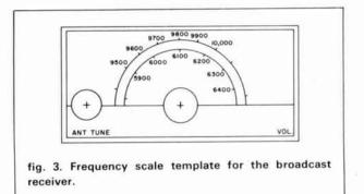
If you have a signal generator modulated by an audio tone it helps to align the 455 kHz IF and approximately calibrate the main frequency dials. If your signal generator is not accurate, then the dial should be checked against another receiver and recalibrated if necessary. (A frequency scale template is provided in fig. 3.)
