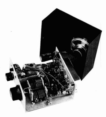
Total shielding of the VFO may not be possible in small packages like this one. This does not seem to degrade performance. The BFO should always be fully shielded. Note the bandpass filter mounted on the rear panel to save interior space.
