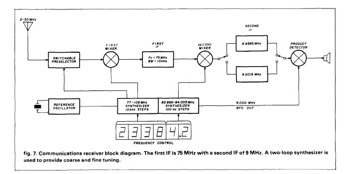
The filtered first IF range of 74.995 to 75.005 MHz is further mixed with the second local oscillator operating in 0.0001 MHz (100 Hz) steps over the 10 kHz range of 83.995 to 84.005 MHz, providing fine tuning for the receiver. If  $R_{MIN}$  and  $R_{MAX}$  are found for the second IF a new band of interest can be located on our chart, as shown in **fig. 8**.
