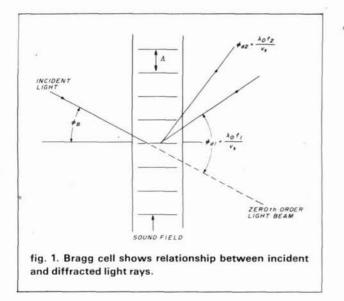
angles have been exaggerated for clarity. The Bragg cell diffracts light rays into angles controlled by spectrum of acoustic frequencies  $f_i$ , where i = 1, 2, etc. This acoustic spectrum is identical to the frequency spectrum of the electrical signal. Though Bragg cells exhibit limited bandwidth, this design is sufficiently wide to accommodate the entire FM band.
