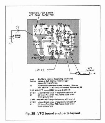
are installed on the circuit board. For that reason, all tuned circuits are wound, tacked together with solder, and checked for resonance with a grid-dip meter prior to actual board construction. A length of hook-up wire is used to link-couple the grid-dipper to the toroids. Each tuned circuit is then marked and set aside for later installation.
