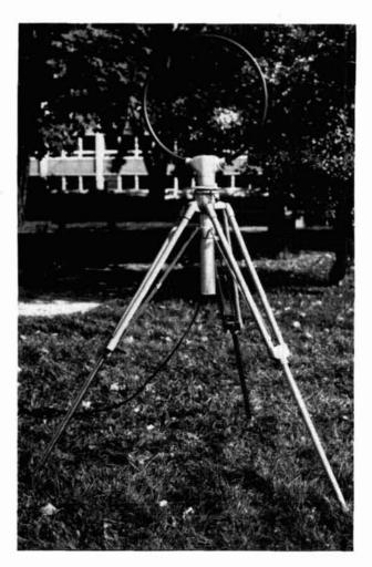
fig. 9. Loop antenna system recommended for EMI/RFI testing.
