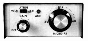
Simplicity of design is reflected in the front panel of this 75meter net monitor. In place of a signal-strength meter, an LED peak-indicator illuminates at full audio output to indicate AGC action.
