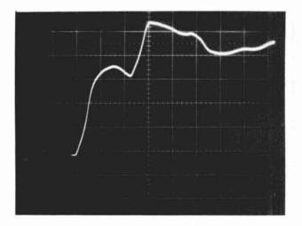
fig. 5. One hundred feet of RG-213 is now pulsed while an open exists at the far end (load end). The rapid rise in pulse height marks the location of the "fault" (open circuit). Horizontal deflection is 0.1 microseconds per centimeter.
