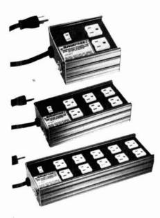
Designated "Surgefree," the new unit features all solid-state electronic circuitry. Compact in size, it can be plugged into any 120 VAC outlet to instantly sense and suppress destructive effects of high-voltage transient spikes and surges to sensitive electronic equipment. It is rated at 15 amps (1875 watt), 125 VAC, with a resettable circuit breaker that protects against accidental power overloads.
