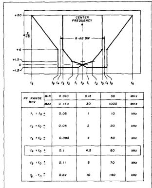
fig. 7. Required selectivity of the EMI/RFI receiver as a function of frequency range.
