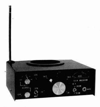
The completed receiver can be packaged to suit the builder. This 20-meter version features a signal-strength meter and a built-in voltage probe antenna system. The illuminated frequency pointer is an LED that has been filed to shape and polished. former. Builders desiring a thorough treatment of the design along with temperature compensation information should refer to current editions of the *ARRL Handbook*.
