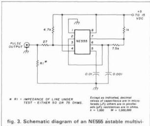
brator used in the time domain reflectometer.
