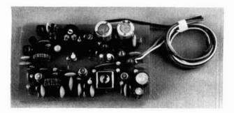
With the exception of the oscillators, all receiver circuitry is contained on the main board. Interconnecting leads for the speaker, volume control, and DC power are salvaged rainbow-wire.
