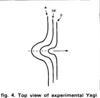
fig. 4. Top view of experimental Yagi using gain-optimized elements, each approximately 3/2-wavelengths long. VHF array of this design provided 11.5 dBi gain and a front-to-back ratio of about 26 dB.
