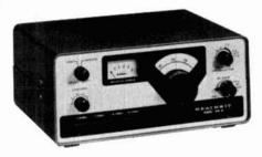
The HW-8 transceiver exhibits approximately 1500 Hz drift in transmit and receive frequency when the supply voltage varies over a range of 10 to 13.5 VDC. This results in CW chirp when using a poorly regulated supply, such as a weak, dry battery. Additionally, even with a well-regulated supply, the VFO dial calibration is in error on all but the 7 MHz band.
