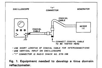
repeater group saying the repeater cannot be heard. They believe the malfunction is in either the transmission line or the antenna, but they're not certain which it might be. With a time domain reflectometer, you can tell whether the problem is in the antenna or the line — and if the trouble is in the line, approximately where it is.
