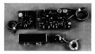
The main board, two oscillator boards, and a bandpass filter are the basic modules required to build one of these receivers. Interconnecting wires are salvaged rainbow-wire and mini-audio cable.
