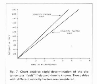
because of the extremely short times involved. In this case it would be desirable to add a 100-foot section of coax and then subtract 100 feet when you are calculating the distance.
