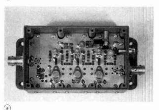
fig. 19. Finished amplifier with lid (A) and without (B).
