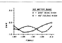
fig. 3. Computer-derived SWR curves for K4MT crossed-dipole antenna for 160-meter band. (Computer program by Paul Scholz, W6PYK.)
