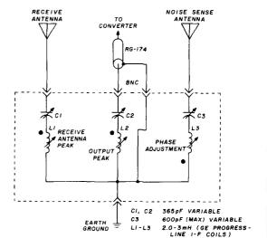
fig. 2. The 160-200 kHz RF phase cancelling circuit schematic. C1-C3 and L1-L3 can be increased or decreased in value to suit your frequency of interest. All coils are spaced 0.5 inch (12.7 mm) apart.
