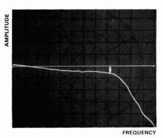
fig. 20. Swept frequency response of HF amplifier using GPD 460 series devices; the marker "birdie" is at 825 MHz (-3 dB point).
