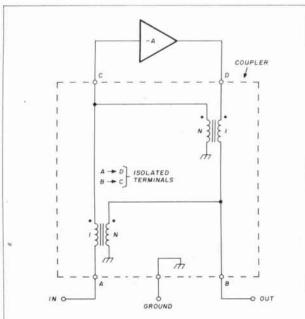
fig. 5. Transformer-type feedback networks provide lower noise figure and higher power to the load than the previous circuits.
