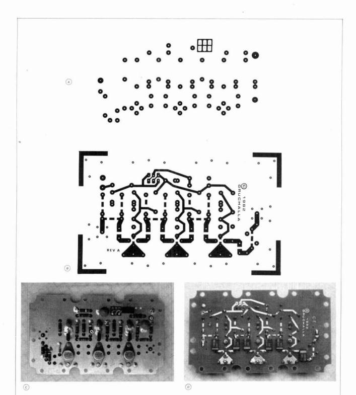
fig. 16. Double-sided PC board: (A) component side artwork, (B) ground plane side artwork, (C) completed assembly — component side view, and (D) completed assembly — ground plane side.
