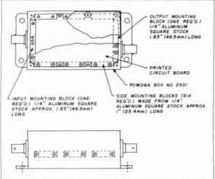
fig. 11A. Mounting shelves provide good ground plane coupling to box and good ground plane continuity between RF connectors and board.
