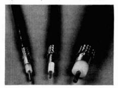
Belden 9915, an RG-218/U type solid polyethylene insulated coax, has an attenuation of 0.83 dB at 100 MHz, 1.6 dB at 300 MHz, 2.4 dB at 500 MHz, 2.7 dB at 700 MHz, 3.5 dB at 1 GHz, and 10 dB at 4 GHz. Nominal capacitance is 30.8 pF per foot. Overall diameter is 0.870 inch. Standard put-ups are 250 and 500 feet. Representative price is \$1,186.50 for 500 feet.
