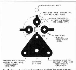
fig. 7. Ground pad configuration details by-pass capacitor, mounting and through hole locations.
