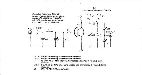
fig. 3. Frequency doubler: with a 95-110 MHz, 5-10 milliwatt input, a 190-220 MHz, 10-20 milliwatt output is produced.
