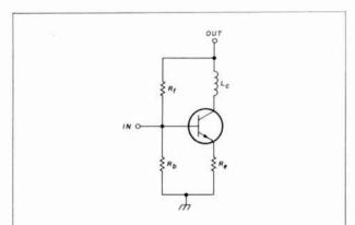
fig. 2. Simplified schematic of a 100 MHz bandwidth RF amplifier designed around the MWA module.
