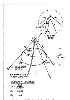
fig. 5. The K2GNC "Y-doublet" antenna for 80 meters. Antenna covers complete band with low SWR. It is supported from a single pole.
