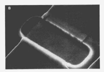
fig. 4. (A) shows static damage, magnified 7000 times, to a 3N157 MOSFET: (B) shows damage to an input pull-up resistor on a p-MOS character generator at 3000x magnification.
