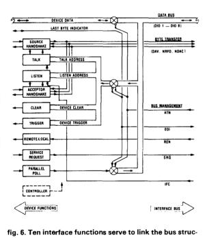
fig. 6. Ten interface functions serve to link the bus structure to the device functions.
