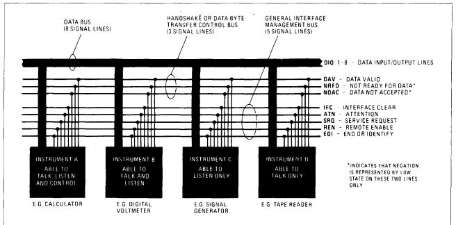
fig. 1. The HP-IB bus uses a 16-line cable to quickly link any instruments equipped with appropriate interface circuitry into a system. Data transfer is byte serial, bit-parallel at rates as high as 1 megabyte per second.
