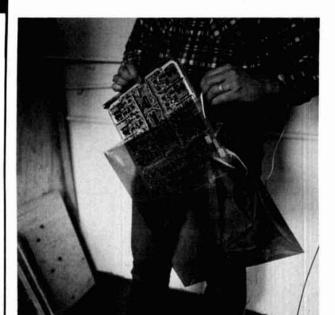
fig. 5. Three-layer bag protects circuit boards in shipping, storage, and handling. The outer surface is vapor coated with nickel to provide low surface resistivity to shield contents from external static fields. The middle layer provides strength, and the inner, heat-sealable layer prevents buildup of triboelectric (frictional) charge inside the bag.
