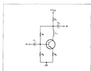
fig. 3. Simplified schematic of a wide bandwidth RF amplifier designed around the Avantek GPD series modules.
