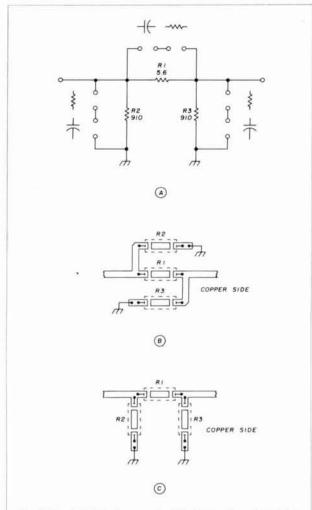
fig. 9. Typical interstage pads: (A) attenuator schematic; (B) input configuration; (C) interstage and output configuration.
