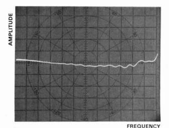
fig. 13. Response of 1 GHz (0-1200 MHz, 5 dB gain variation) amplifier using 10  $\mu$ F, 196D capacitors.
