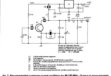
fig. 2. Recommended overtone crystal oscillator for 90-125 MHz. Output is approximately 10 milliwatts.
