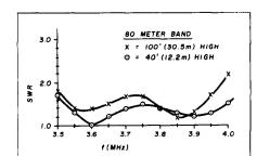
fig. 4. Computer-derived SWR curves for K4MT crossed-dipole antenna for 80-meter band. (Computer program by Paul Scholz, W6PYK.)
