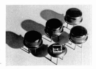
fig. 1. Hybrid modules are the basic building blocks around which the broadband amplifier is constructed.
