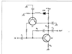
fig. 4. Schematic of a broadband amplifier that incorporates the Avantek UTO series of modules. More precise and stable operation is associated with slightly greater circuit complexity.
