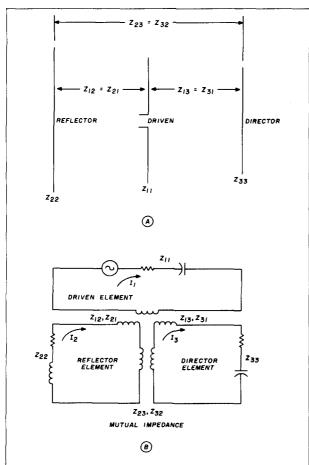
fig. 1A. Three-element Yagi antenna showing self- and mutual-impedance locations. fig. 1B. Network equivalent of three-element Yagi-Uda antenna.
