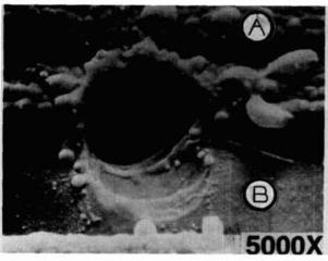
fig. 1. Enlarged, detailed views of a 6-micron (0.0002 inch) diameter hole created in aluminum metallization (A) and silicon dioxide substrate (B) by static electricity on an op amp integrated circuit.
