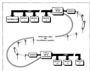
fig. 5. Point-to-point connection using twin twisted pair cable or full duplex modem link.
