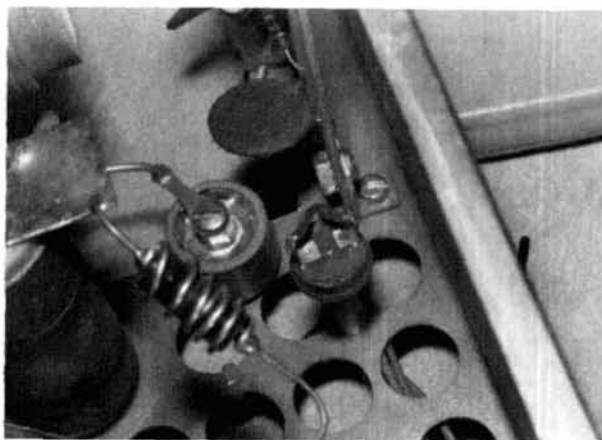
fig. 9. Original mounting of thermal sensor.
