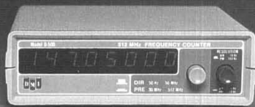
50 Hz to 512 MHz 1 PPM ACCURACY TCXO 5 1/4 X 5 X 1 1/2
