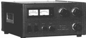
TL-922A 160-15 m 2 KW PEP/1 KW DC Input Linear Amplifier. Pair of EIMAC 3-500Z tubes and excellent IMD characteristics. Perfect safety protection with blower turn-off delay circuit.
