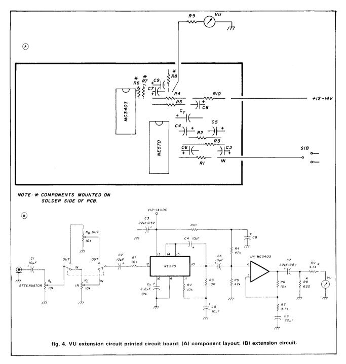
at the input. This can be checked with a VOM or digital voltmeter. After switching S1 to "IN," adjust  $R_{\rm C}$  for the same reading. You'll now notice that by dropping the input level 10 dB in the "OUT" position, you'll read -5 dB when you switch to the "IN" position.
