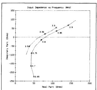
fig. 6. Computed input impedence versus frequency for phone and CW modes. These do not correlate well with measurement (see text).
