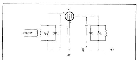
fig. 1. Simplified cathode driven circuit with  $R_D$  representing driver load and  $R_L$  amplifier load. Polarity of instantaneous RF voltages is indicated.
