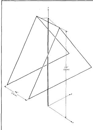
fig. 1. Delta loop array configuration. The perimeter of each equilateral loop is 264 feet. The horizontal side is 39 feet above ground.
