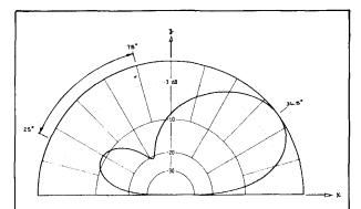
fig. 2. Elevation radiation pattern at 3.8 MHz. Peak gain is 8.69 dBi at 36.5 degrees. Front to back averaged over 25 to 75 degrees (see text) is 11.49 dB. The x and z axes are illustrated in fig. 1.
