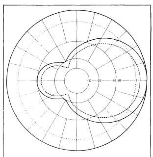
fig. 21. Azimuth pattern at 3.8 MHz and 36 degree elevation angle for salt water ground. The dashed pattern is for poor ground.
