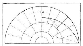
fig. 22. Reflected field intensity amplitude versus angle of incidence for horizontal (solid curve) and vertical (dashed curve) polarization with poor ground ( $\epsilon_{
