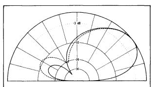
fig. 12. Elevation pattern at 3.8 MHz with spacing reduced to 32.4 feet. Peak gain is 8.70 dB at 36.5 degrees and average F/B is 16.07 dB. The dashed pattern is for 46-foot spacing.
