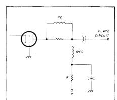
fig. 9. Resistor in series with B-plus protects tube and circuitry in case of flashover.
