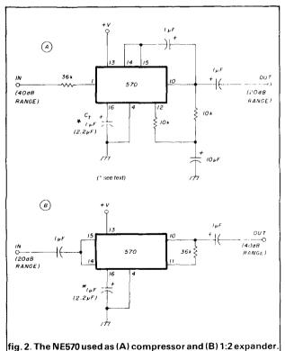
NE570 circuit compresses 40 dB-range into 20 dB
