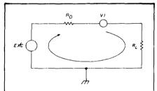
fig. 2. Exciter and amplifier are in series with respect to RF voltages. RF current flows through driver, as indicated by arrow.
