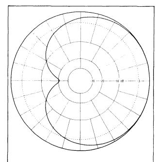
fig. 19. Azimuth pattern at 3.8 MHz for halfwave sloper plus 120 foot grounded tower.
