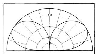
fig. 13. Elevation pattern at 3.8 MHz with both loops driven 180 degrees out-of-phase. Peak gain is 7.05 dB at 33 degrees.
