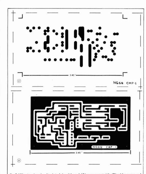
fig. 3. VU extension circuit printed circuit board: (A) component side; (B) solder or ground side. Note: if reader interest warrants, Project OSCAR will prepare printed circuit boards. Address inquiries to author (enclose SASE).
