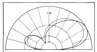
fig. 10. Elevation pattern at 3.8 MHz with the array raised to 145 feet. Peak gain is 9.97 dBi at 30.5 degrees and average F/B is 11.10 dB. The dashed pattern is for boom at 115
