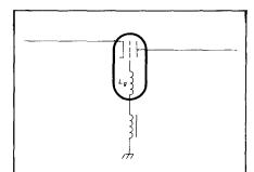
fig. 6. Below self-neutralizing frequency of tube, series inductor shifts point of self neutralization to operating frequency.
