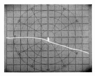
fig. 9. Amplifier frequency response.
