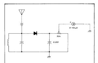
fig. 1. The typical field-strength meter circuit will work for HF medium power applications, but is useless for 1750-meter QRP testing.
