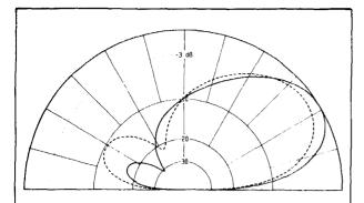
fig. 14. Elevation pattern at 3.8 MHz for square loops with the same perimeter as the triangular loops. Peak gain is 9.71 dBi at 31.5 degrees and average F/B is 16.52 dB. The dashed pattern is for triangular loops.
