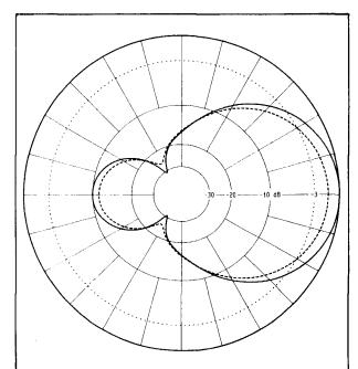
fig. 11. Azimuth pattern at 3.8 MHz with the array raised to 145 feet. The dashed pattern is for boom at 115 feet.
