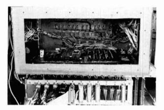
fig. 3. Inside of computer controller. Much of the visible wiring is for the diagnostic front panel.
