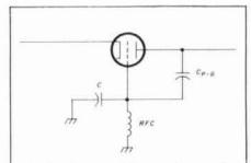
fig. 10. Plate-to-grid capacitance plus capacitor C forms voltage divider to impress negative feedback voltage with respect to cathode. RF choke completes grid DC return.
