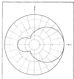
fig. 3. Azimuth radiation pattern at 3.8 MHz for 36 degree elevation angle. The x and y axes are illustrated in fig. 1.
