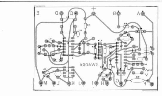
fig. 2A. Component layout on the WA2PZO printed circuit board (foil side down).
