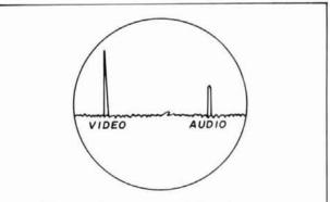
fig. 6. 8-MHz horizontal sweep width, with channel 2 video signal at left and channel 2 audio at right.
