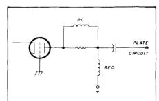
fig. 8. Proper position of parasitic choke is in the plate lead of cathode driven amplifier.
