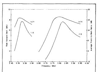
fig. 4. Two element delta loop array performance versus frequency for phone and CW modes. The phone-mode design frequency is 3.8 MHz. The CW-mode is created by series-loading each loop with a 12  $\mu$ H inductor.
