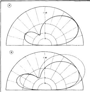
fig. 8. Elevation patterns at 3.8 MHz for alternate feedpoints. Peak gains are 8.80 dBi and 5.48 dBi for (A) bottom and (B) corner feed, respectively. Corresponding average F/B ratios are 11.53 dB and 7.83 dB. The dashed pattern on these charts is for top feed.
