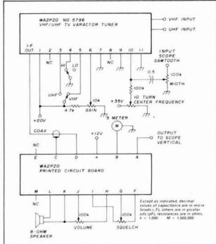
fig. 3. Schematic showing interconnections between tuner, printed circuit board, and oscilloscope. Note: +35, + 20, and + 12 VDc sources are regulated supplies.
