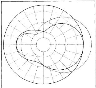
fig. 9. Azimuth pattern at 3.8 MHz with corner feed. The pattern is skewed towards the side of the boom containing the feedpoint. The dashed pattern is for top feed.
