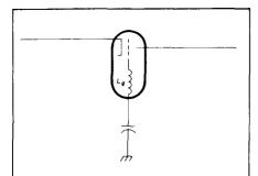
fig. 7. Above self-neutralizing frequency of tube, series capacitor shifts point of self neutralization to operating frequency.
