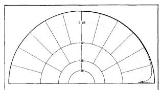
fig. 23. Reflected field intensity amplitude versus angle of incidence for horizontal (solid curve) and vertical (dashed curve) polarization with good ground ( $\epsilon_0 = 80$  and  $\delta = 5$ S/m). The solid curve nearly coincides with the 0 dB arc at all angles.
