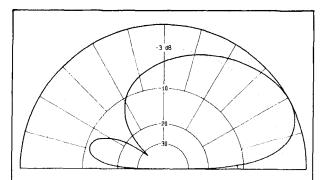
fig. 18. Elevation pattern at 3.8 MHz for a halfwave sloper plus 120 foot grounded tower. Peak gain is 1.56 dBi at 28.5 degrees and average F/B is 11.12 dB. Peak gain without the tower is 0.81 dBi at 31.5 degrees.
