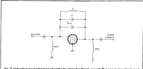
$fig.\,3.\,Inductive\,neutralization\,of\,cathode-plate\,feedback\,circuit.\,Resonant\,circuit\,is\,tuned$ to operating frequency.
