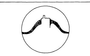
fig. 7. Sweep width reduced to about 2 or 3 MHz with center frequency set to channel 2's video carrier.
