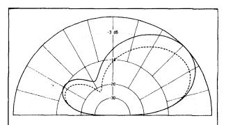
fig. 20. Elevation pattern at 3.8 MHz for sea water ground conditions. Peak gain is 10.47 dBi at 42.0 degrees and average F/B is 11.25 dB. The dashed pattern is for poor ground.
