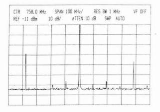
fig. 8. Spectal output plot of the multiplier chain. The desired signal is at +9 dBm. The highest undesired products are at 379 and 1137 MHz, approximately 30 dB down the 758 MHz signal.
