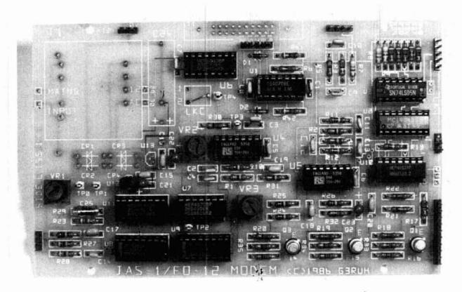
Photo D. Completed circuit board. AC power supply components have been omitted; link LKC is shown for a TAPR TNC-2.
