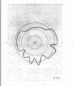
fig. 13. MUF propagation prediction from Los Angeles, California at 1600 UTC at a solar flux of 70. 1 UTC
