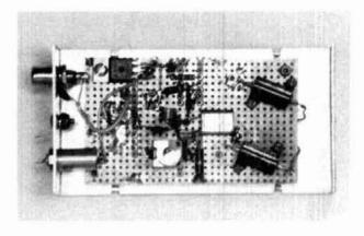
fig. 7. Photograph of the prototype oscillator in its shielded housing.
