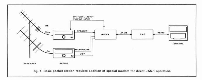
connect the internal modem and substitute an external modulator/PSK demodulator such as the one described in this article. This isn't particularly difficult. Just build the circuit, link it to your TNC with only four or five wires, adjust the audio connections, and the global mailbox is yours to enjoy!
