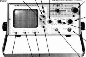
POWER switch has 3 positions for Battery Operation, Standby, and AC Line Operation
