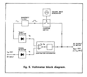
diodes, their temperature and I-V curve variations are minimized. Of course, since the mimic detector measures only a fixed low frequency signal, no frequency response compensation for the input detector is provided. Therefore, it's best to choose the diode that has the flattest possible response.
