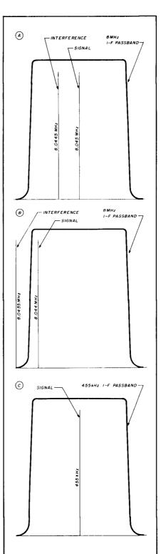
fig. 2. I-F shift, or i-f tuning, can move an interfering signal out of the i-f passband, then place the wanted signal back in the low-freqency i-f window for clear reception. This example uses approximately 8 MHz for a passband filter, then converts down to a conventional 455kHz i-f for further amplification and detection. and might end up as a tone that's not easy to hear (on CW) or as duck-talk (on SSB).
