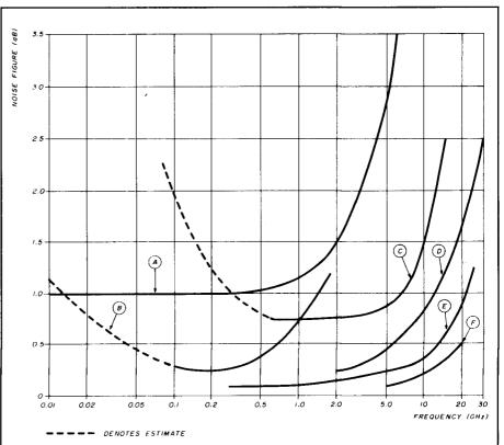
fig. 2. Typical 1987 state-of-the-art noise figures of bipolar transistors, GaAsFETs, and HEMTs: (A) uncooled bipolar transistor; (B) low-frequency GaAsFET at room temperature; (C) high-frequency GaAsFET at room temperature; (D) HEMT at room temperature; (E) GaAsFET cooled to 12 degrees Kelvin; (F) HEMT cooled to 12 degrees Kelvin. means that the noise figure increases not only as you increase frequency, but also as frequency is decreased! This effect is shown in **fig. 2**.
