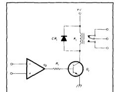
fig. 3. Addition of switching transistor allows higher current loads to be controlled.
