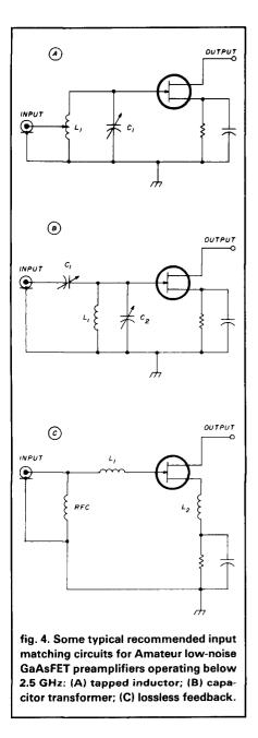
carefully chosen. This can be very tedious and time-consuming, especially if you want to achieve minimum noise figure. Therefore, the input impedance-matching circuit shown in **fig. 4B** is recommended for 500 MHz and below.<sup>1</sup>
