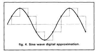
processor or memory circuit. A sine wave or any other waveform can be approximated by discrete steps as shown in **fig. 4**. For LO applications, sine wave approximation is preferred because sine waves have the lowest harmonic content. (A perfect sine wave will have no harmonic content.)
