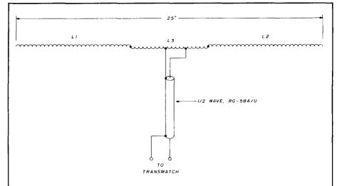
fig. 3. The mini-antenna of WOSVM. Adjust coax tap for best SWR at resonance.
