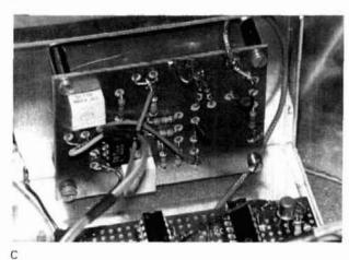
fig. 8. Internal views of the rf voltmeter: (A) internal power provided by two 9-volt batteries; (B) "clean" construction enhanced by use of Veroboard; (C) "rf" section of voltmeter.
