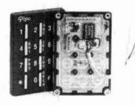
The P-7, a 12-key touchtone encoder, comes in vertical (P-7V) or horizontal (P-7H) formats measuring 2.16 inches by 1.5 inches by 0.20 inches. The P-8, a 16-key touchtone encoder, is available in a vertical (P-8V) format only; it measures 2.16 inches by 1.9 inches by 0.20 inches. Both are available in black or dark brown.
