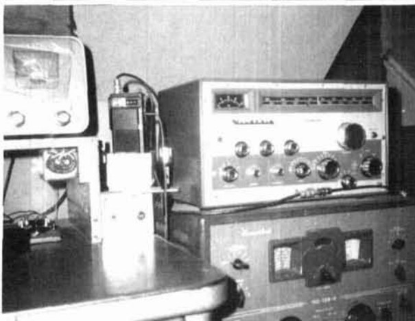
The Heathkit Seneca as a 2-meter FM amplifier for a handheld transceiver.
