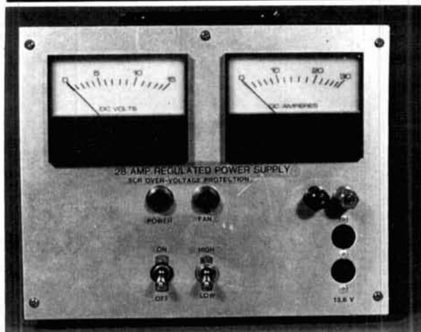
28-A power supply. Note switch for 2-speed fan.
