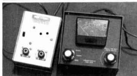
Heath combined power/VSWR meter with wired remote sensor.
